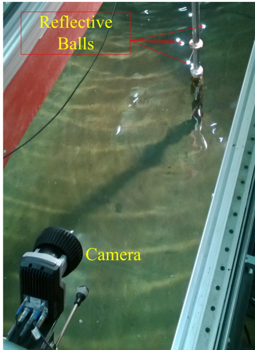
Figure 4.9: The Qualisys optical motion capture system; one of the cameras and the reflective balls can be seen in the photo.
