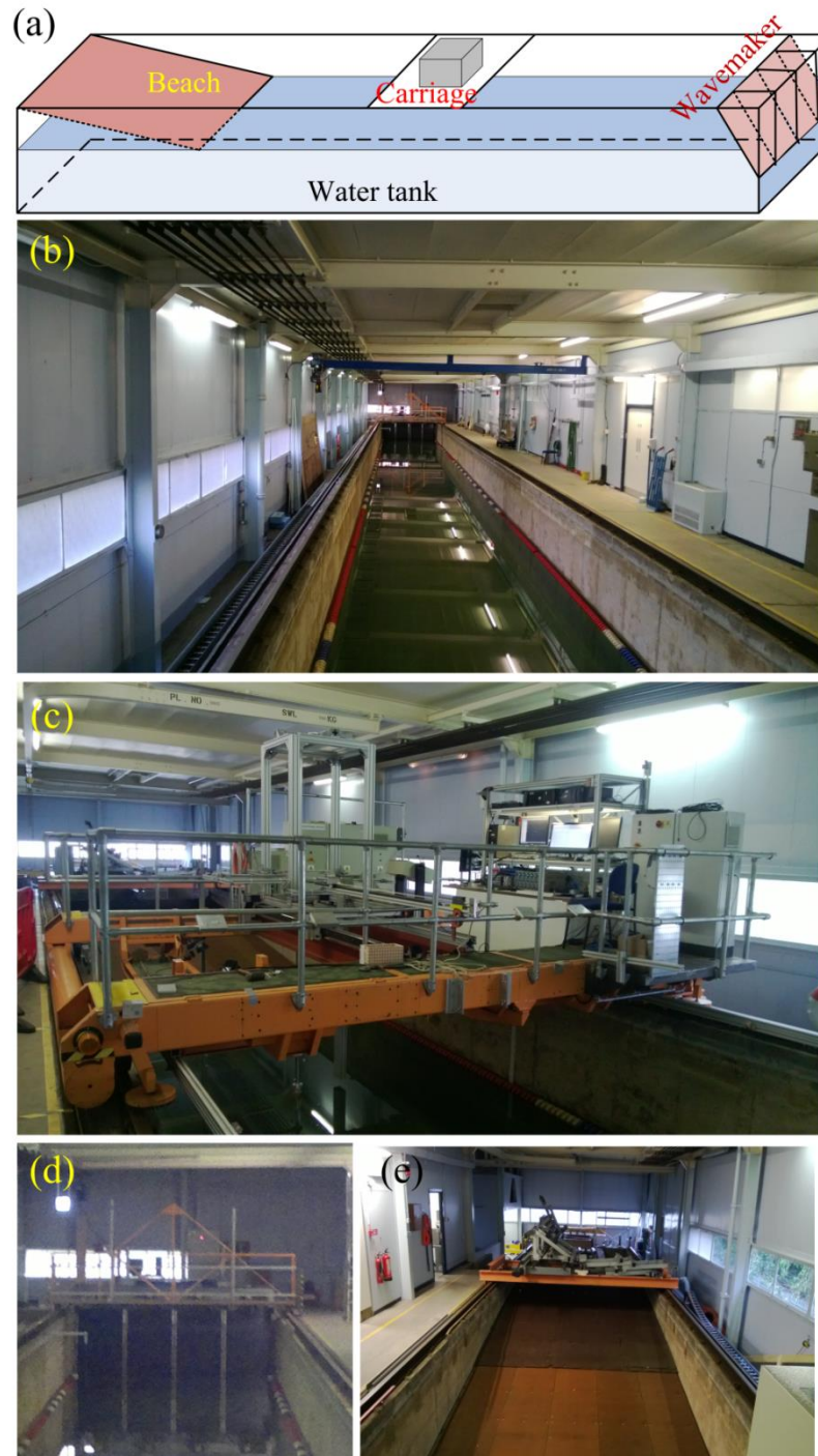
Figure 4.1: Towing tank of the Kelvin Hydrodynamic Laboratory (a) schematic representation, (b) water tank, (c) carriage, (d) wavemaker and (e) beach of the towing tank.
