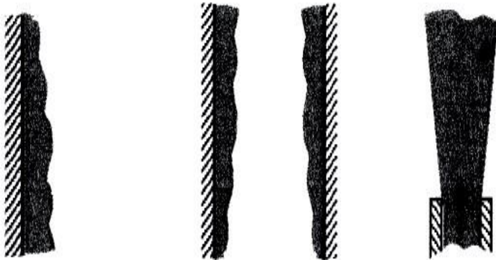
Figure3-3: Separated two-phase flow: film flow, annular flow and jet flow [62]
