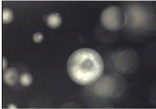
Figure. 5.22 Polarised photomicrograph of material formed from sprayed ibuprofen-GMS mixture, comprising of 53-90 \mu m ibuprofen, 2hrs post manufacture at x10 magnification.
