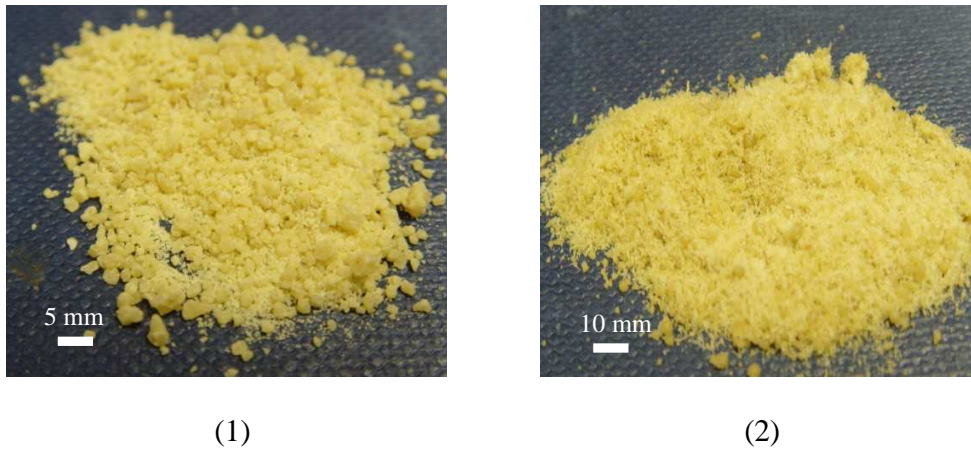
Figure 7.7 Digital photographs of (1) Minocycline HCl milled granules and (2) Minocycline HCl sprayed granules.
