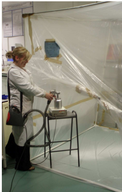
Figure 2.1 Agitated hot-melt spray system and spraying chamber
