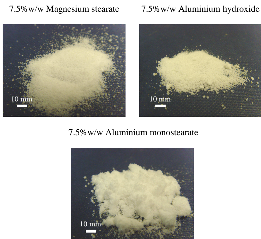
Figure 6.4 Macroscopic appearance of ibuprofen-GMS sprayed granules produced at 80°C with varying multivalent organic salts at 7.5% w/w.
