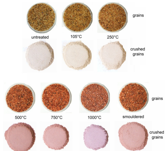
Figure 1. Silica Sand grains and crushes grains after heat treatment
