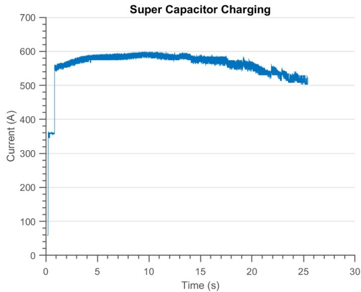
Fig. 6.27 Capacitor charging current (Approx)
