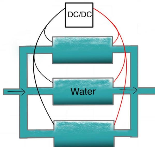
*Fig. 1.5 Water desalination cells connected in parallel, electrically connected in parallel*
