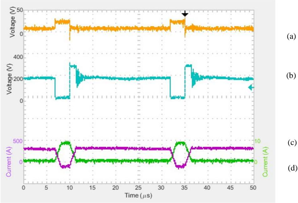
Fig. 6.12 Switch Q2 and Q3 and primary and secondary currents. (a) Q1 Switch Voltage (Vds), (b) Q2 Switch Voltage (Vds), (c) Secondary (L2) inductor current, (d) Primary (L1) inductor current
