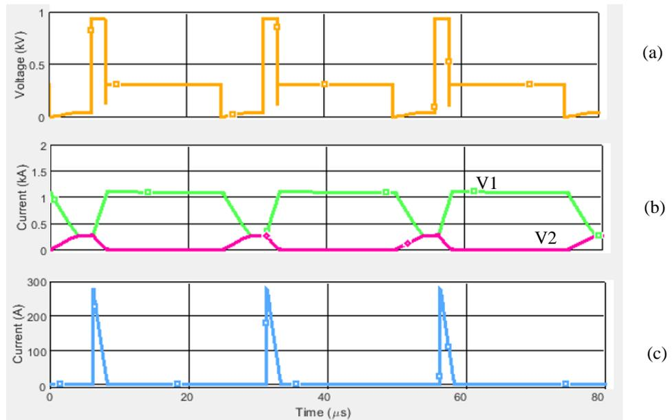
Fig. 4.12 Buck-boost clamp snubber 3:1 turns ratio with 32% snubber switch duty cycle. (a)  $Q1$  Switch Voltage ( $V_{ds}$ ), (b)(V1) Secondary ( $L2$ ) inductor current, (b)(V2) Primary ( $L1$ ) inductor current, (c) Snubber diode current ( $D1$ )
