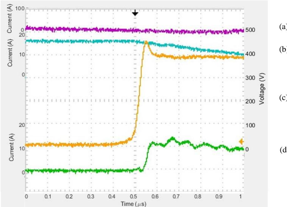
Fig. 4.17. Detailed view of circuit waveforms at clamp voltage of 385V. (a) Secondary (L2) inductor current, (b) Primary (L1) inductor current, (c) Q1 Switch Voltage (Vds), (d) Snubber diode current (D1)
