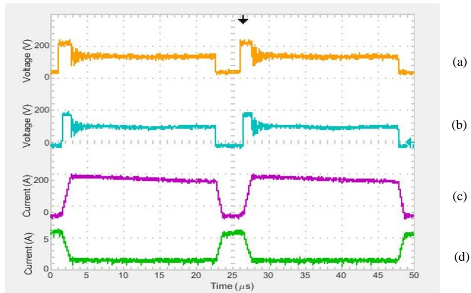
Fig. 6.19 Two full switching waveforms at minimum capacitor voltage of 0.8V. (a)  $Q1$  Switch Voltage ( $V_{ds}$ ), (b)  $Q2$  Switch Voltage ( $V_{ds}$ ), (c) Secondary ( $L2$ ) inductor current, (d) Primary ( $L1$ ) inductor current
