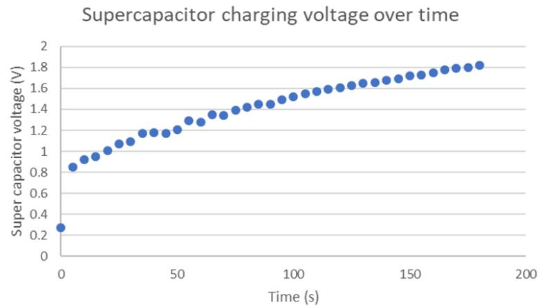
*Fig. 6.29 capacitor voltage (charging) 350A*
