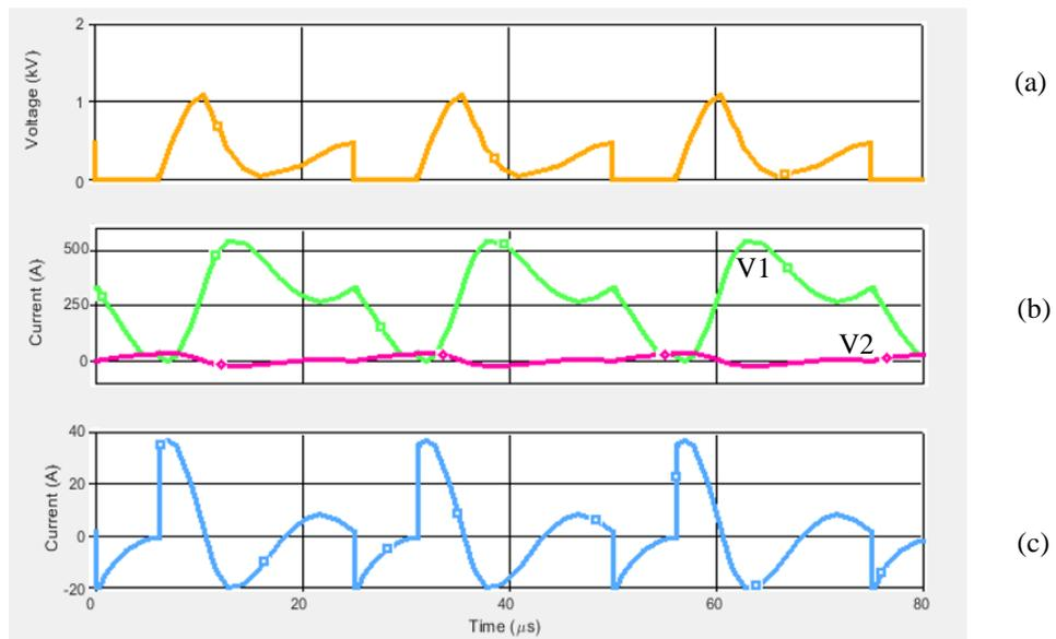
Fig. 2.27 RCD Snubber 10:1. (a) Q1 Switch Voltage ( $V_{ds}$ ), (b)(V1) Secondary ( $L_2$ ) inductor current, (b)(V2) Primary ( $L_1$ ) inductor current, (c) Snubber capacitor ( $C_1$ ) current
