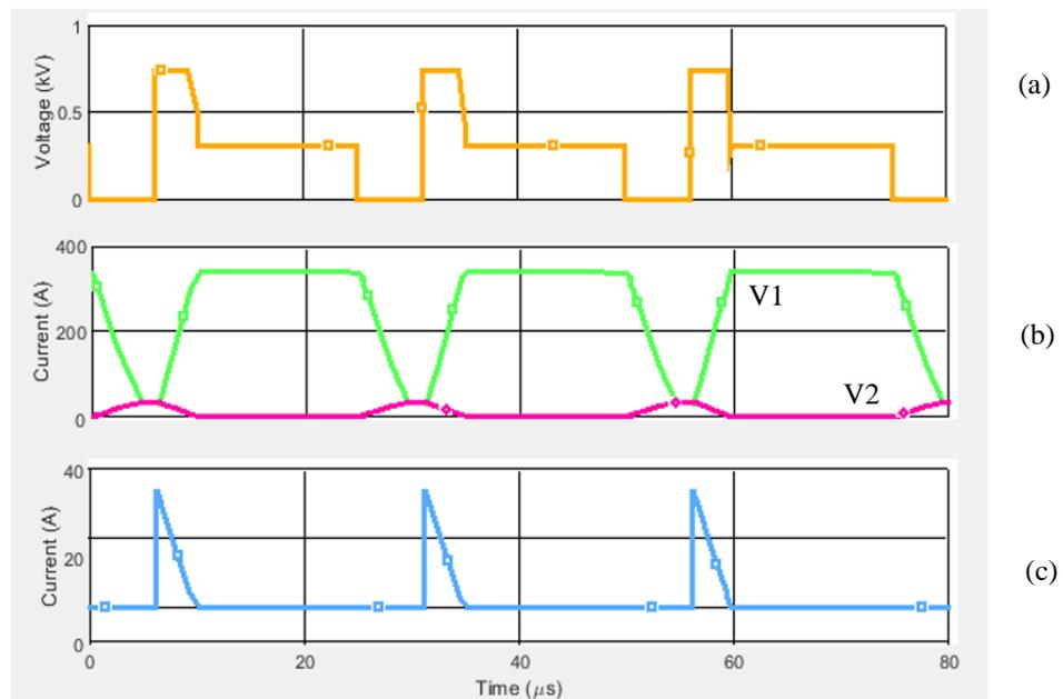
Fig. 4.13 Buck-boost clamp snubber 10:1 turns ratio with 40% snubber switch duty cycle (a)  $Q1$  Switch Voltage ( $V_{ds}$ ), (b)(V1) Secondary ( $L2$ ) inductor current, (b)(V2) Primary ( $L1$ ) inductor current, (c) Snubber diode current ( $D1$ )
