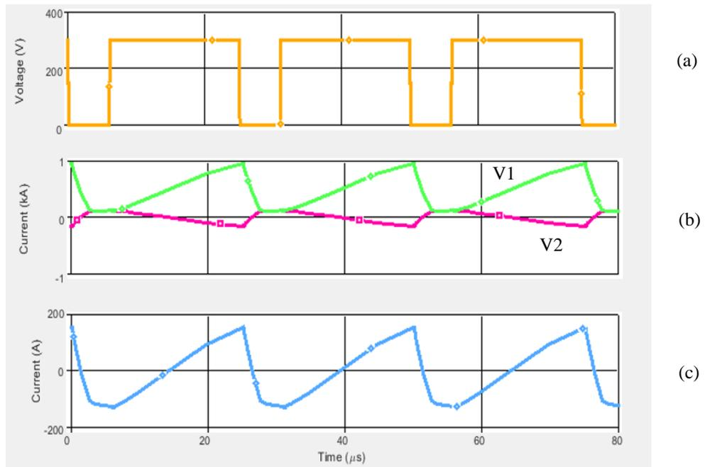
Fig. 2.15 Ultra high stepdown converter simulated with 3:1 turns ratio. (a)  $Q1$  Switch Voltage ( $V_{ds}$ ), (b)(V1) Secondary ( $L2$ ) inductor current, (b)(V2) Primary ( $L1$ ) inductor current, (c) Snubber capacitor ( $C_s$ ) current
