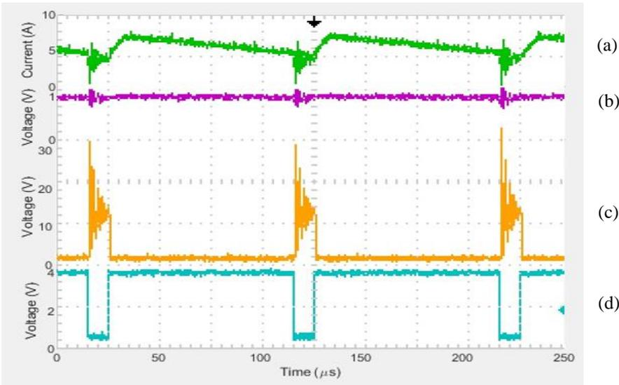
Fig. 4.6 Discontinuous operation with reverse current flow. (a) Secondary (L2) inductor current, (b) Load Voltage R1, (c) Q2 Switch voltage (Vds), (d) Q1 Gate Signal (Vgs)
