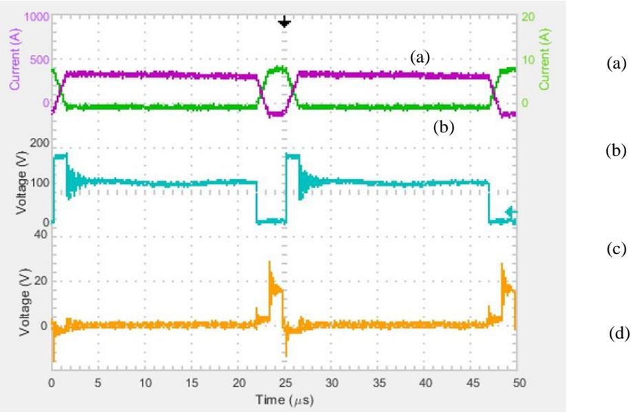
Fig. 6.10 Maximum operation with secondary switch voltage at 29V. (a) Secondary (L2) inductor current, (b) Primary (L1) inductor current, (c) Q1 Switch Voltage (Vds), (d) Q3 Switch Voltage (Vds)
