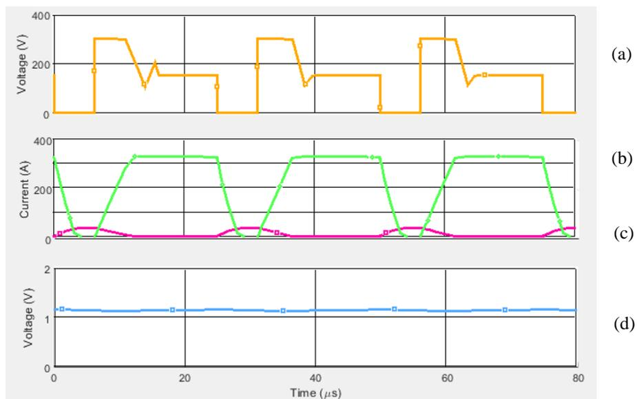
Fig. 6.2 Affirmation simulations of the asymmetrical half-bridge flyback converter. (a) Q1 Switch Voltage ( $V_{ds}$ ), (b) Secondary ( $L_2$ ) inductor current, (c) Primary ( $L_1$ ) inductor current, (d) Output Voltage ( $V_{out}$ )
