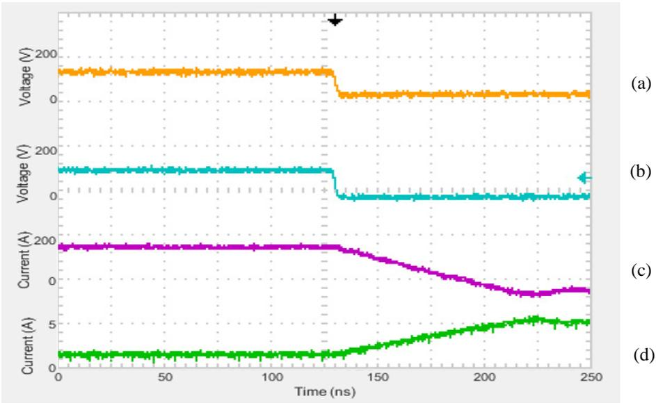
Fig. 6.17 Primary switch turn on transition 0.8V. (a) Q1 Switch Voltage (Vds), (b) Q2 Switch Voltage (Vds), (c) Secondary (L2) inductor current, (d) Primary (L1) inductor current
