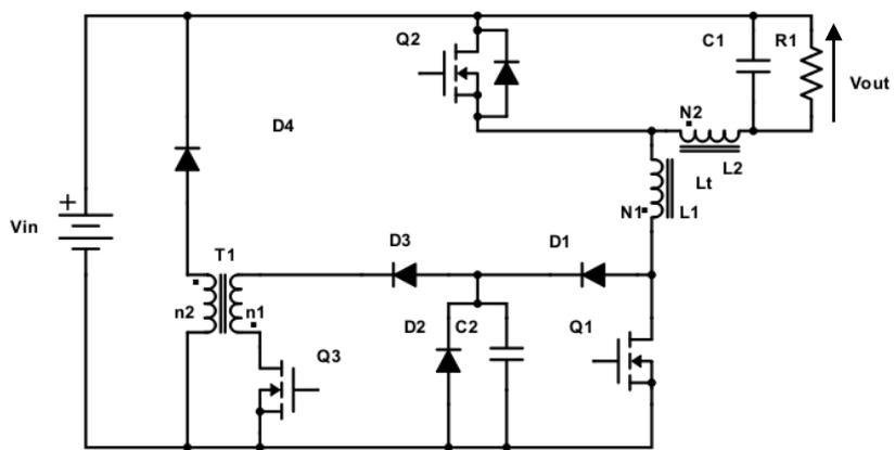
Fig. 4.8. Snubber circuit modified to a flyback configuration (note change in dot convention of  $T_1$ ).
