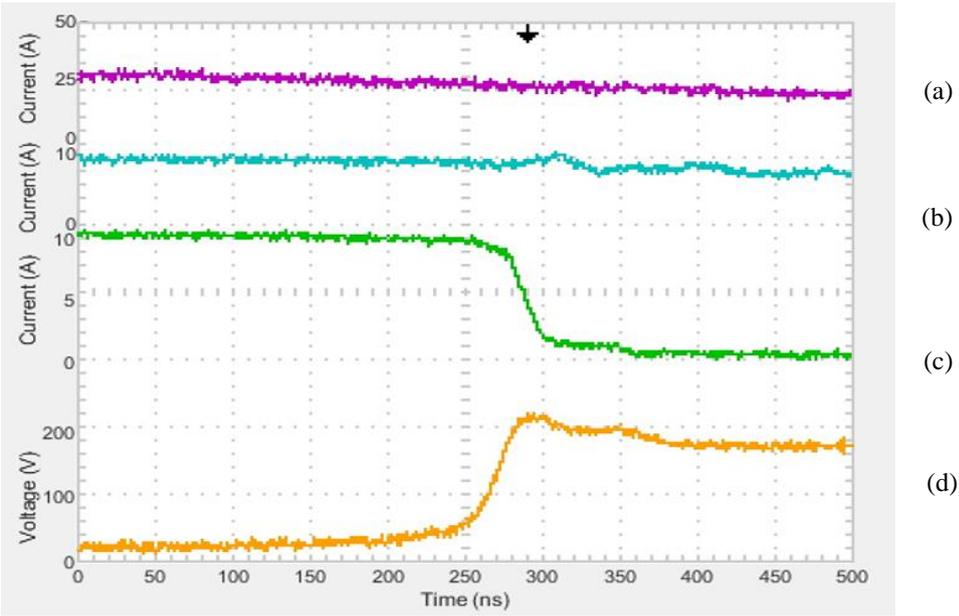
Fig. 5.4 Detailed switching waveforms of the asymmetrical half-bridge coupled-inductor buck converter. (a) Secondary (L2) inductor current, (b) Primary (L1) inductor current, (c) Q1 source current, (d) Q1 Switch Voltage (Vds)
