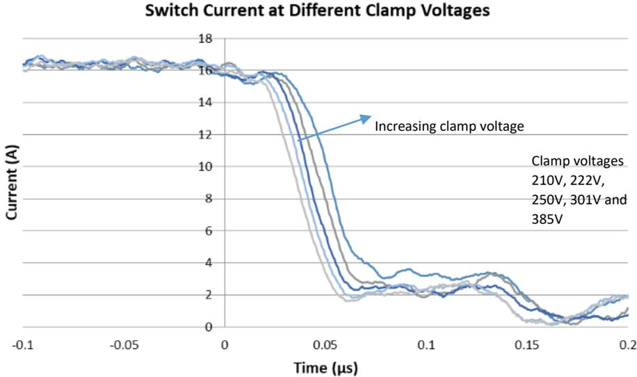
Fig. 4.18 Q1 turn off transition currents at different clamp voltages.
