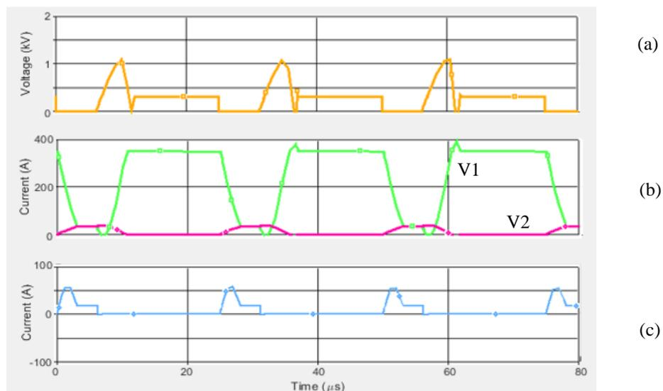
Fig. 4.3 Simulation of regenerative snubber, voltage across Q1 and primary and secondary currents showing conventional operation. (a) Q1 Switch Voltage ( $V_{ds}$ ), (b)(V1) Secondary (L2) inductor current, (b)(V2) Primary (L1) inductor current, (c) T1 primary current ( $n1$ )
