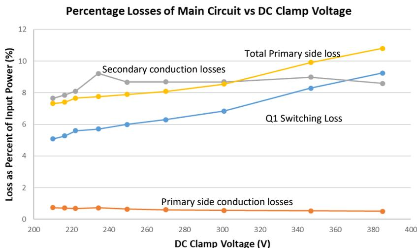
Fig. 4.21 Summary of switching and conduction losses.
