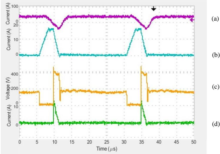
Fig. 4.15 Circuit waveforms at clamp voltage of 385V. (a) Secondary (L2) inductor current, (b) Primary (L1) inductor current, (c) Q1 Switch Voltage (Vds), (d) Snubber diode current (D1)
