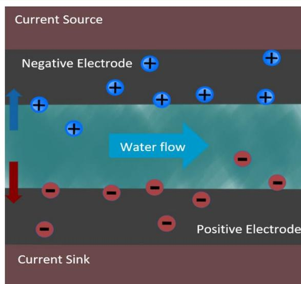
*Fig. 1.2 Capacitive deionisation electrode cross section*
