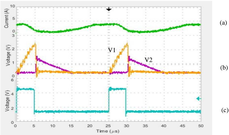
Fig. 4.9 Flyback snubber with  $N_1:N_2=2:1$  turns ratio. (a) Secondary (L2) inductor current, (b)(V1) T1 Primary current, (b)(V2) T1 Secondary current, (c) Q1 Gate Signal ( $V_{gs}$ )
