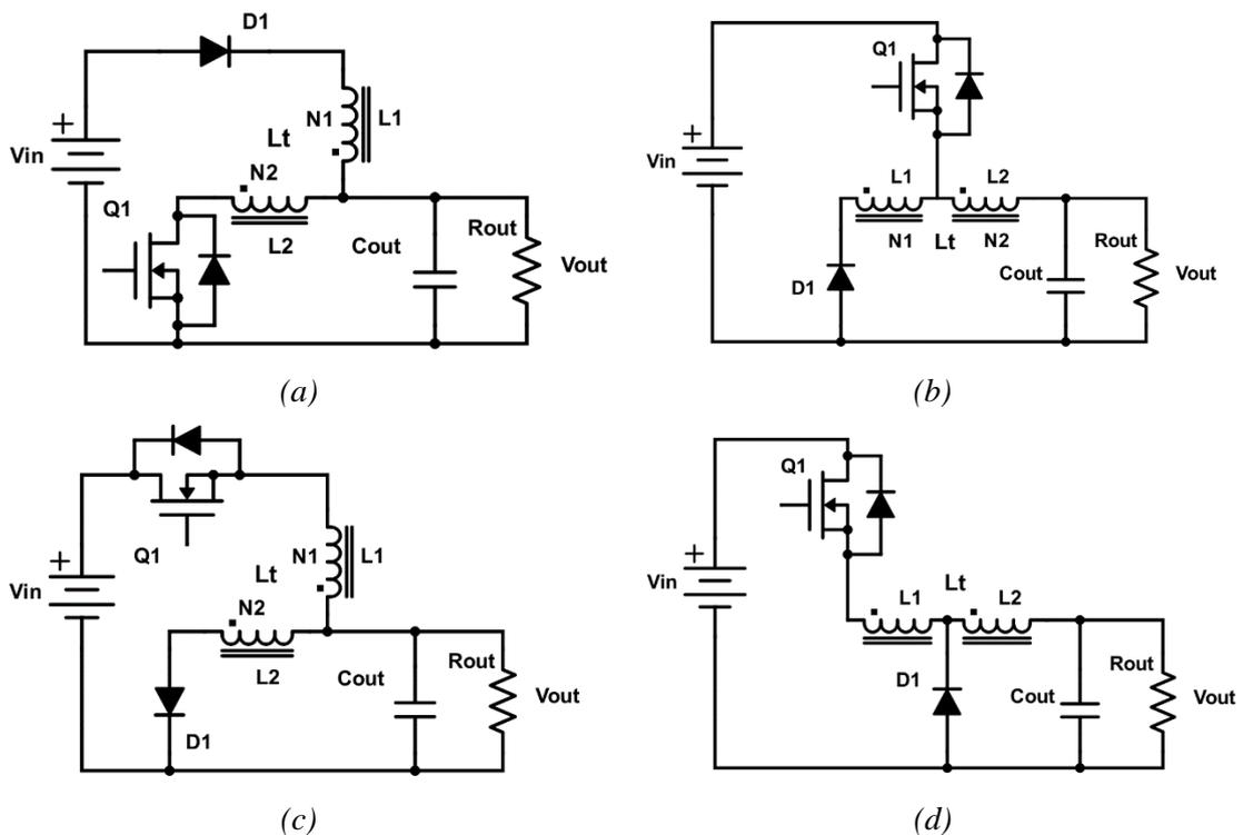
Fig. 2.7 four buck function circuits: (a) T1b+ output tap, (b) S1+/- switch tap, (c) T1+ output tap, (d) S5+/- diode tap [41]
