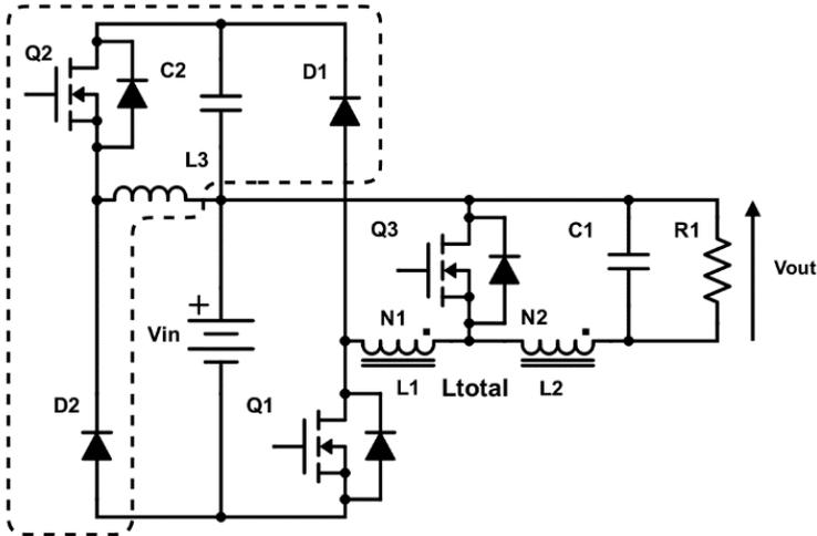
Fig. 4.11. Voltage clamp circuit for single-ended coupled-inductor circuit. The dotted line shows the added buck-boost converter with capacitor C2 referenced to  $V_{in}$ .
