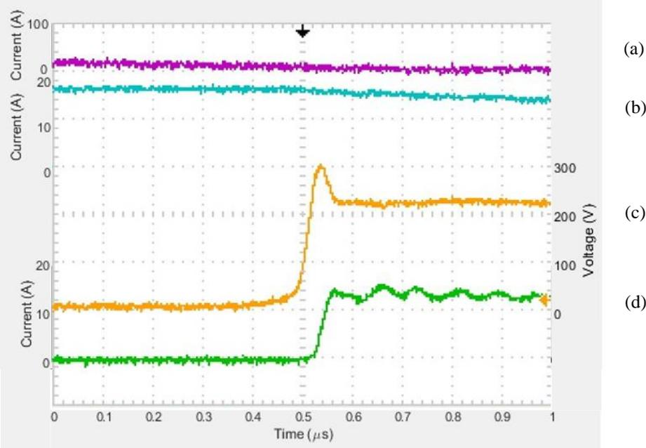
Fig. 4.16. Detailed view of circuit waveforms at clamp voltage of 250V. (a) Secondary (L2) inductor current, (b) Primary (L1) inductor current, (c) Q1 Switch Voltage (Vds), (d) Snubber diode current (D1)
