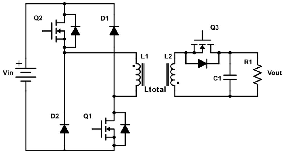
Fig. 6.1 Asymmetrical half-bridge flyback converter
