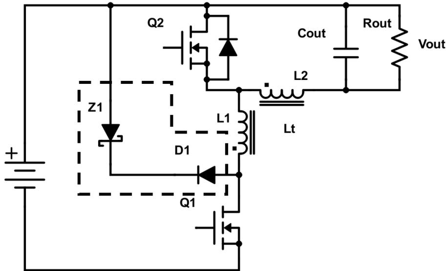
Fig. 2.34 Zener diode snubber circuit
