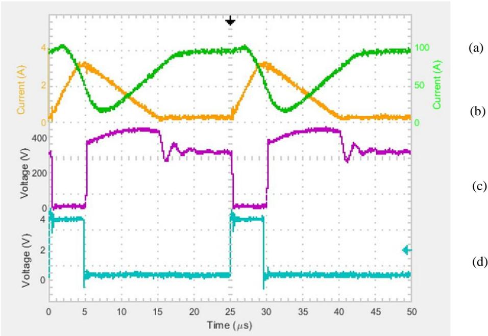
Fig. 2.32 Passive RC snubber experimental testing (hardware details described in Section 4.5, Table 3.4) (a) Secondary (L2) inductor current, (b) Primary (L1) inductor current, (c) Q1 Switch Voltage (Vds), (d) Q1 Gate Signal (Vgs)
