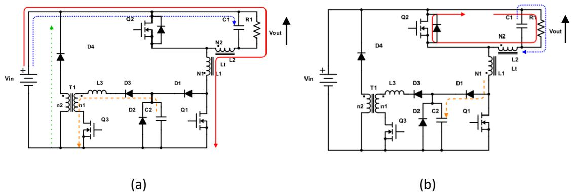
Fig. 4.2 (a) Mode 1 - energising coupled inductor  $L_t$ , (b) Q1 turned off discharging  $L_t$ .
