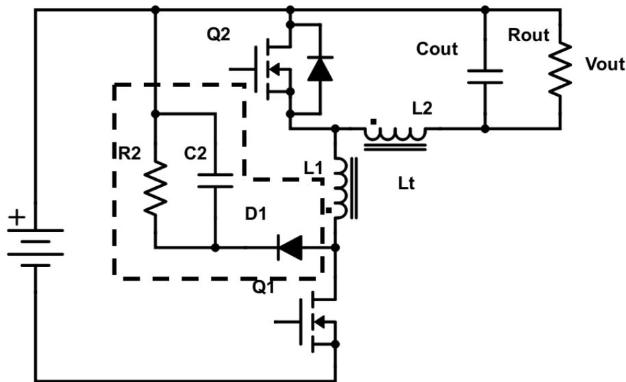
Fig. 2.29 Passive snubber implementation. The S5+/- circuit, but with the topology rearranged so the main switch is referenced to 0V.
