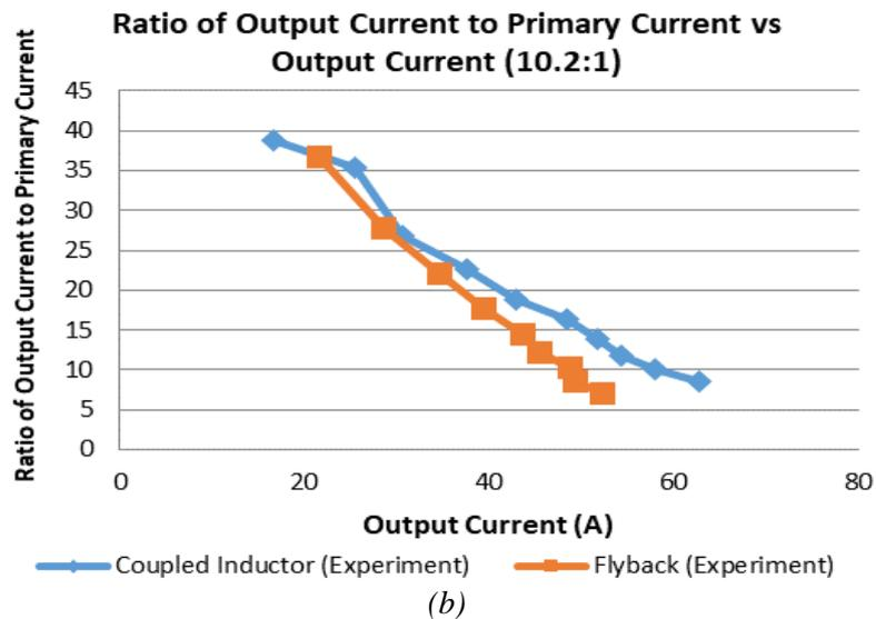
Fig. 3.10 Ratio of output current to primary current plotted against output current by varying duty cycle, for a turns ratio of: (a) 2.65:1 and (b) 10.2:1.
