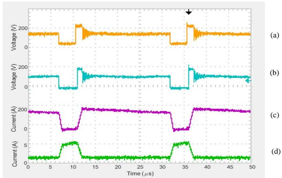
Fig. 6.22 Two full charging waveforms for 1.3V super-capacitors. (a)  $Q1$  Switch Voltage ( $V_{ds}$ ), (b)  $Q2$  Switch Voltage ( $V_{ds}$ ), (c) Secondary ( $L2$ ) inductor current, (d) Primary ( $L1$ ) inductor current
