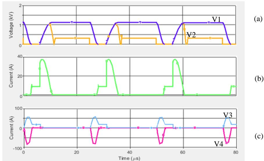
Fig. 4.4 Regenerative snubber operation (a)(V1) C2 Capacitor Voltage, (a)(V2) Q1 Switch Voltage ( $V_{ds}$ ), (b) Snubber current (D1), (c)(V3) T1 Primary current, (c)(V4) T1 Secondary current
