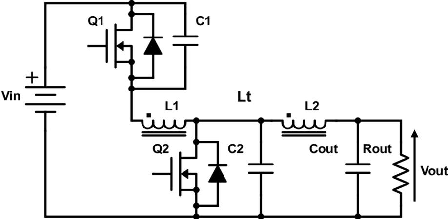
Fig. 2.17 High Voltage coupled-inductor buck converter S5+/- with additional shunt capacitors [51]
