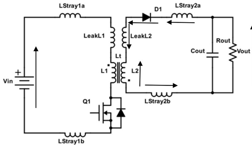
Fig. 2.10 Non ideal voltages seen by flyback converter
