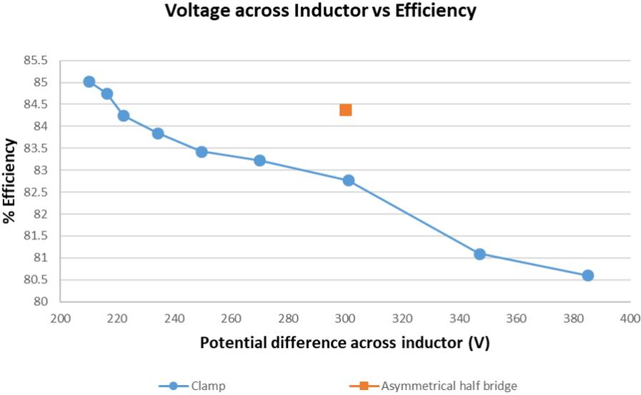
Fig. 5.5 Asymmetrical half-bridge and single-ended voltage clamped, coupled-inductor converter efficiencies versus inductor potential difference.
