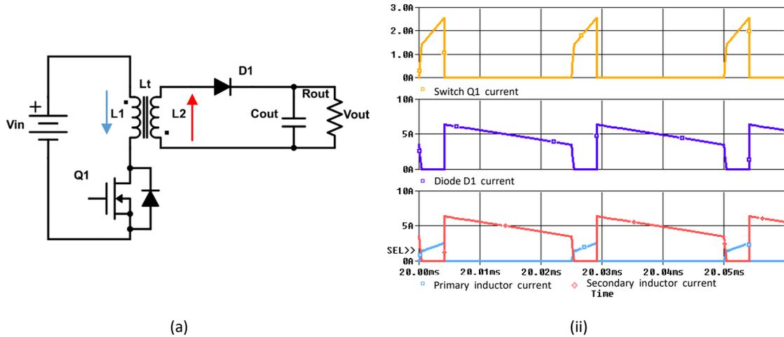
Fig. 2.3 Single switch flyback converter: (i) schematic and (ii) simulation currents for switch  $Q1$ , diode  $D1$  and the primary and secondary of  $L_t$ .
