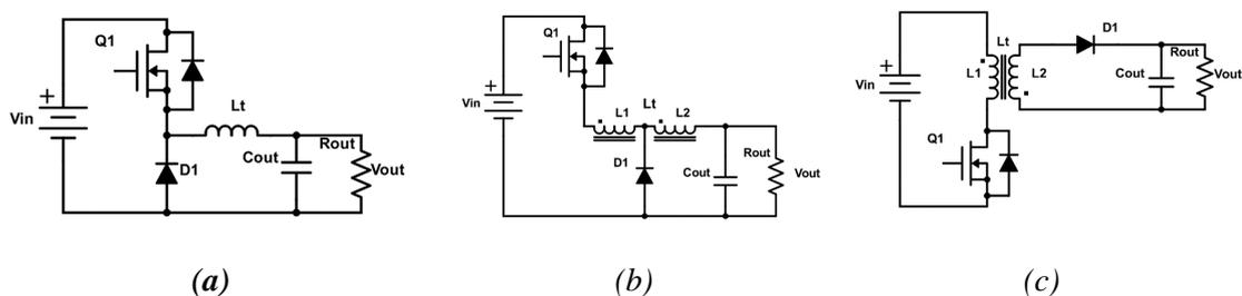
Fig. 3.1 Circuit schematics of (a) Buck converter, (b) Coupled-inductor buck converter, (c) Flyback converter
