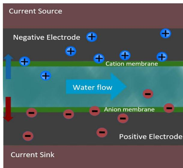
*Fig. 1.3 Membrane Capacitive Deionisation cross section*
