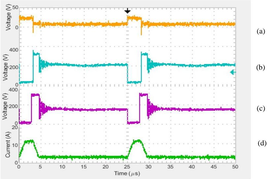
Fig. 6.11 Three switch voltages and Primary current. (a) Q3 Switch Voltage (Vds), (b) Q1 Switch Voltage (Vds), (c) Q2 Switch Voltage (Vds), (d) Primary (L1) inductor current
