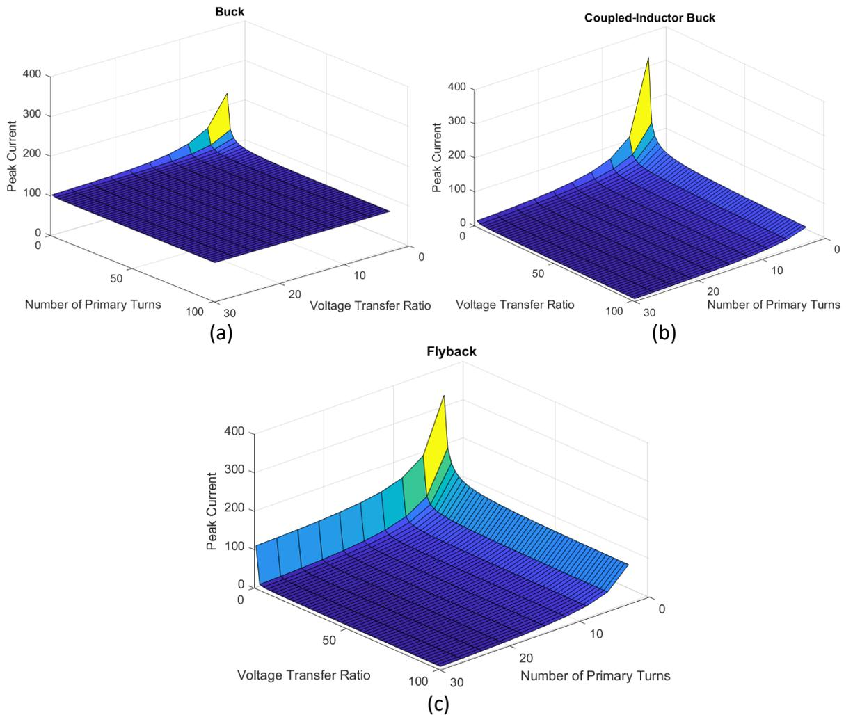
*Fig. 3.3 Maximum switch current for 100A load current versus voltage step-down ratio for each circuit against an increasing No. Primary Turns and (Fixed secondary turns = 3) (a) Buck converter (total turns = No. Primary Turns + 3) (b) Coupled-inductor buck converter (c) Flyback converter*
