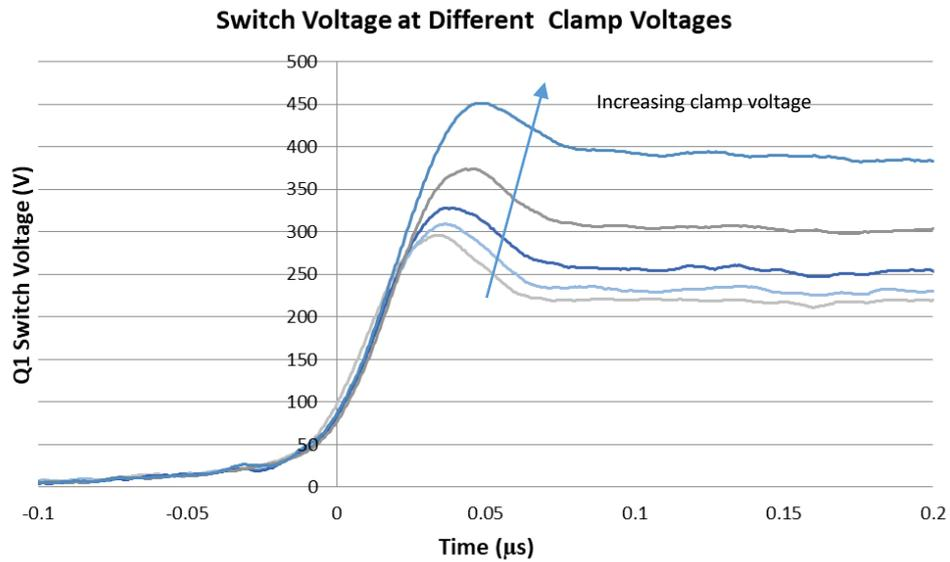
Fig. 4.19 Voltage across main switch Q1 at the turn off transition.
