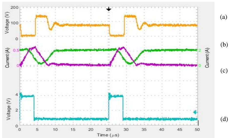
Fig. 4.7 Continuous operation and coupled inductor current transferring from  $L_1$  to  $L_2$ . (a)  $Q_1$  Switch Voltage ( $V_{ds}$ ), (b) Secondary ( $L_2$ ) inductor current, (c) Primary ( $L_1$ ) inductor current, (d)  $Q_1$  Gate Signal ( $V_{gs}$ )
