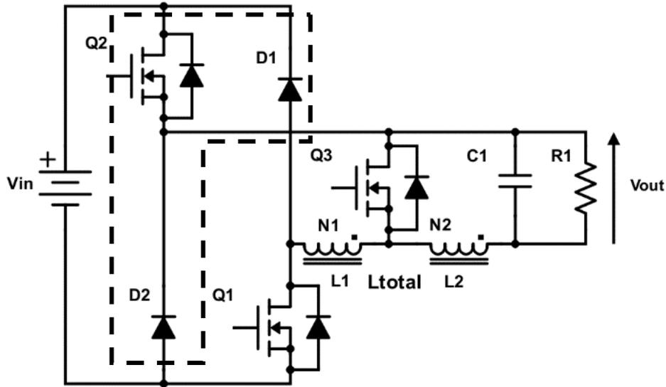
Fig. 5.1 Asymmetrical half-bridge coupled-inductor circuit.
