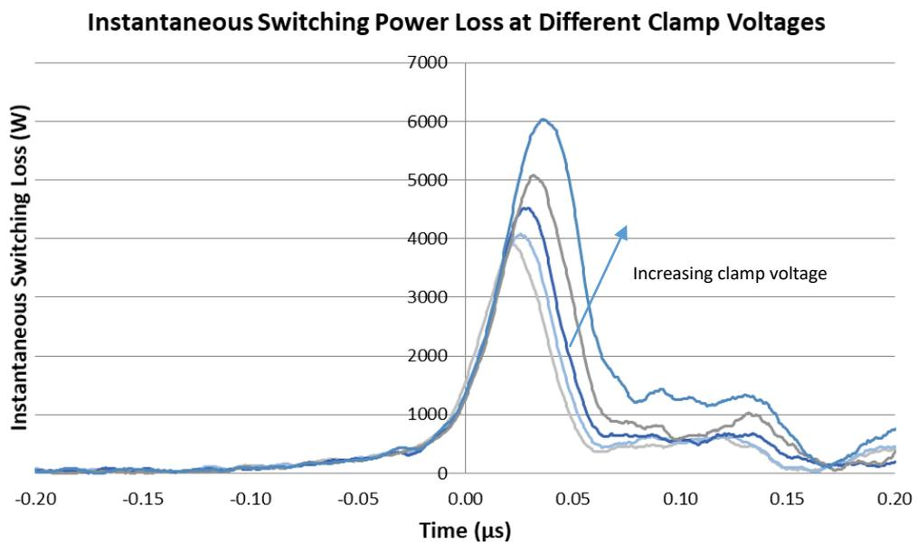
Fig. 4.20 Switching loss dependence on clamping voltage.
