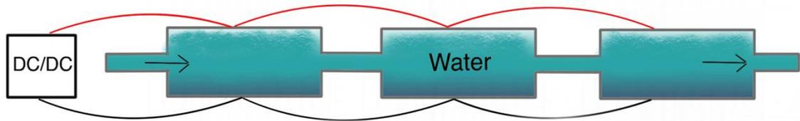
*Fig. 1.4 Water desalination cells arranged in series physically connected in parallel*
