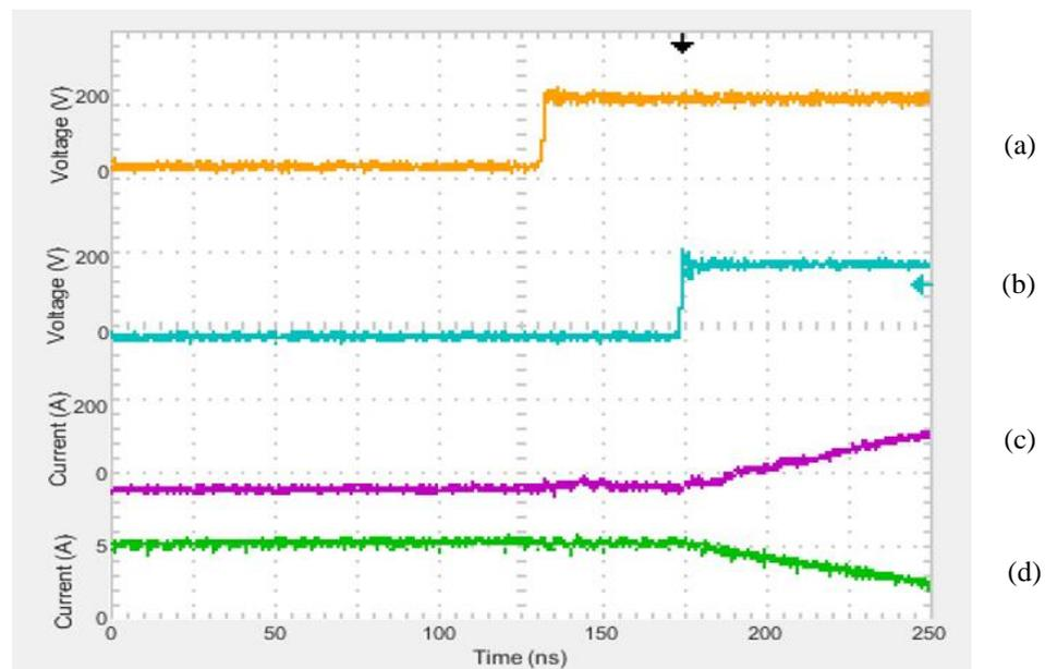
Fig. 6.21 Primary switch turn off for 1.3V super-capacitors. (a)  $Q1$  Switch Voltage ( $V_{ds}$ ), (b)  $Q2$  Switch Voltage ( $V_{ds}$ ), (c) Secondary ( $L2$ ) inductor current, (d) Primary ( $L1$ ) inductor current
