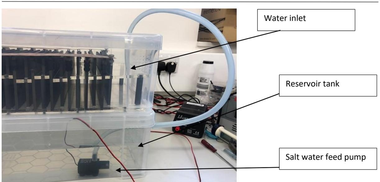
*Fig. v Use of water pumps within the test rig*
