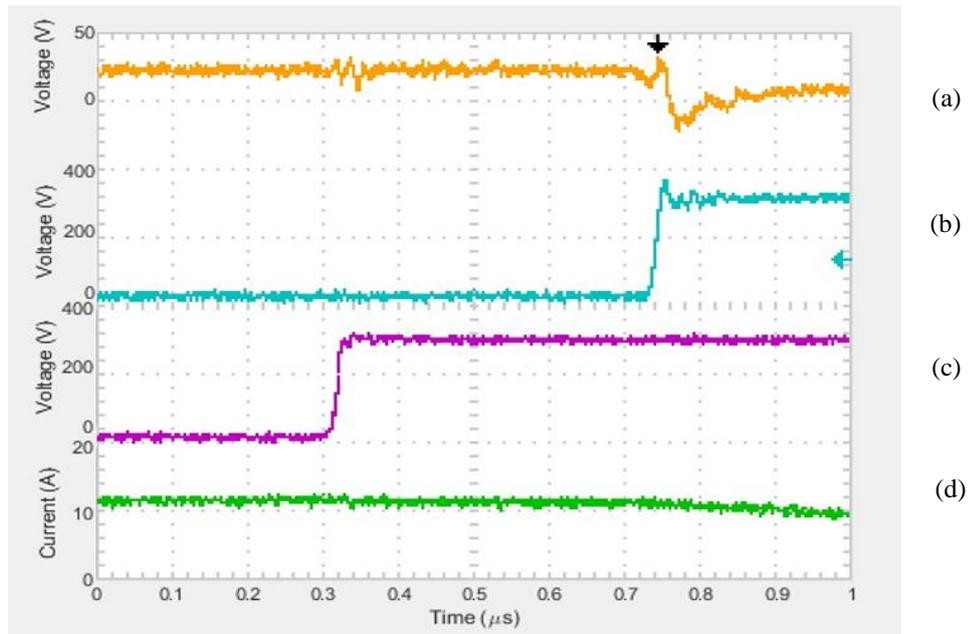
Fig. 6.13 Rising edge showing the delay of the second switch. (a)  $Q3$  Switch Voltage ( $V_{ds}$ ), (b)  $Q1$  Switch Voltage ( $V_{ds}$ ), (c)  $Q2$  Switch Voltage ( $V_{ds}$ ), (d) Primary ( $L1$ ) inductor current
