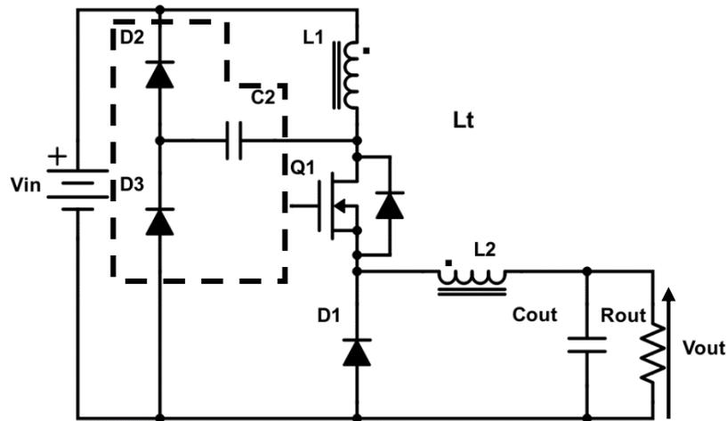
Fig. 2.18 Coupled-inductor buck converter  $S5+/-$  with DCD snubber, (Fig. 4 in [44]).
