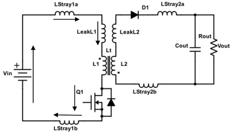
Fig. 2.11 Non idealities on primary side of flyback converter, referred back from the secondary
