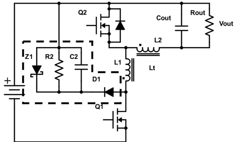
Fig. 2.33 ZRC snubber circuit
