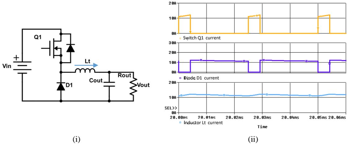
Fig. 2.1 Conventional buck converter: (i) Schematic and (ii) simulated currents of  $Q1$ ,  $D1$  and  $L_t$ .
