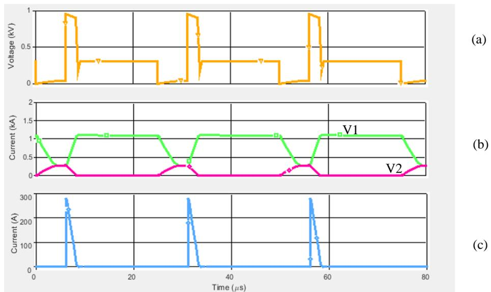
Fig. 2.35 Zener snubber simulation with 3:1 turns ratio and 600V Zener diode threshold voltage. (a) Q1 Switch Voltage ( $V_{ds}$ ), (b)(V1) Secondary ( $L_2$ ) inductor current, (b)(V2) Primary ( $L_1$ ) inductor current, (c) Snubber Diode ( $D_1$ ) current
