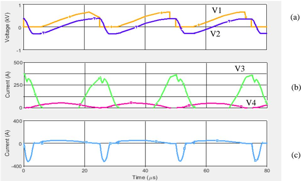
Fig. 2.23 DCDL snubber using 2 $\mu$ F capacitor and 1 $\mu$ H inductor to create resonant operation. (a)(V1) Q1 Switch Voltage ( $V_{ds}$ ), (a)(V2) Capacitor Voltage ( $V_{cap}$ ), (b)(V3) Secondary ( $L_2$ ) inductor current, (b)(V4) Primary ( $L_1$ ) inductor current, (c) Snubber capacitor ( $C_2$ ) current
