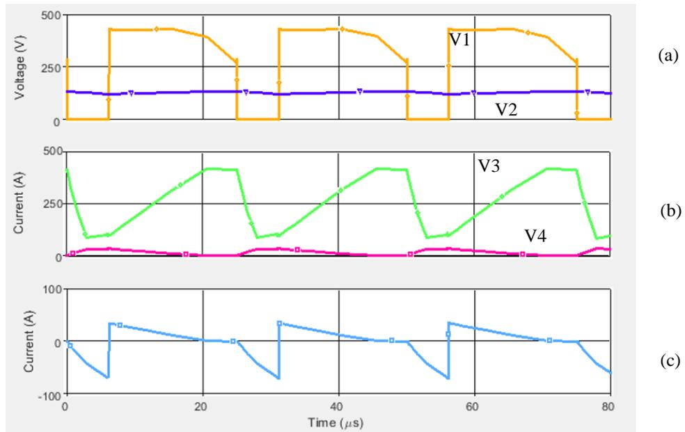
Fig. 2.22 DCDL snubber using  $20\mu\text{F}$  capacitor and  $10\mu\text{H}$  inductor to create clamp operation. (a)(V1) Q1 Switch Voltage ( $V_{ds}$ ), (a)(V2) Capacitor Voltage ( $V_{cap}$ ), (b)(V3) Secondary ( $L_2$ ) inductor current, (b)(V4) Primary ( $L_1$ ) inductor current, (c) Snubber capacitor ( $C_2$ ) current
