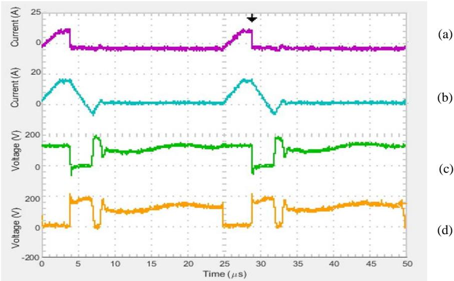
Fig. 5.3 Switching waveforms of the asymmetrical half-bridge coupled-inductor buck converter. (a) Q1 source current, (b) Primary (L1) inductor current, (c) D2 Voltage, (d) Q1 Switch Voltage ( $V_{ds}$ )
