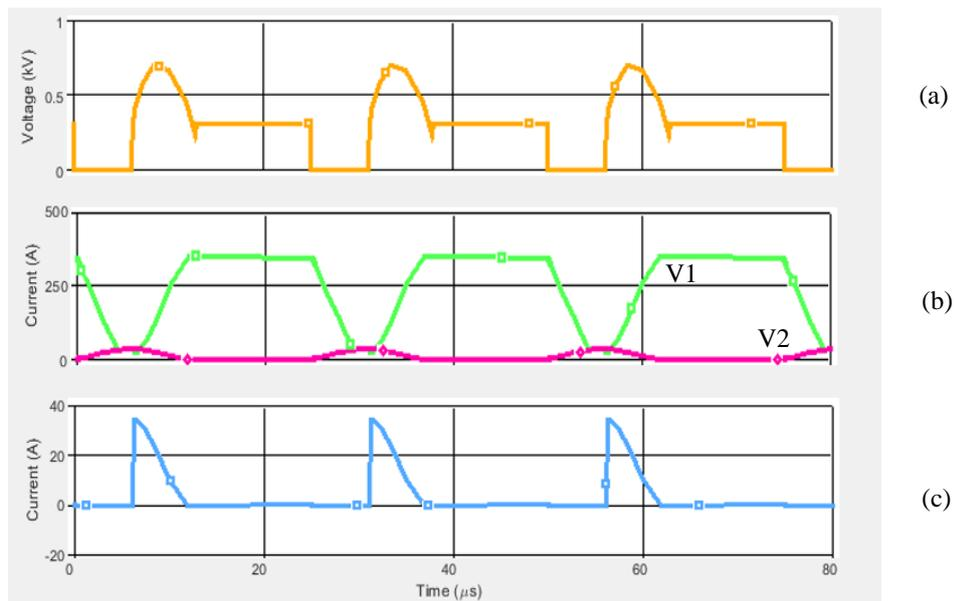
Fig. 2.31 RC snubber simulation with 10:1 turns ratio,  $C_2=700\text{nF}$ ,  $R_2=10\Omega$ . (a)  $Q1$  Switch Voltage ( $V_{ds}$ ), (b)(V1) Secondary ( $L_2$ ) inductor current, (b)(V2) Primary ( $L_1$ ) inductor current, (c) Snubber Diode ( $D1$ ) current
