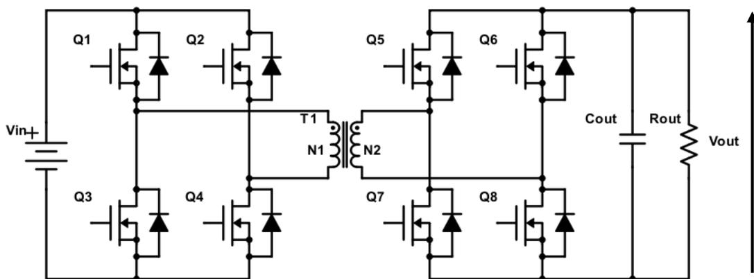
Fig. 2.6 Dual active bridge converter
