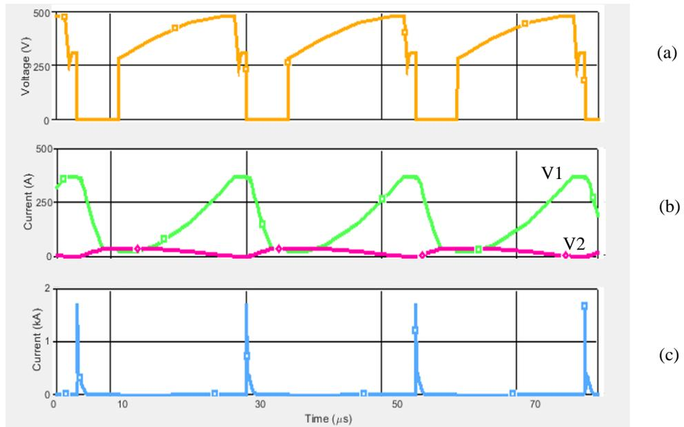
Fig. 2.20 Coupled inductor buck converter simulated with 10:1 turns ratio in  $N1:N2$ . A 1500A current pulse flows through  $Q1$ . (a)  $Q1$  Switch Voltage ( $V_{ds}$ ), (b)(V1) Secondary ( $L2$ ) inductor current, (b)(V2) Primary ( $L1$ ) inductor current, (c) Snubber capacitor ( $C_s$ ) current
