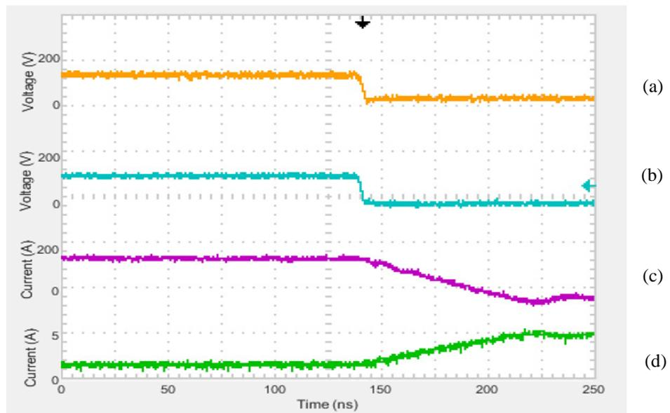
Fig. 6.20 Primary switch turn on for 1.3V super-capacitors. (a)  $Q1$  Switch Voltage ( $V_{ds}$ ), (b)  $Q2$  Switch Voltage ( $V_{ds}$ ), (c) Secondary ( $L2$ ) inductor current, (d) Primary ( $L1$ ) inductor current
