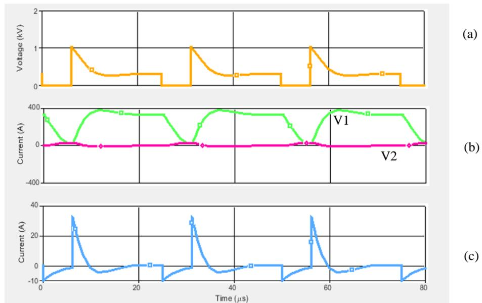
Fig. 2.25 RC Snubber simulation. (a)  $Q1$  Switch Voltage ( $V_{ds}$ ), (b)(V1) Secondary ( $L2$ ) inductor current, (b)(V2) Primary ( $L1$ ) inductor current, (c) Snubber capacitor ( $C1$ ) current
