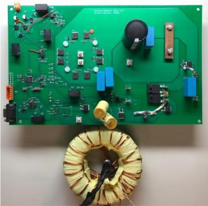
Fig. 4.5 Coupled-inductor circuit prototype
