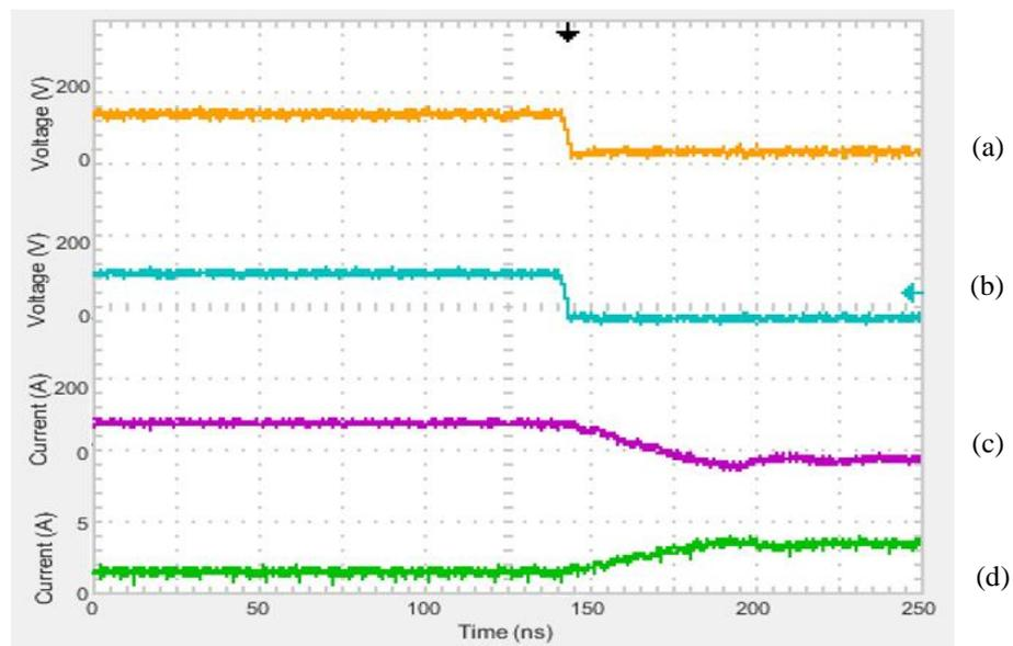
Fig. 6.23 Primary switch turn on for 1.8V super-capacitors. (a)  $Q1$  Switch Voltage ( $V_{ds}$ ), (b)  $Q2$  Switch Voltage ( $V_{ds}$ ), (c) Secondary ( $L2$ ) inductor current, (d) Primary ( $L1$ ) inductor current
