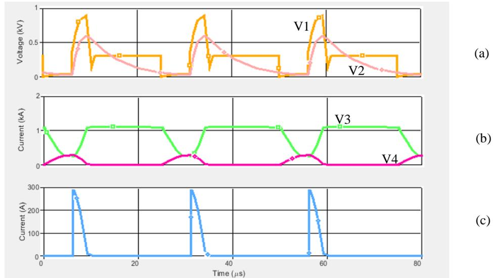
Fig. 2.30 RC snubber simulation with 3:1 turns ratio,  $C_2=700\text{nF}$ ,  $R_2=10\text{ohm}$ . (a)(V1)  $Q1$  Switch Voltage ( $V_{ds}$ ), (a)(V2)  $C_2$  Voltage, (b)(V3) Secondary ( $L_2$ ) inductor current, (b)(V4) Primary ( $L_1$ ) inductor current, (c) Snubber Diode ( $D1$ ) current
