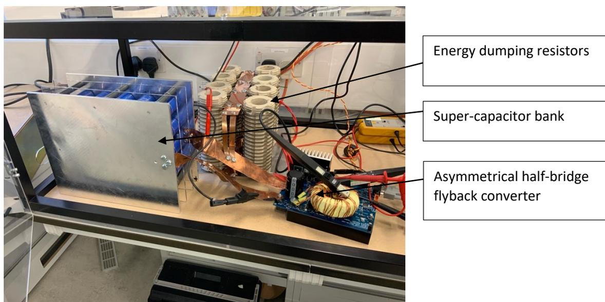
*Fig. 6.16 Complete super-capacitor test setup*
