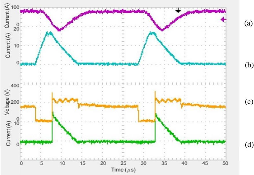
Fig. 4.14 Circuit waveforms at clamp voltage of 250V. (a) Secondary (L2) inductor current, (b) Primary (L1) inductor current, (c) Q1 Switch Voltage (Vds), (d) Snubber diode current (D1)
