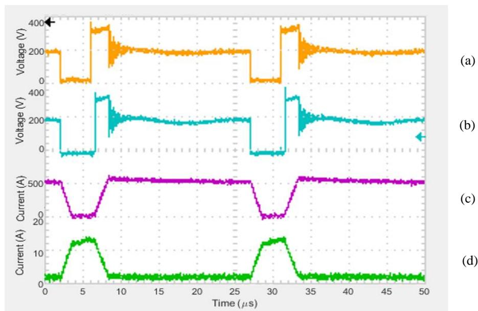
Fig. 6.26 340V input voltage with 550A output current. (a) Q1 Switch Voltage ( $V_{ds}$ ), (b) Q2 Switch Voltage ( $V_{ds}$ ), (c) Secondary ( $L2$ ) inductor current, (d) Primary ( $L1$ ) inductor current
