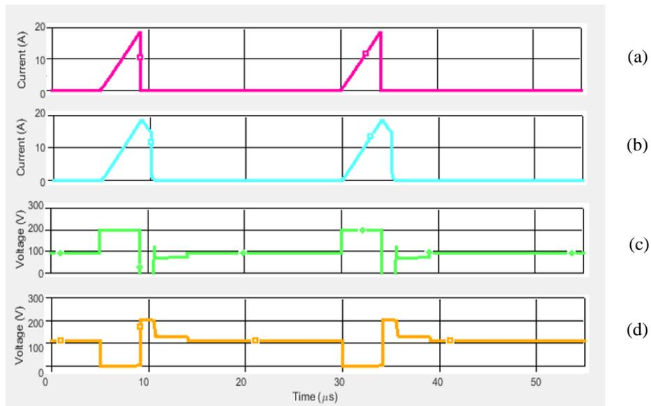
Fig. 5.2 Simulated switching waveforms of the asymmetrical half-bridge coupled-inductor buck converter. (a)  $Q1$  source current, (b) Primary ( $L1$ ) inductor current, (c)  $D2$  Voltage, (d)  $Q1$  Switch Voltage ( $V_{ds}$ )
