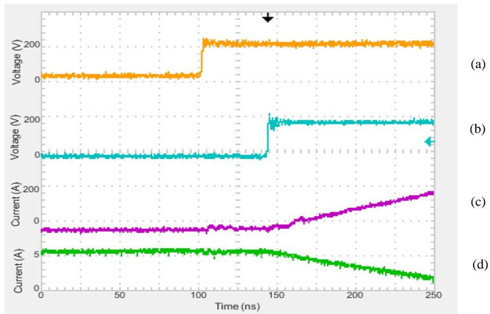
Fig. 6.18 Primary switch turn off showing delay to reduce zero volt ringing at 0.8V. (a)  $Q1$  Switch Voltage ( $V_{ds}$ ), (b)  $Q2$  Switch Voltage ( $V_{ds}$ ), (c) Secondary ( $L2$ ) inductor current, (d) Primary ( $L1$ ) inductor current
