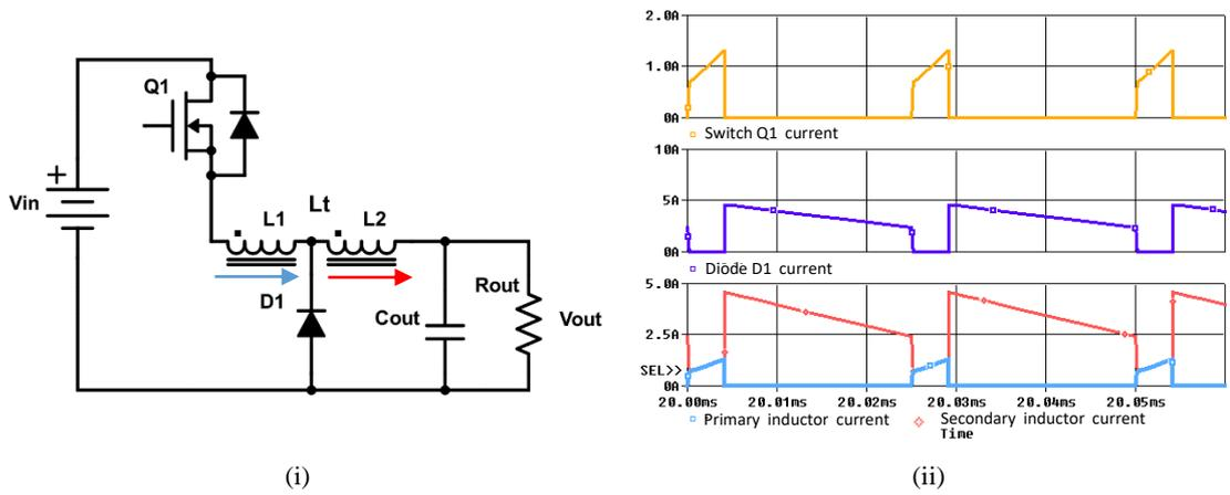
Fig. 2.9. Coupled-inductor buck converter S5+/- [46]: (i) Schematic and (ii) simulated currents for switch Q1, diode D1 and the primary and secondary of Lt.
