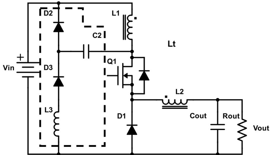
Fig. 2.21 Inductor added to DCD snubber for controlled discharge current
