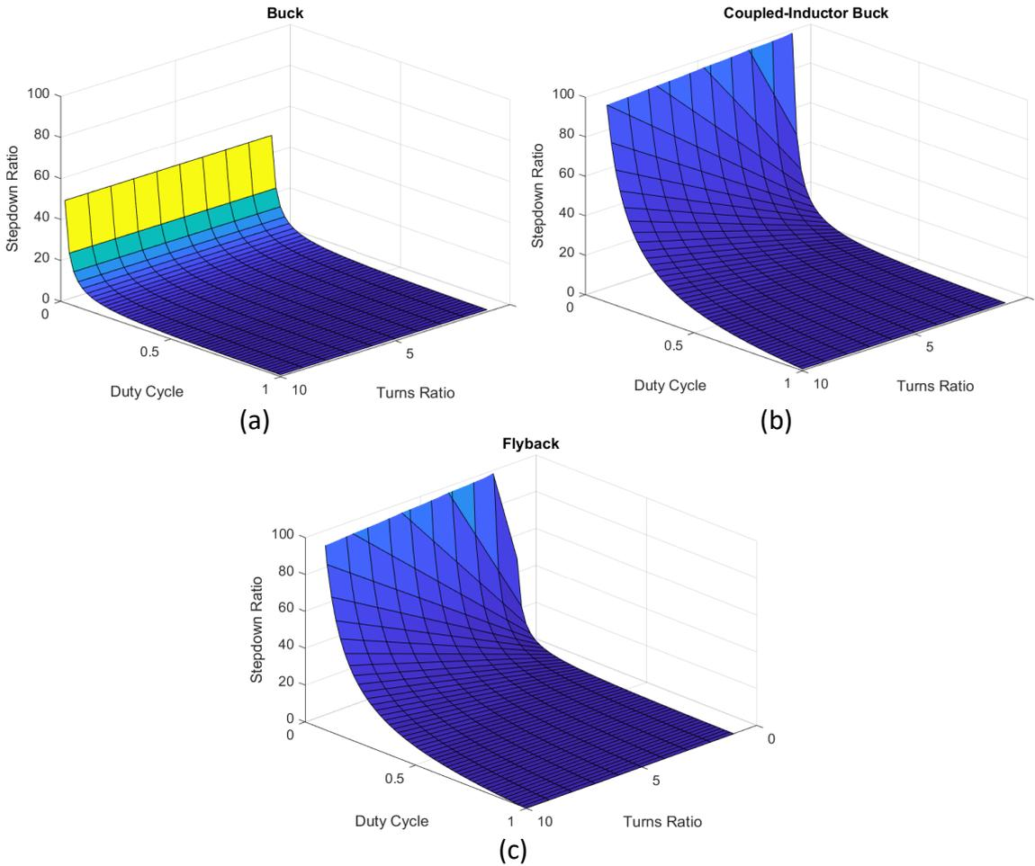
Fig. 3.2 Voltage transfer ratio versus turns ratio, (a) buck, (b) coupled-inductor buck and (c) flyback.
