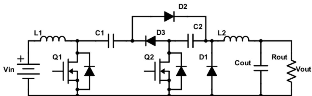
Fig. 2.5 Multi-stage Cuk converter.
