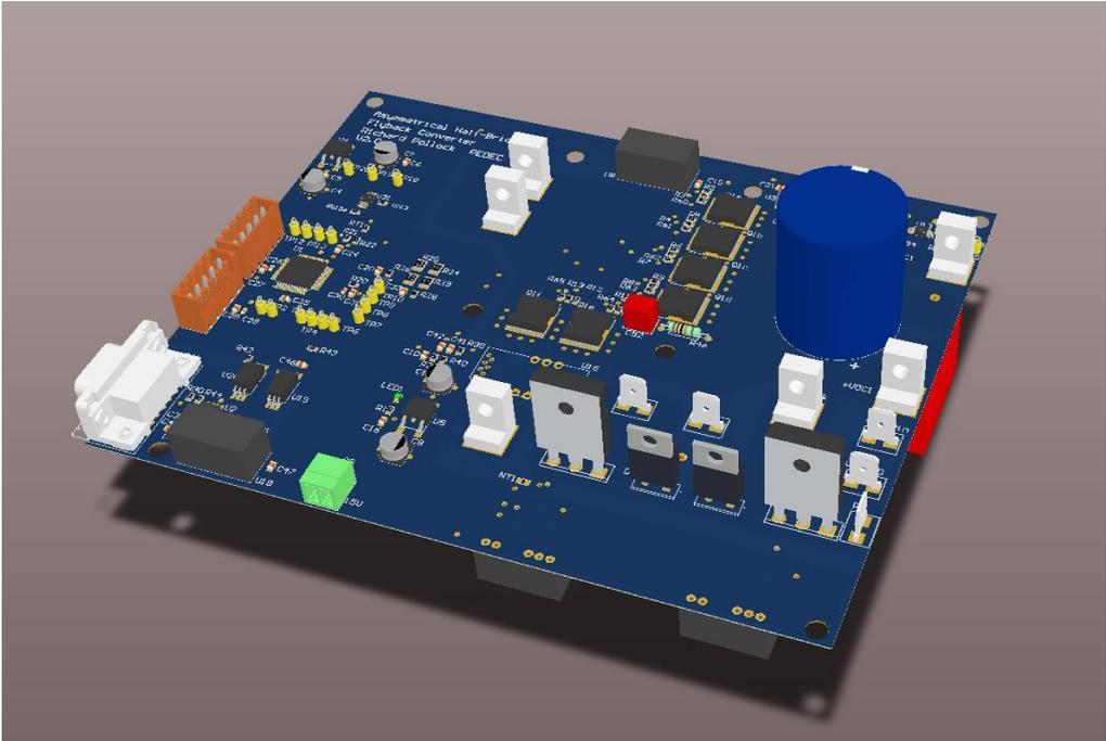
Fig. 6.3 3D model of final PCB design
