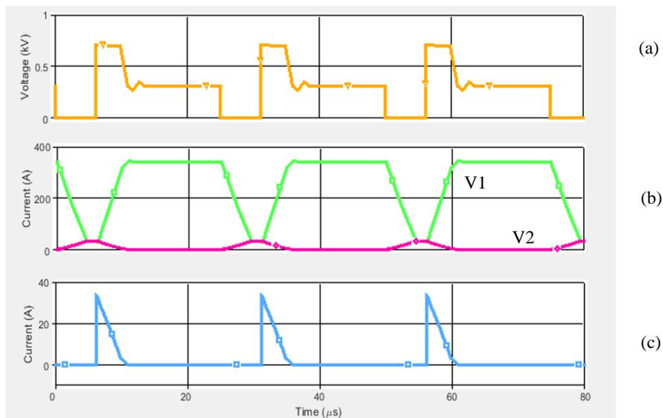
Fig. 2.36 Zener snubber simulation with 10:1 turns ratio and 400V Zener snubber threshold voltage. (a) Q1 Switch Voltage ( $V_{ds}$ ), (b)(V1) Secondary ( $L_2$ ) inductor current, (b)(V2) Primary ( $L_1$ ) inductor current, (c) Snubber Diode ( $D_1$ ) current
