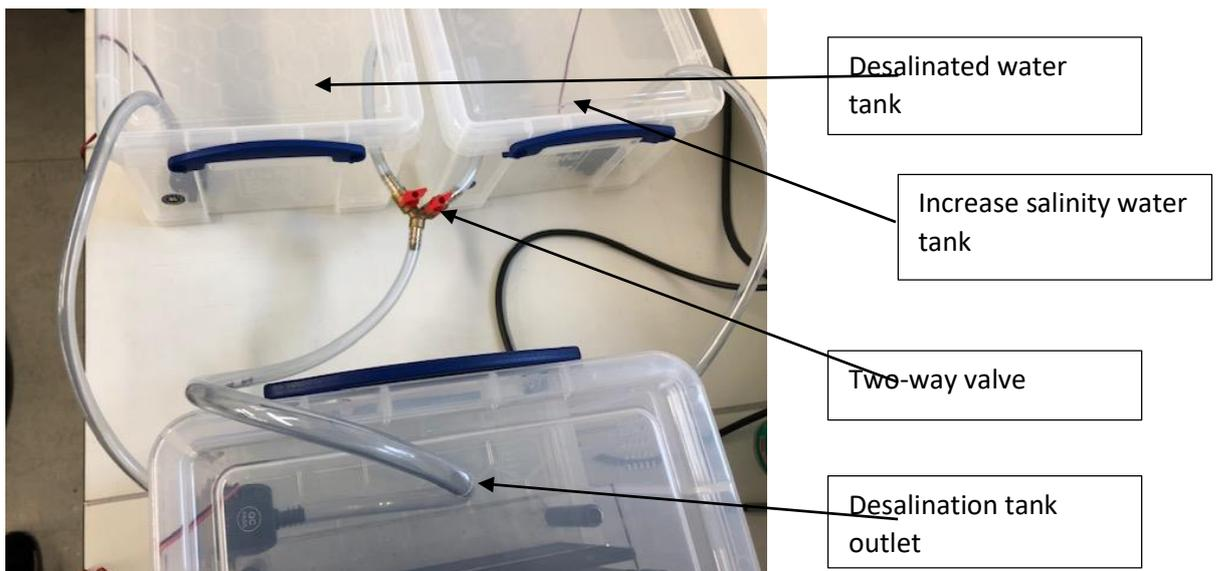
*Fig. vi Tubing to determine the path of the flow at the output of the cell.*
