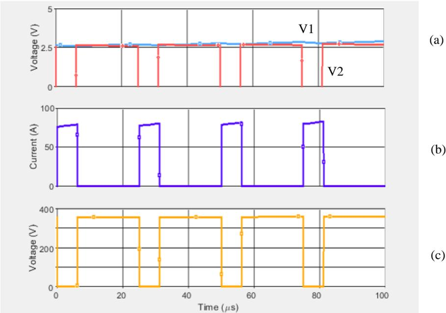
Fig. 2.12 simulation showing referred voltage (a)(V1) Output Voltage ( $V_{out}$ ), (a)(V2) Diode Voltage ( $V_{D1}$ ), (b) Primary ( $L1$ ) inductor current, (c)  $Q1$  Switch Voltage ( $V_{ds}$ )
