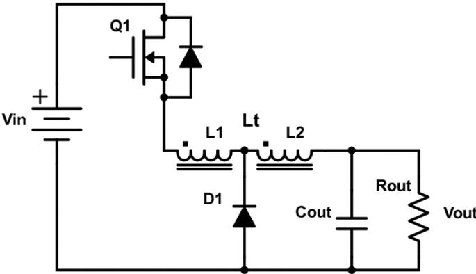
Fig. 2.13 Coupled-inductor buck converter,  $S5+/-$
