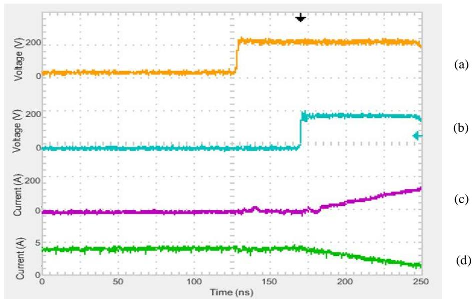
Fig. 6.24 Primary switch turn off for 1.8V super-capacitors. (a)  $Q1$  Switch Voltage ( $V_{ds}$ ), (b)  $Q2$  Switch Voltage ( $V_{ds}$ ), (c) Secondary ( $L2$ ) inductor current, (d) Primary ( $L1$ ) inductor current
