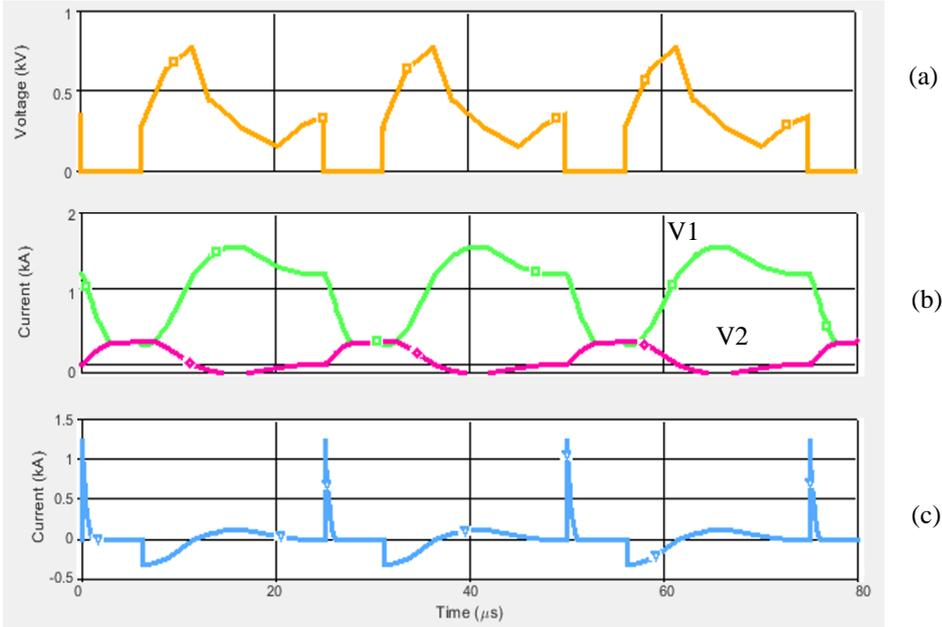
Fig. 2.19 Coupled-inductor buck converter simulated with 3:1 turns ratio in  $N1:N2$ . A 1000A capacitor current flows through Q1. (a) Q1 Switch Voltage ( $V_{ds}$ ), (b)(V1) Secondary (L2) inductor current, (b)(V2) Primary (L1) inductor current, (c) Snubber capacitor ( $C_s$ ) current
