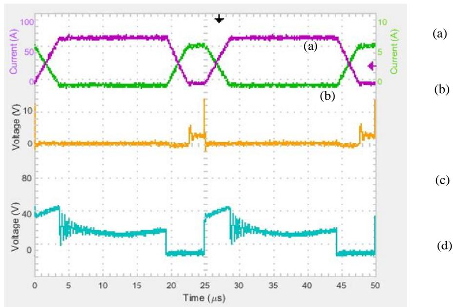
Fig. 6.8 Initial testing of Asymmetrical half-bridge flyback converter. (a) Secondary ( $L_2$ ) inductor current, (b) Primary ( $L_1$ ) inductor current, (c)  $Q_3$  Switch Voltage ( $V_{ds}$ ), (d)  $Q_1$  Switch Voltage ( $V_{ds}$ )
