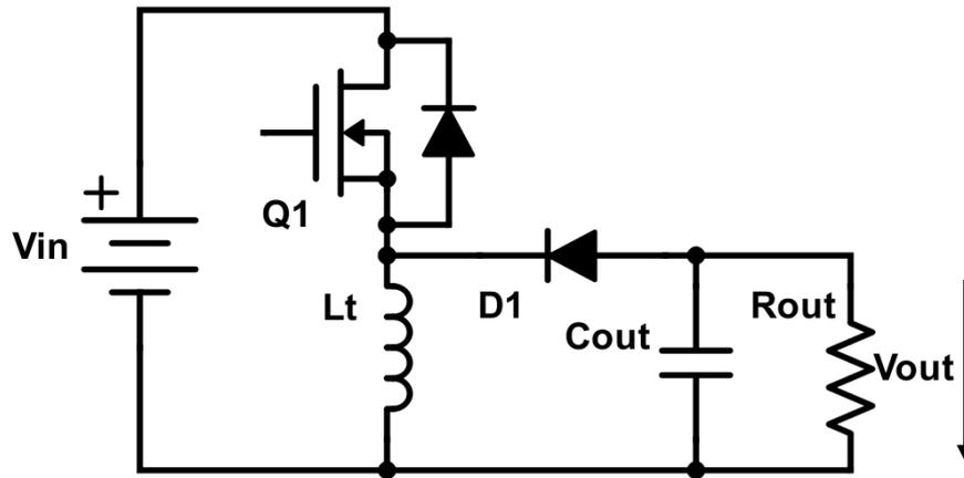
Fig. 2.2 Buck-boost converter
