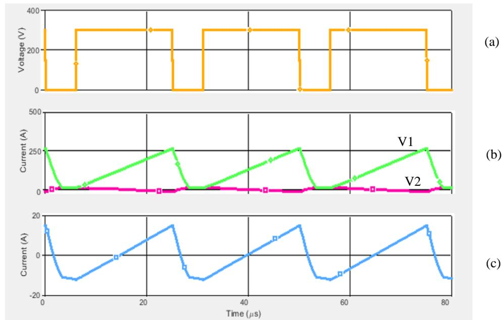
Fig. 2.16 Ultra high stepdown converter simulated with 10:1 turns ratio. (a)  $Q1$  Switch Voltage ( $V_{ds}$ ), (b)(V1) Secondary ( $L2$ ) inductor current, (b)(V2) Primary ( $L1$ ) inductor current, (c) Snubber capacitor ( $C_s$ ) current
