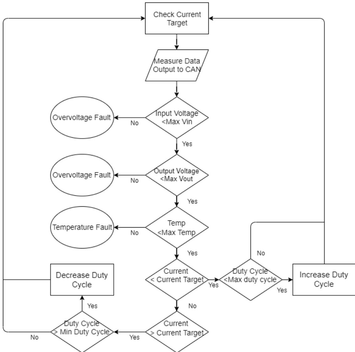
Fig. 6.7 Simplified Software Flowchart
