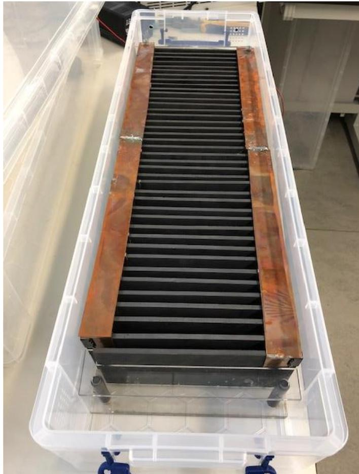
*Fig. iv Assembled desalination cell desalination test tank*
