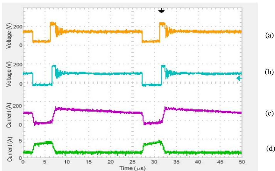
Fig. 6.25 Two full switching cycles for 1.8V super-capacitors. (a)  $Q1$  Switch Voltage ( $V_{ds}$ ), (b)  $Q2$  Switch Voltage ( $V_{ds}$ ), (c) Secondary ( $L2$ ) inductor current, (d) Primary ( $L1$ ) inductor current
