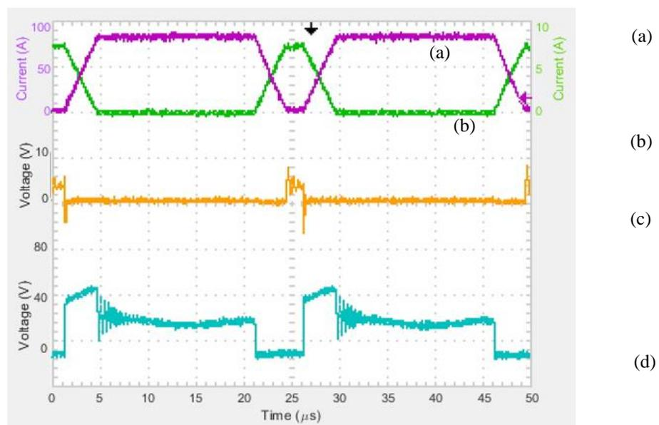
Fig. 6.9 Delayed primary switches reducing secondary switch voltage. (a) Secondary ( $L_2$ ) inductor current, (b) Primary ( $L_1$ ) inductor current, (c)  $Q_3$  Switch Voltage ( $V_{ds}$ ), (d)  $Q_1$  Switch Voltage ( $V_{ds}$ )
