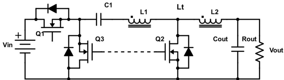
Fig. 2.14 Ultra high step-down ratio converter [50]
