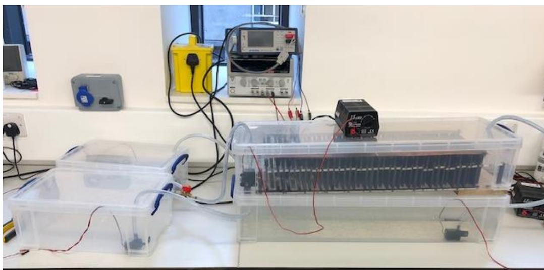
*Fig. 6.15 Water desalination test rig*
