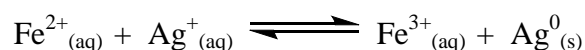
Figure 1-31 The redox reaction that is the chemical basis for the PD process [75]
