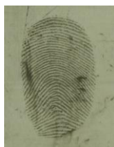
Figure 1-39 Powder suspension enhanced fingerprint on uPVC
