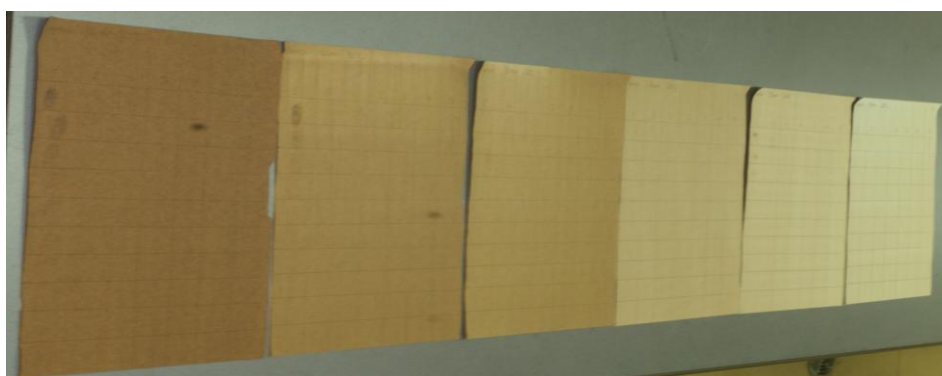
Figure 3-8 Photograph of paper subjected to 200°C - aged for 1 month.
