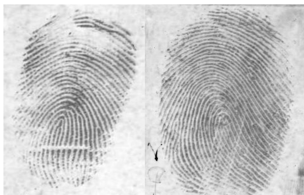
Figure 4-15 Photograph of eccrine (left – which was scored as grade 3) and sebaceous (right – which was scored as grade 4) fingerprints on glass subjected to 250°C for 10 min - aged for 1 day
