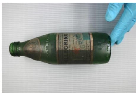
Figure 5-19 Photograph of glass bottle – half of which has been treated with lifting tape and Absorene
