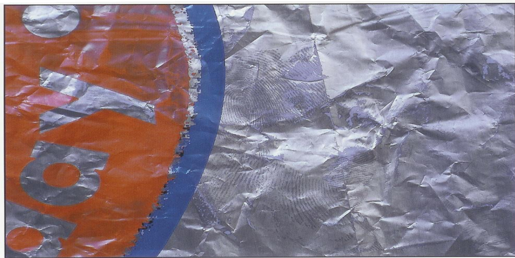
Figure 1-38 VMD on a high density polythene bag [101]
