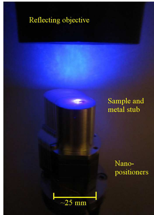
Figure 7.1: Photo depicting PL mapping with moving nanopositioners and sample luminescence. The sample is mounted on to a metal stub which is connected to the movable positioners and a reflecting objective is used to focus the laser light and collect the emission from the sample. The size of the positioners are given for scale purposes.
