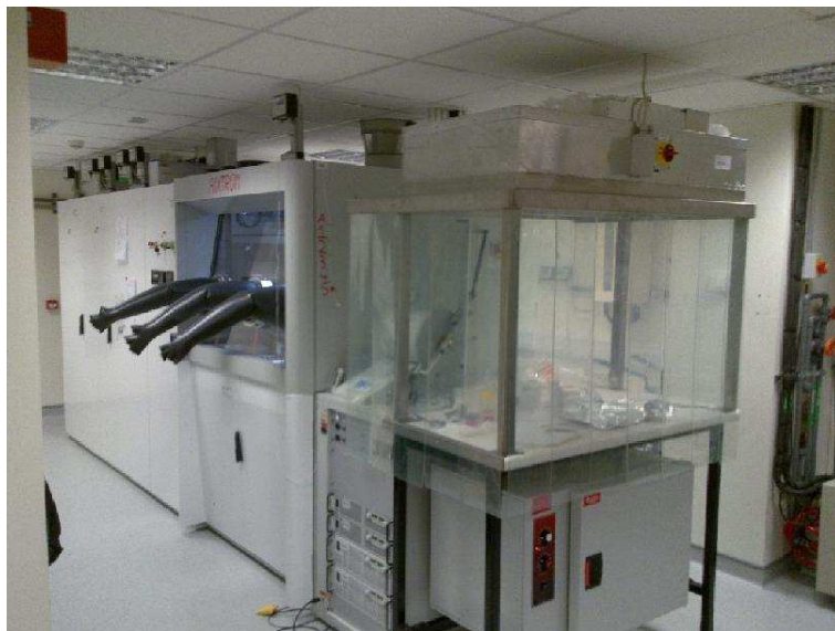
Figure 3.1: MOCVD reactor used at Tyndall National Institute. This is an 3\times 2 " AIXTRON close-coupled showerhead MOCVD reactor. Image taken from http://www.tyndall.ie/content/nitride-materials-0 .
