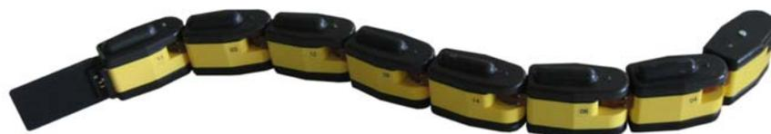
Figure 1.14 An amphibious snake robot, AmphiBot.
