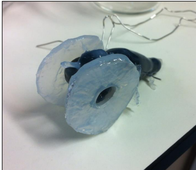
Figure 62 - Dip coated dummy device with attached sewing rings
