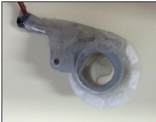
Figure 98 - Final single ring open mould, with Dacron
