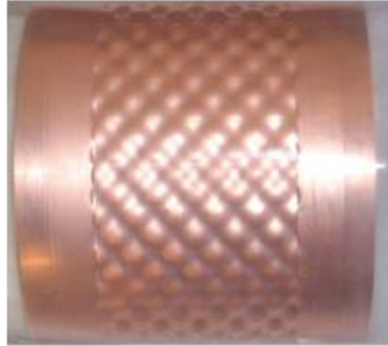
Figure 4.1(a): Photograph of the cylindrical 2D periodic structure which forms the cavity, having diameter 80mm, corrugation depth 1mm, 28 azimuthal variations and longitudinal period equal to 8mm.
