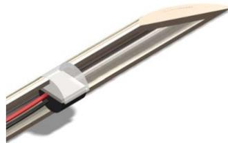
**Figure 5.** Drawing of single element transducer in needle.
