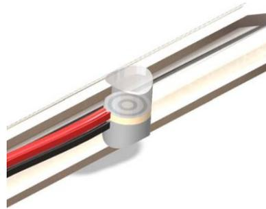
**Figure 7.** Drawing of a side-viewing annular array positioned in a needle
