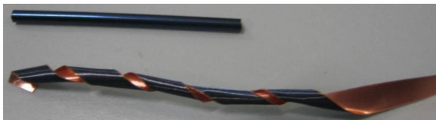
**Figure 14.** An example of a helical circuit next to a 2 mm diameter tungsten tube.
