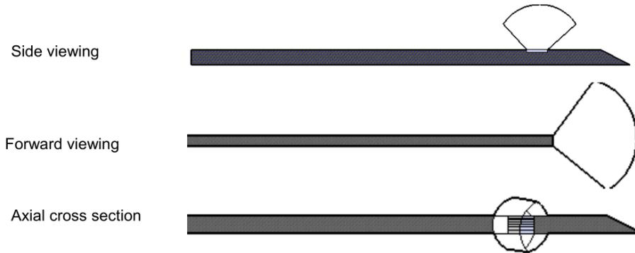
**Figure 1.** Diagrams of transducer configurations for (a) a side viewing linear array, (b) forward viewing linear phased array and (c) axial cross section with single element transducers or annular arrays.
