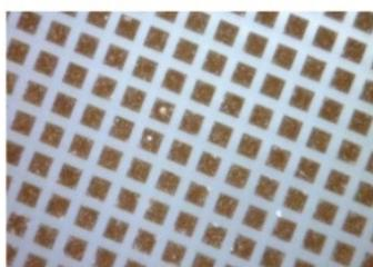
**Figure 4.** An example of a piezocomposite made by dice and fill method. The brown pillars are surrounded by transparent epoxy
