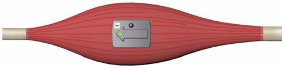
Figure (19): Trigno™ Wireless Sensor Oriented with Muscle Fiber (Delsys, 2012, pp.16)
