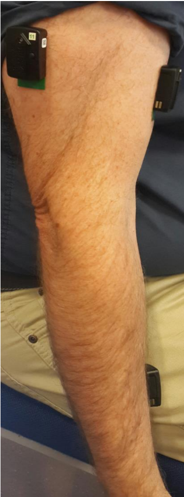
Figure (20): EMG Data Recording using Trigno™ wireless sensors
