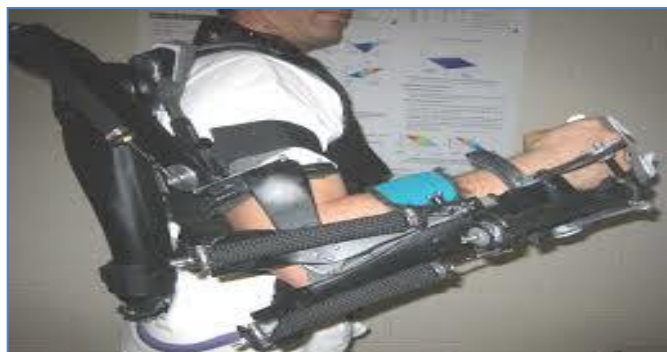
Figure (15): Pneumatic muscle actuator prototype (Chang M.K., 2010)
