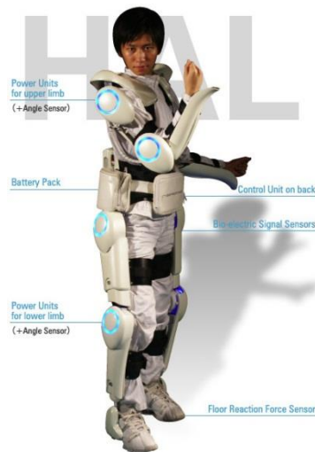
Figure (2): Hybrid Assistive Limb (HAL) exoskeleton prototype
