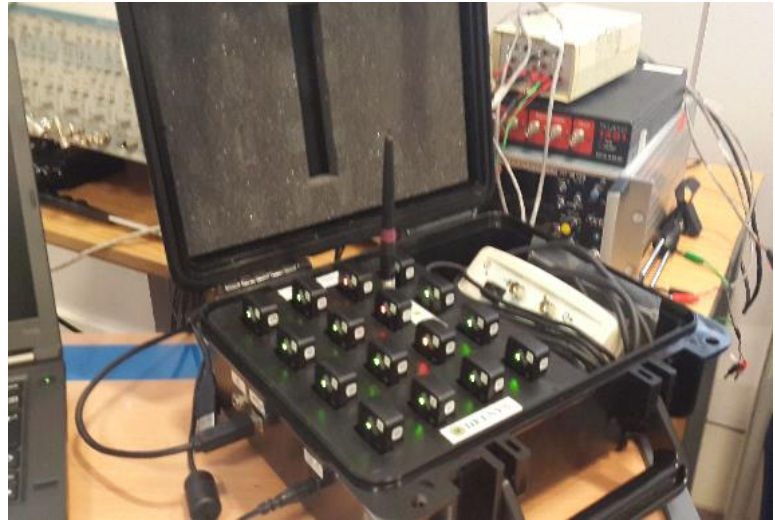
Figure (21): Trigno™ Wireless EMG System
