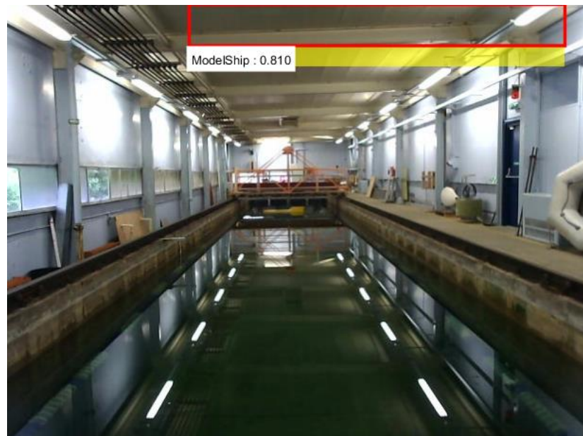
Figure 5.16 Visualisation of distance estimation and object recognition at the time of 277 sec in case 2. The numbers above the bounding box indicate the estimated distance, and the text below indicates the classification result and corresponding matching probability.
