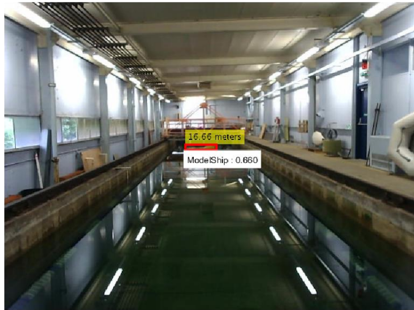
Figure 5.15 Visualisation of distance estimation and object recognition at the time of 277 sec in case 1. The numbers above the bounding box indicate the estimated distance, and the text below indicates the classification result and corresponding matching probability.
