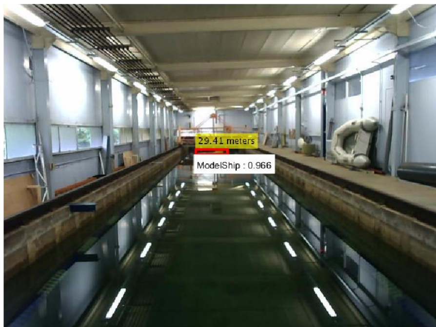
Figure 5.13 Visualisation of distance estimation and object recognition at the time of 231 sec in case 1. The numbers above the bounding box indicate the estimated distance, and the text below indicates the classification result and corresponding matching probability.
