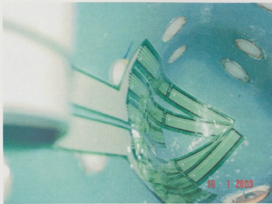
Figure 6.13: F-Socket™ sensor attached with non aggressive spray glue to the socket
