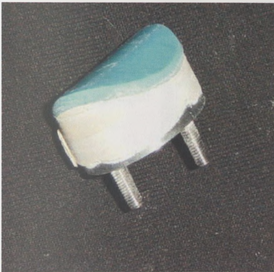
Figure 4.3: Cut off patellar tendon bar curvature sensing surface bonded to the patellar tendon bar holder by Akemi-Putty (Ottobock Healthcare, GmbH, DUDERSTADT, Germany).
