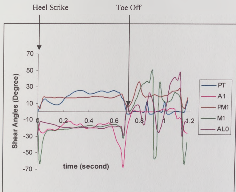
Figure 7.70: Example of shear angles during gait for subject #7 wearing a PTB socket.
