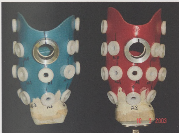
Figure 6.9: PTB socket (left) and Hydrocast socket (right); Transducer locations for the subject no. 4
