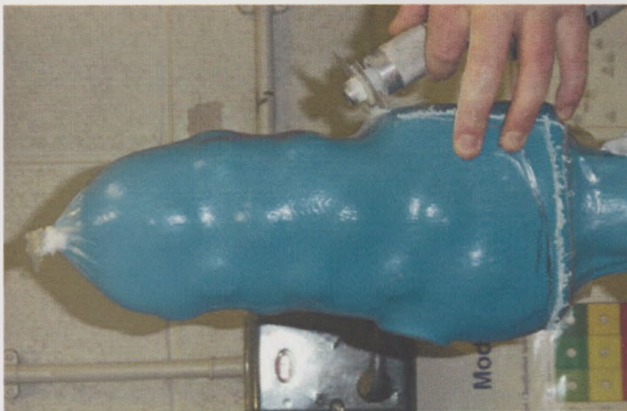
Figure 6.2 : Laminated socket with metal inserts.
