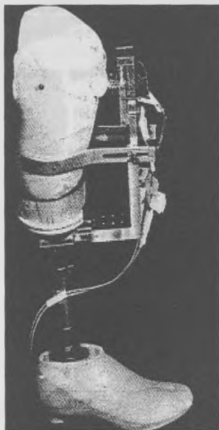
Figure 3.6: Biaxial stress measurement on the patellar tendon. (Adapted from Mizrahi et al, 1985).
