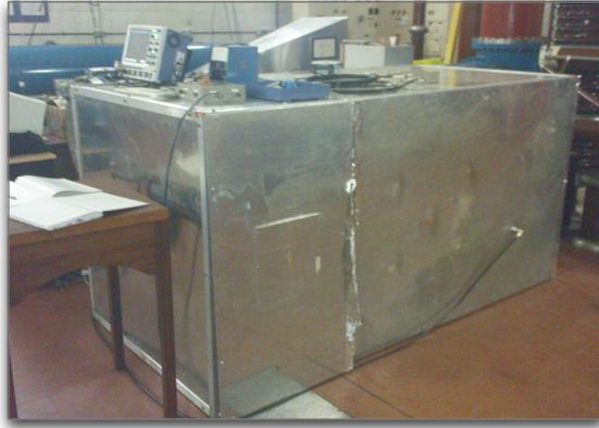
(a) External view of the aluminium PD test enclosure
