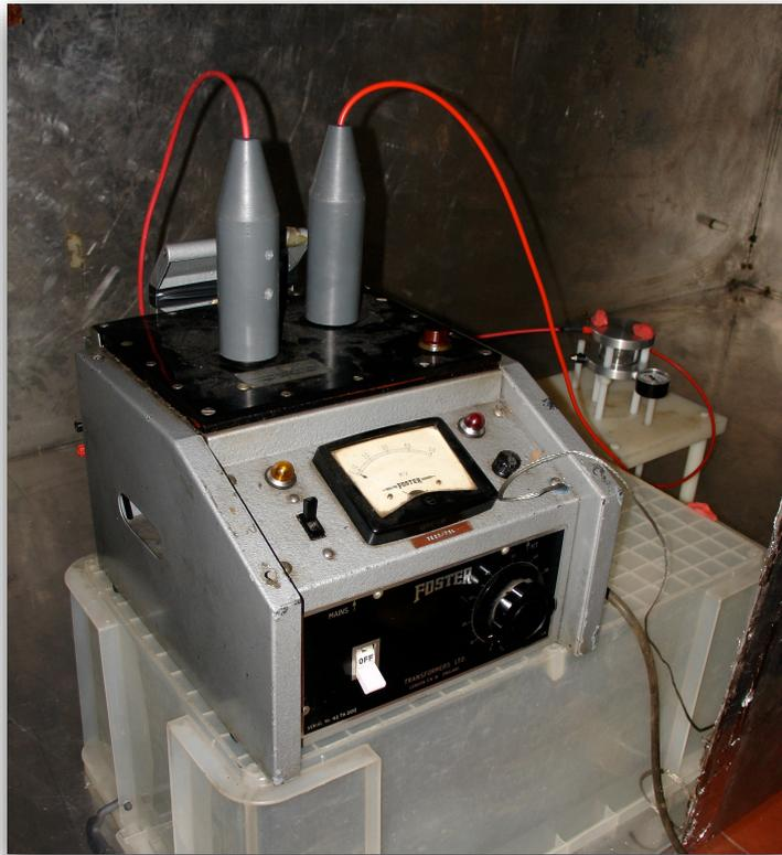
Figure 5.12: Internal view of RF test tank, with 50kV transformer and one of the test cells on an insulation platform behind
