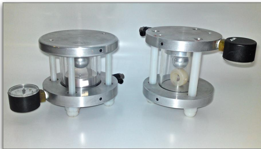
Figure 5.11: Examples of the test cells used for experimentation. To the left, the rolling particle test cell, and to the right, the floating electrode test cell
