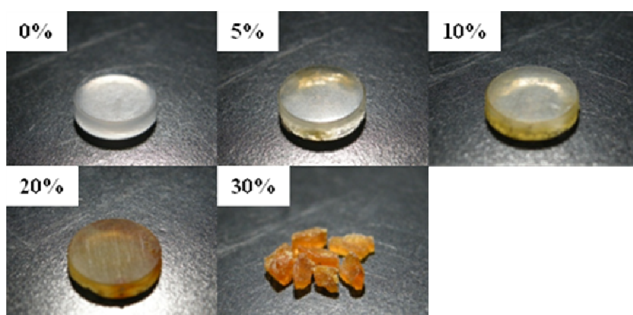
Fig. 4.32 PP47 samples treated to various levels of degradation in TGA
