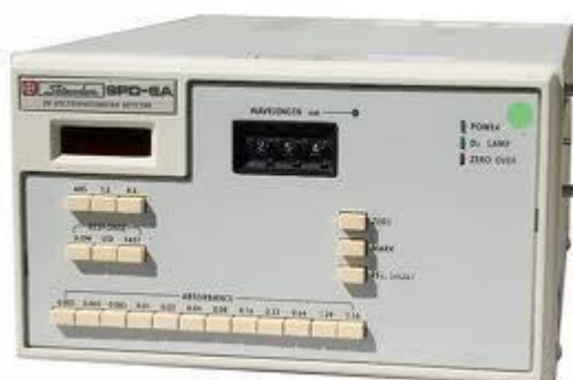
Figure 3.2 – Shimadzu SPD-6A variable wavelength UV detector. 113
