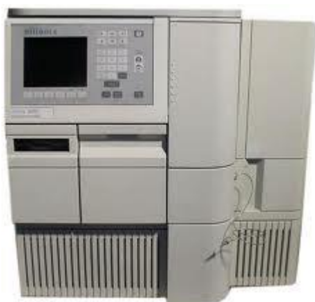
Figure 3.1 – Waters 2690 HPLC system. 112
