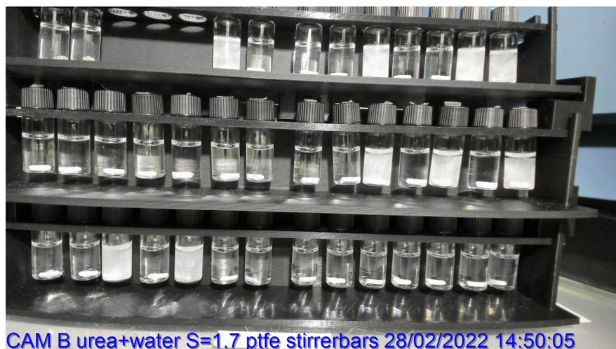
Figure 3.2: Example webcam image from this work. Crystallisation has taken place in nine vials and PTFE stirrer bars are seen at the bottom of most vials.
