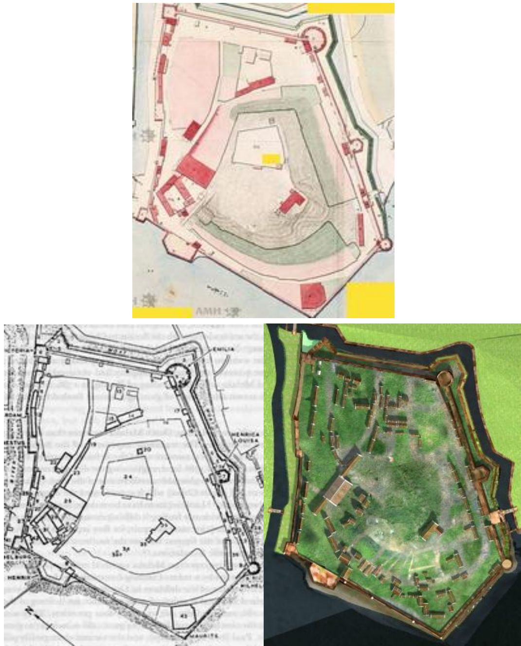
Figure 4.32 Comparison of the selected plans with the 3D reconstructed plan. From above 'Map of the city and fortress at Malacca, 1780' (Source: NA, 2008), below left ' Plan of Malacca fortress, ca. 1792, (after Reimer and Elias)' (Source: Harrison,1986) and below right '3D reconstructed plan' (Source: Author).
