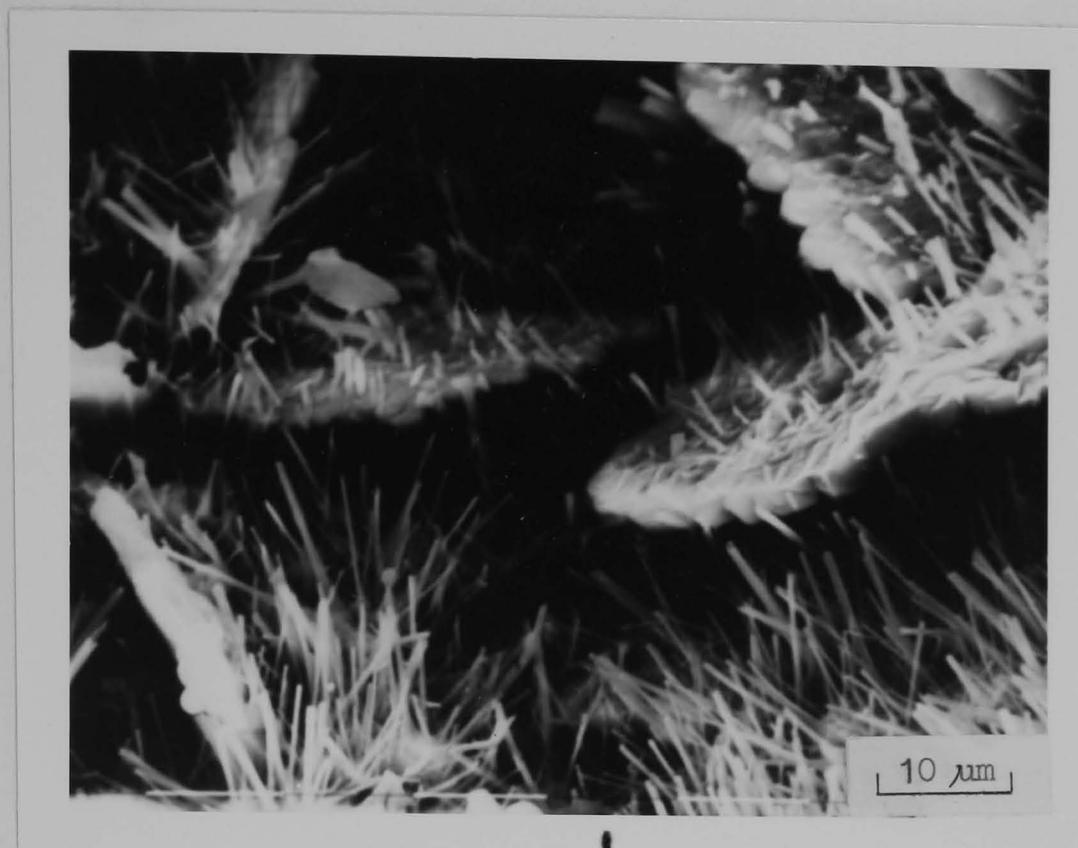
Fig. 6.19 SEM micrograph of paste specimen (W/C = 0.4) cured normally for 7 days and subjected to 54 freeze/thaw cycles in saturated solution of sodium chloride (Mag. 1250)
