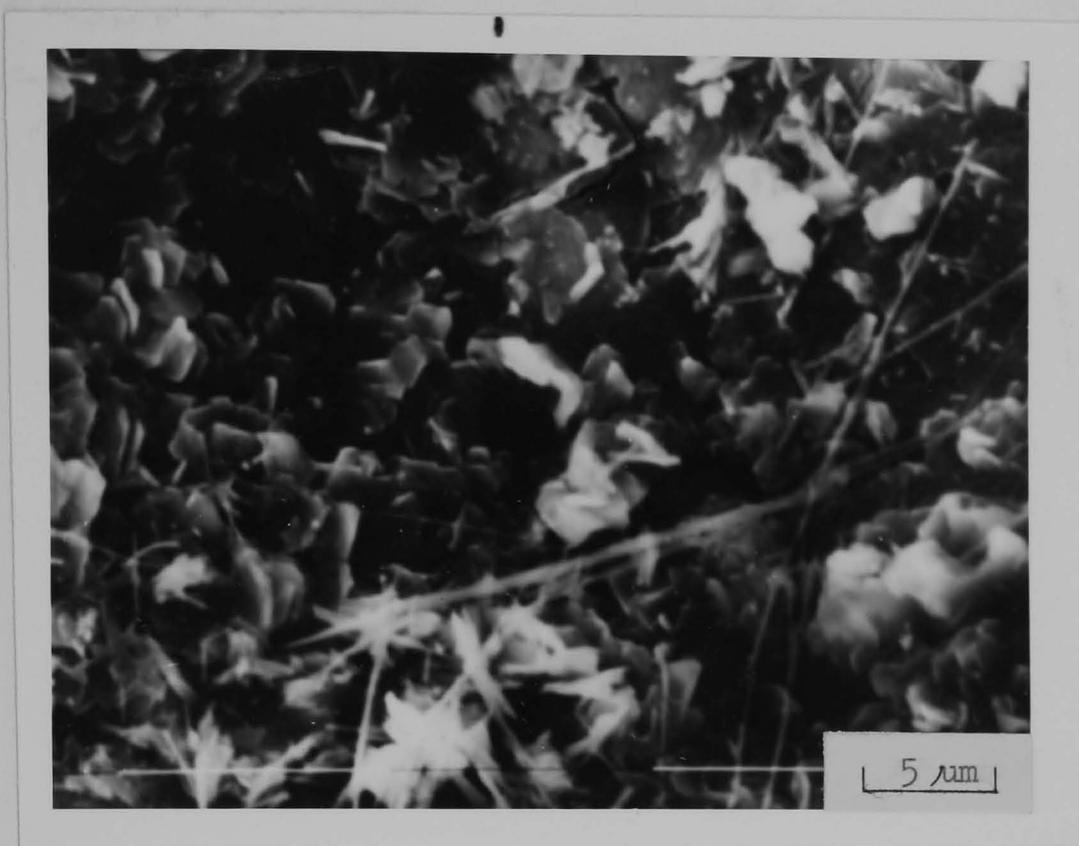
Fig. 6.15 SEM micrograph of a paste specimen (W/C = 0.4) cured normally for 7 days and subjected to 72 freeze/thaw cycles in 4% salt solution (Mag.2500)
