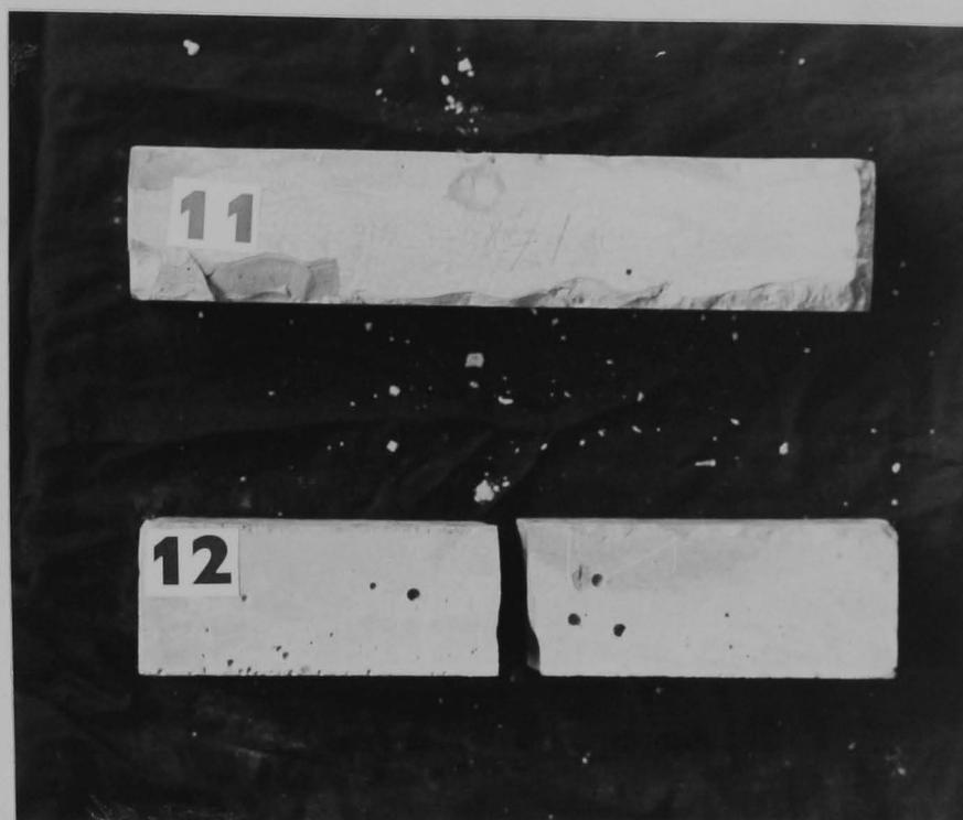
Fig. 9.9 Effect of 216 freeze/thaw cycles on cement paste (W/C = 0.4) initially cured for 28 days in (11) 4% and (12) saturated solution of sodium chloride
