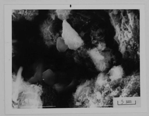
Fig. 6.8 SEM micrograph of a specimen of cement paste (W/C = 0.4) cured normally for 3 days and subjected to 54 freeze/thaw cycles in 0% salt solution (Mag. 2500)
