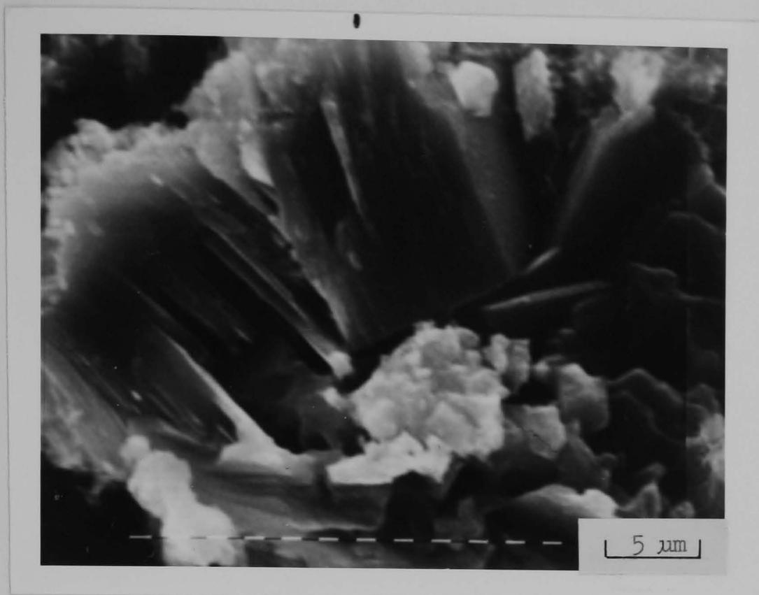
Fig. 6.5 SEM micrograph of a specimen of cement paste (W/C = 0.4) cured normally for 28 days. (Mag. 2500)
