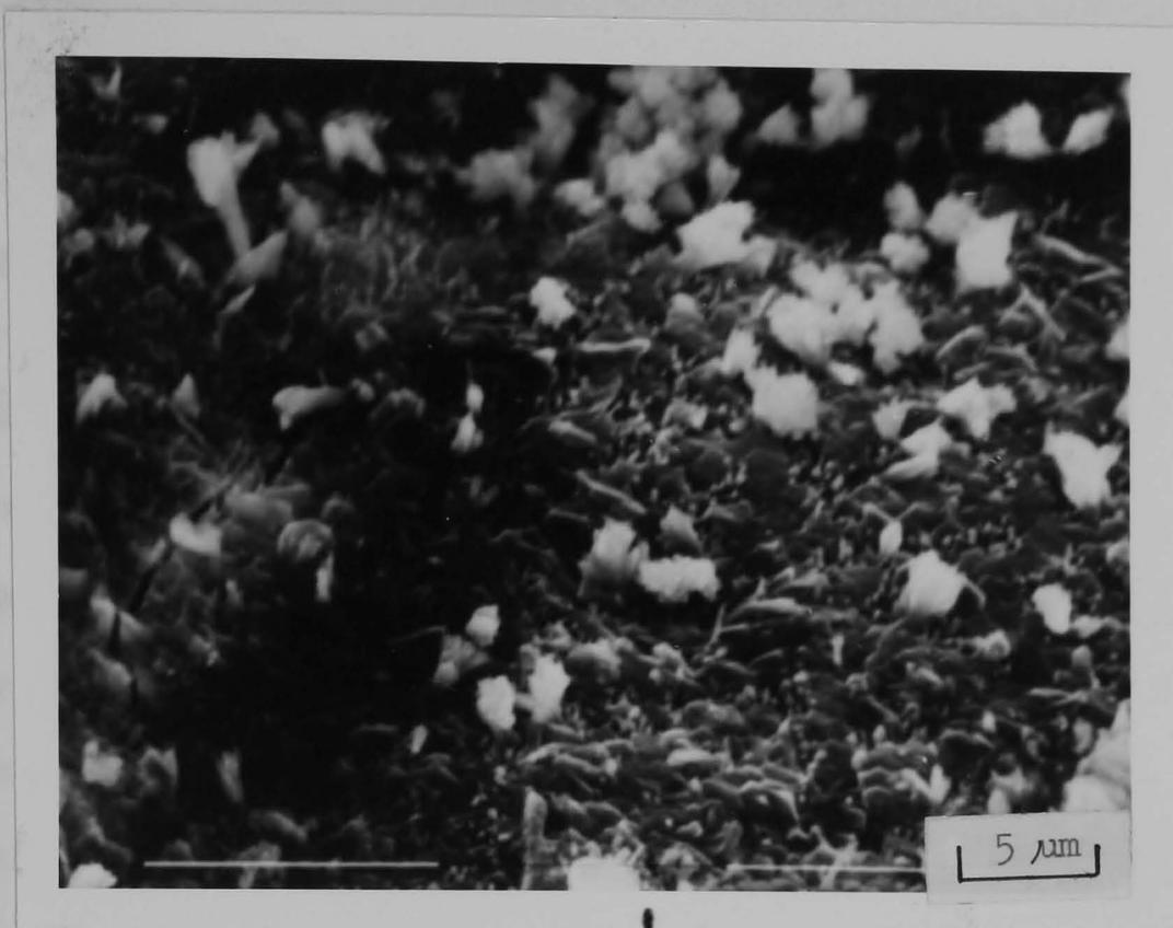
Fig. 6.25 SEM micrograph of a paste specimen (W/C = 0.4) initially cured for 1 day and subjected to 72 wet/dry cycles in 4% salt solution (Mag. 2500)
