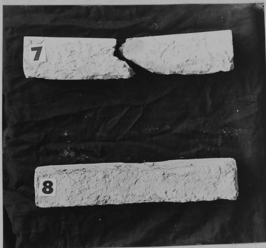
Fig. 9.8 Effect of freeze/thaw cycles on 1 day cured paste specimens ( $W/C = 0.3$ ) in saturated solution of sodium chloride after (7) 72 and (8) 18 cycles.
