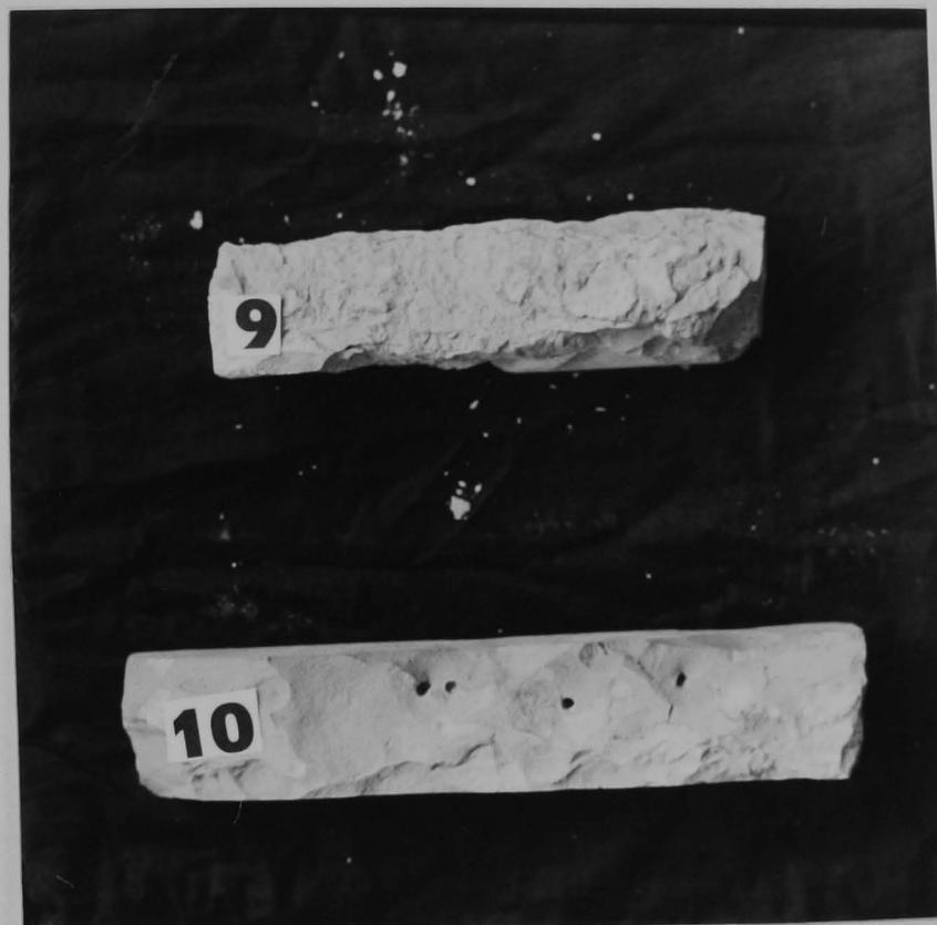
Fig. 9.7 Effect of freeze/thaw cycles on 1 day cured paste specimens ( $W/C = 0.3$ ) in 4% solution of sodium chloride after (9) 72 and (10) 18 cycles
