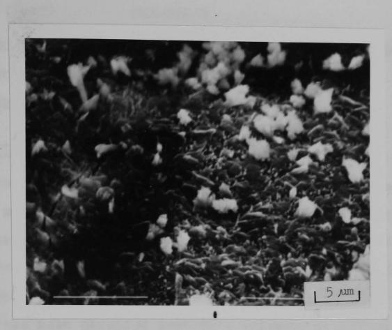
. Fig. 6.25 SEM micrograph of a paste specimen (W/C = 0.4) initially cured for 1 day and subjected to 72 wet/dry cycles in 4% salt solution (Mag. 2500)
