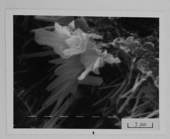
Fig. 6.17 SEM micrograph of paste specimen (W/C = 0.4) cured normally for 3 days and subjected to 36 freeze/thaw cycles in saturated solution of sodium chloride (Mag. 5000)
