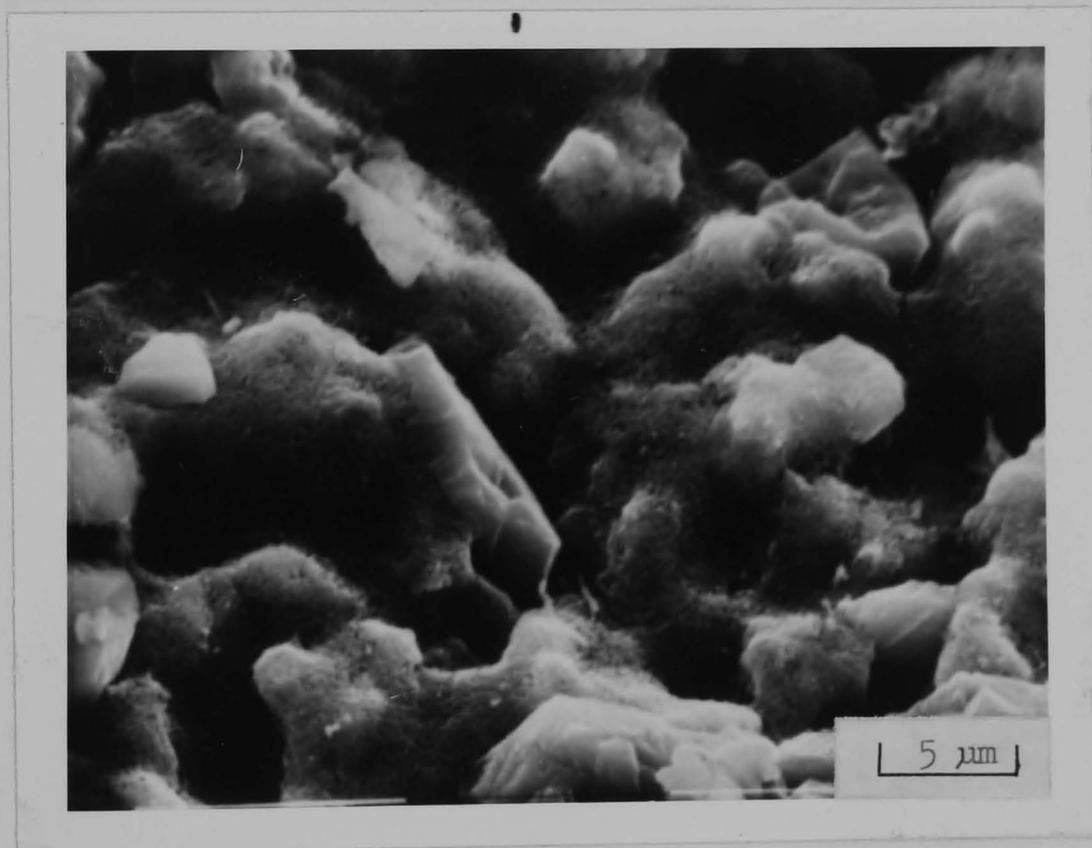
Fig. 6.24 SEM micrograph of a paste specimen (W/C = 0.4) initially cured for 1 day and subjected to 72 wet/dry cycles in 0% salt solution (Mag. 2500)
