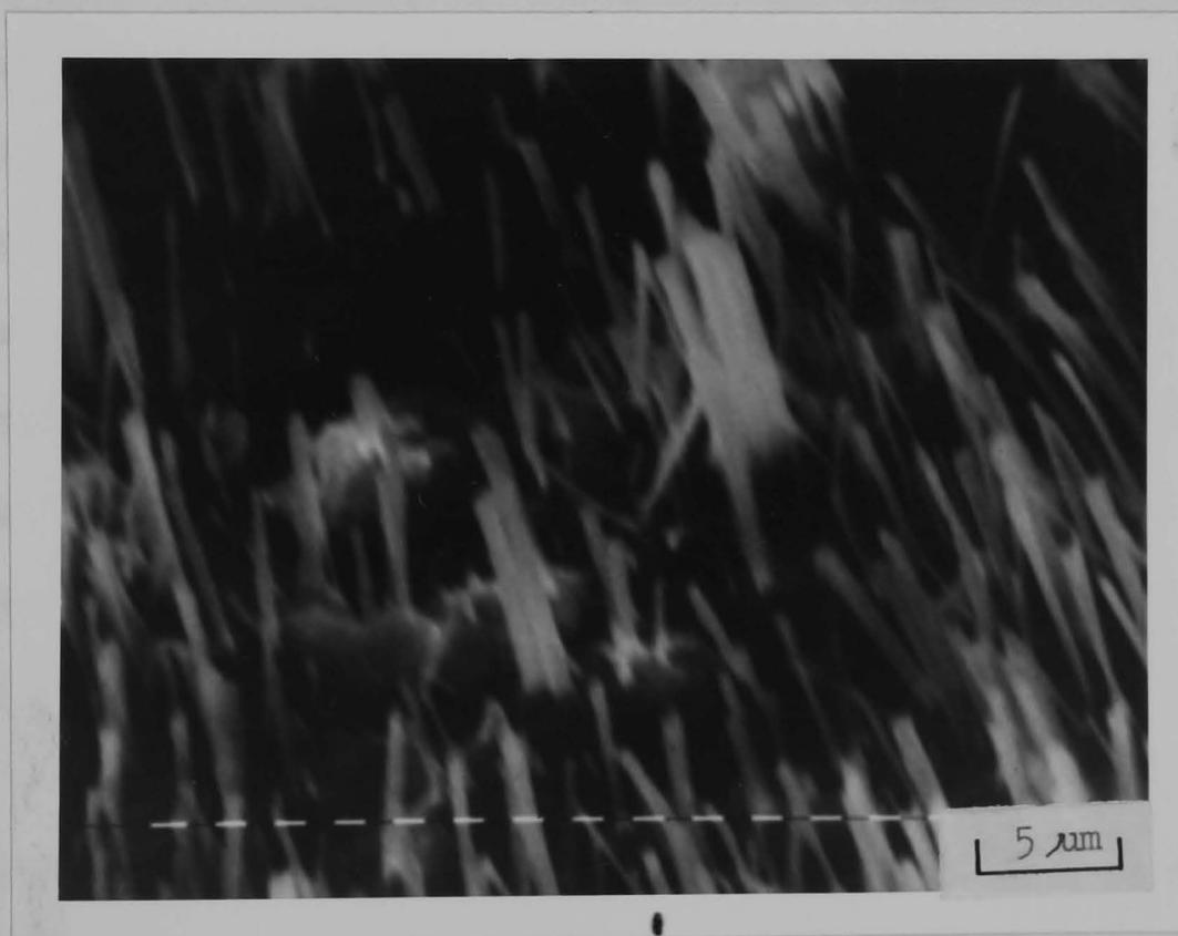
Fig. 6.26 SEM micrograph of a paste specimen (W/C = 0.4) initially cured for 1 day and subjected to 72 wet/dry cycles in saturated solution of sodium chloride (Mag. 2500)
