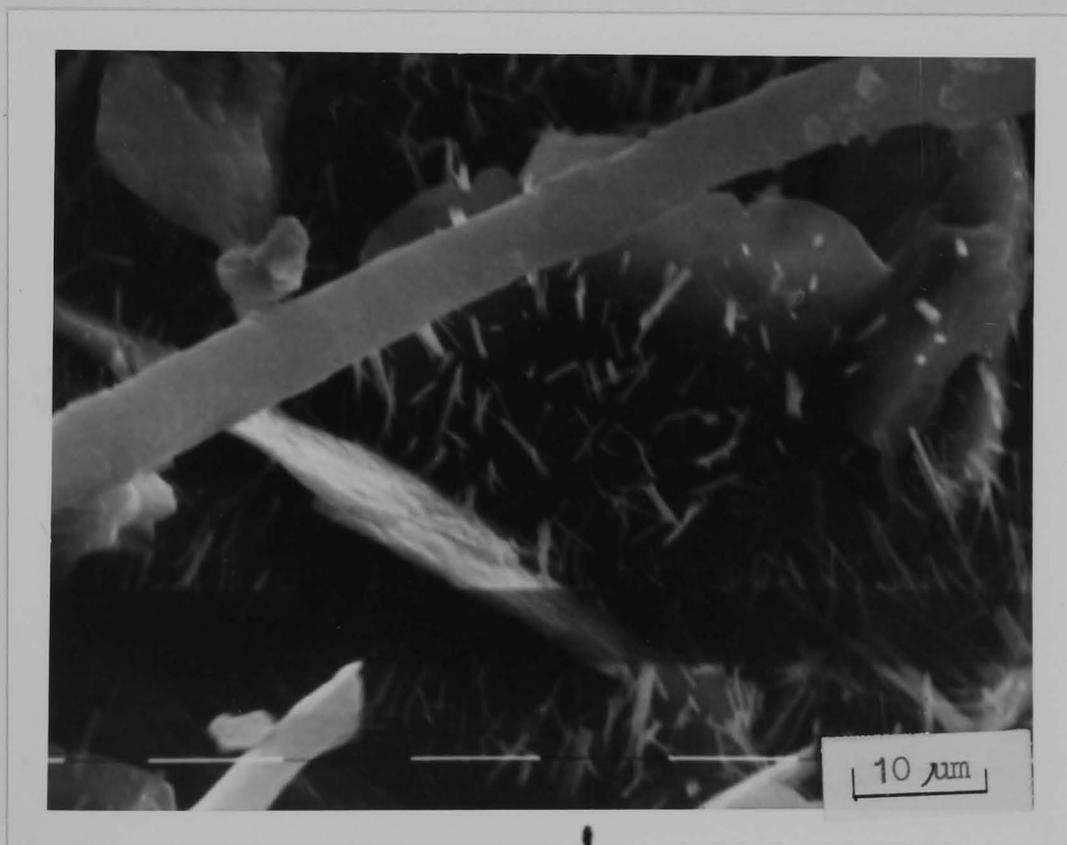
Fig. 6.14 SEM micrograph of a paste specimen (W/C = 0.4) cured normally for 3 days and subjected to 72 freeze/thaw cycles in 4% salt solution (Mag.1250)
