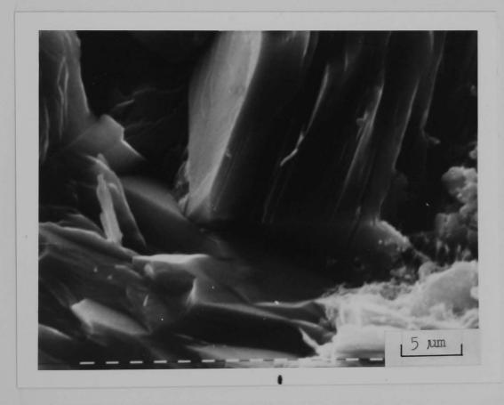
.Fig. 6.6 SEM micrograph of a specimen of cement paste (W/C = 0.3) cured normally for 28 days (Mag. 2500)
