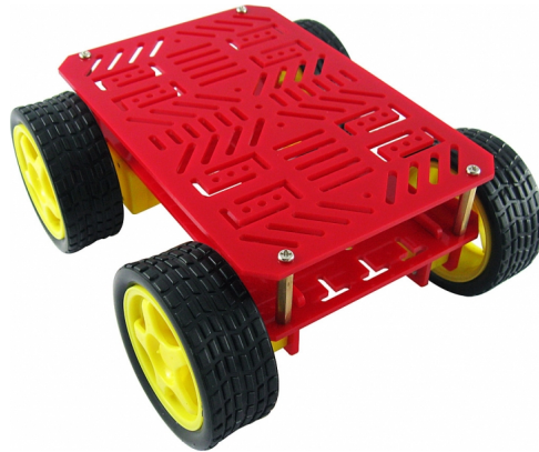
Figure 1.2: A simple wheeled robot model. Robot is constrained to move in the direction of the front wheels (Image Credit: yourduino.com).
