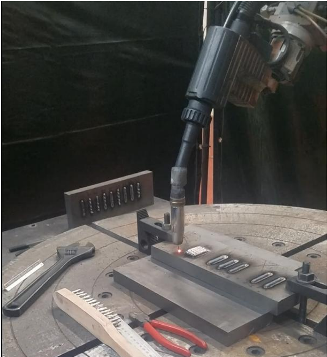
Figure 3-1 An additive manufacturing and robotic welding cell in operation.
