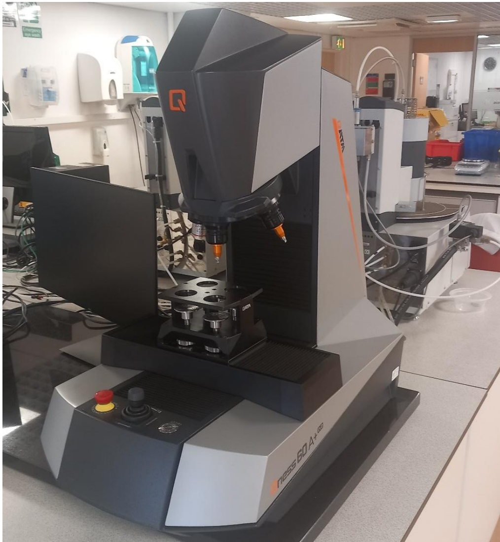
Figure 3-5 Qness 60A+ automated hardness tester.
