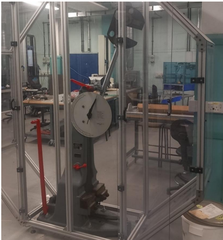
Figure 3-9 Losenhausenwerk 14590 Charpy impact apparatus with sample capturing enclosure.
