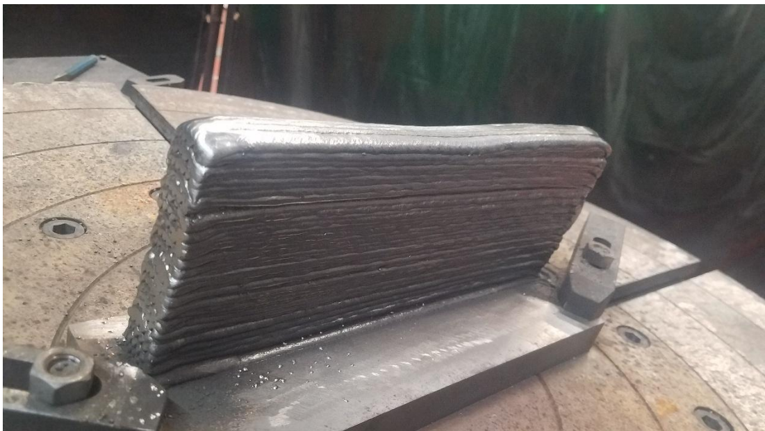
Figure 3-7 A completed example of a deposited wall.
