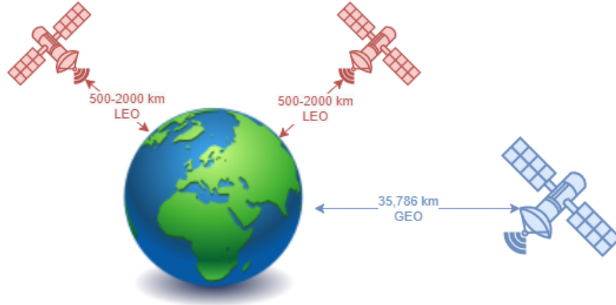
Figure 2.11: High level representation of LEO and GEO satellite deployments.
