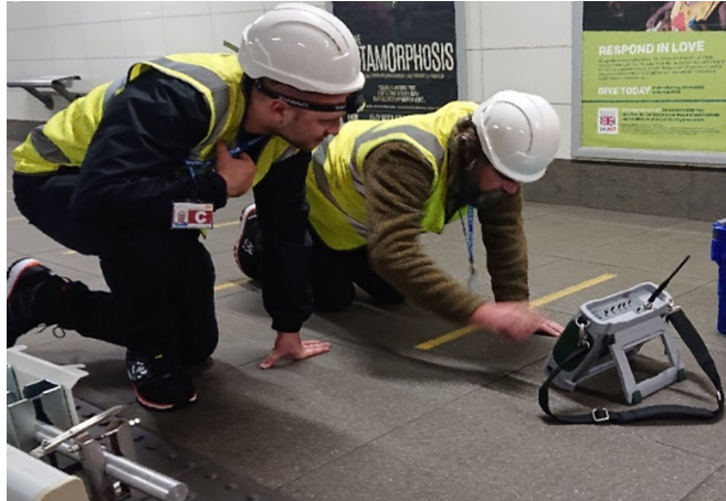
Figure 6.19: StrathSDR Engineers completing the RF Survey for 5GRN using the Field Master spectrum analyser.
