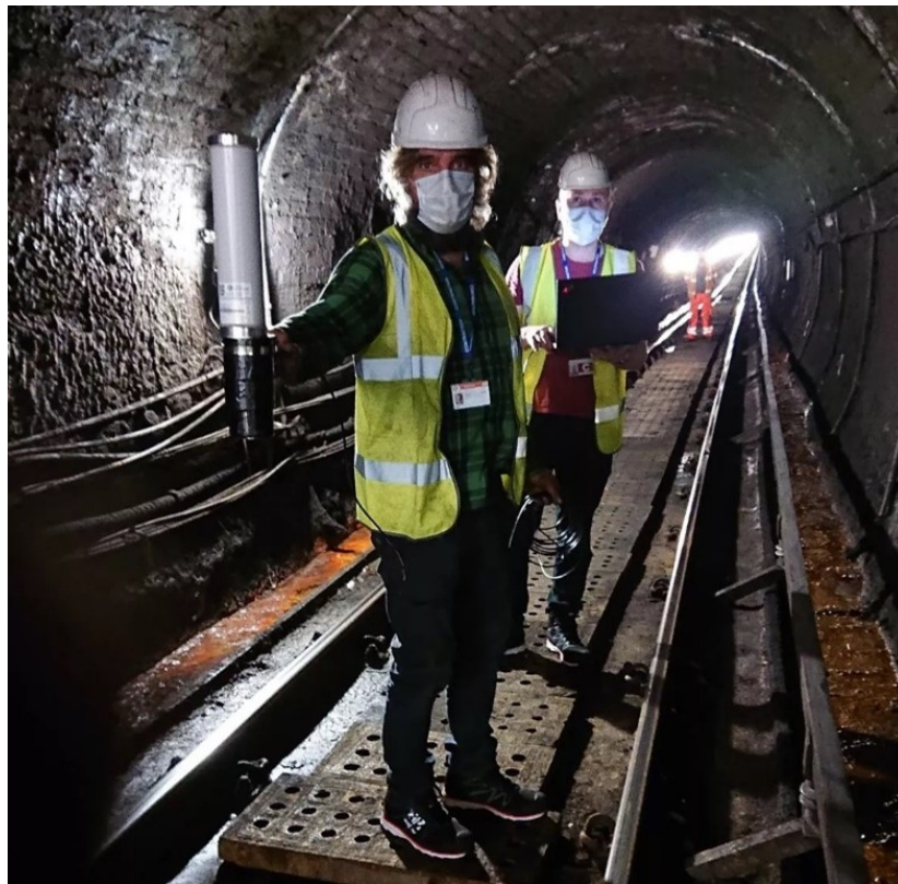
Figure 6.23: StrathSDR engineers completing RSRP measurements in the tunnel between Buchanan Street and St. Enoch Subway Stations.
