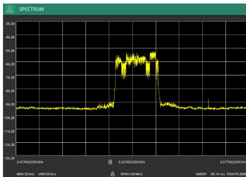
Figure 6.24: Spectrum Analyser response showing active spectral utilisation in the Glasgow Subway.
