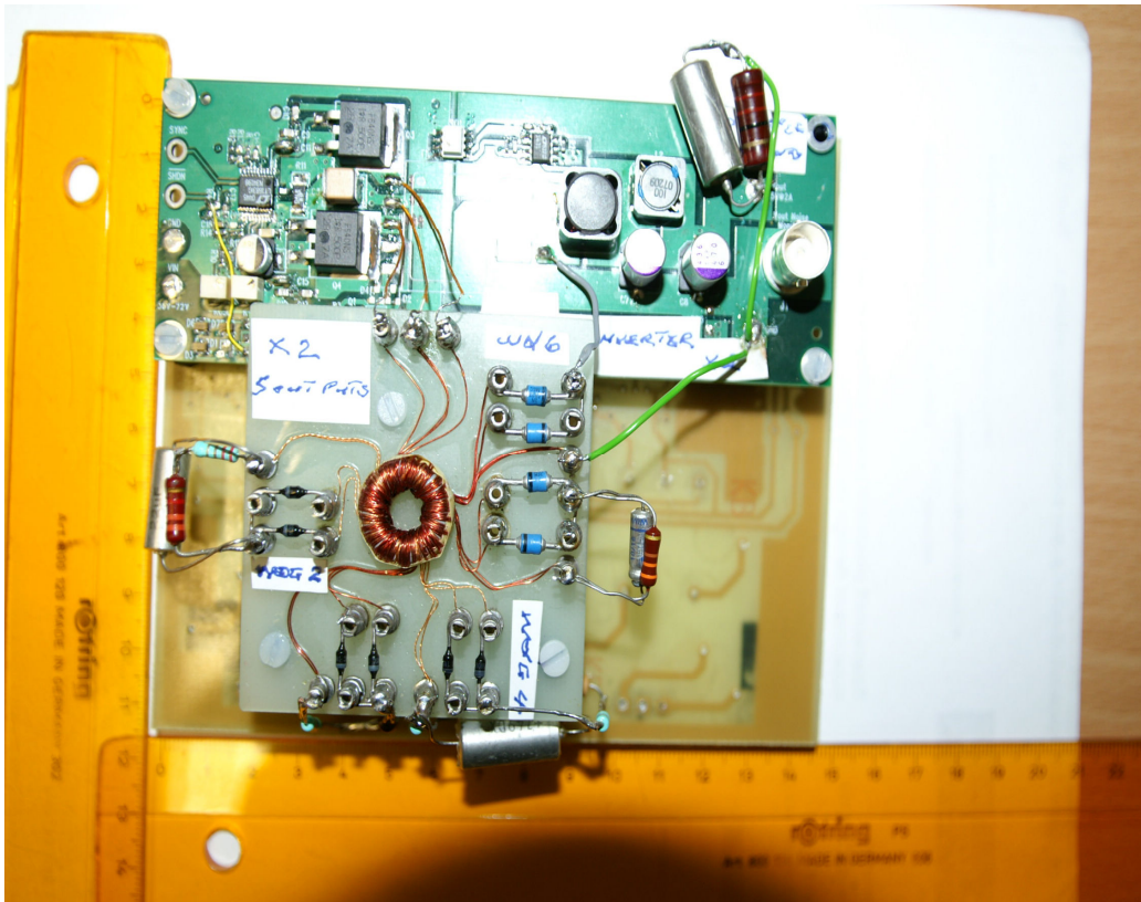
Figure C.5 The Aerostanrew mod1 toroid transformer rectifier board is using the space-qualified Schottky full wave rectifiers and ultra fast switching diodes. This includes all load capacitors and load resistors attached to the (X2) PCB.
