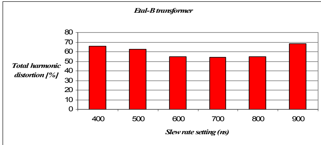
Figure 4.5 Total harmonic distortion as a percentage versus the voltage slew rate setting. These measurements were taken from the Etal-B transformer rectifier board.
