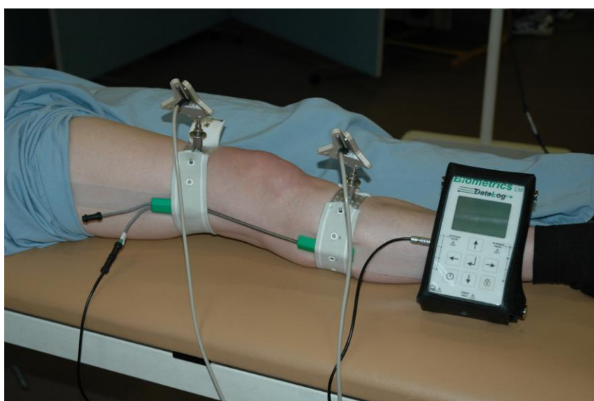
Figure 2.14 Photo of the setup for the validation between the electrogoniometer and the navigation system.
