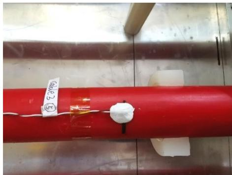
**Figure 19.** Example of temperature sensor fixed on the cable surface
