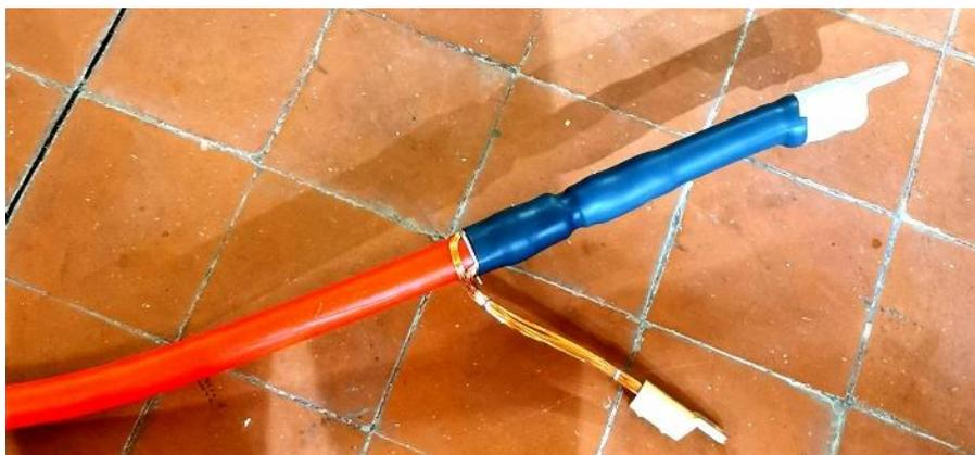
**Figure 10.** Whole scale of cable specimen with prepared terminals
