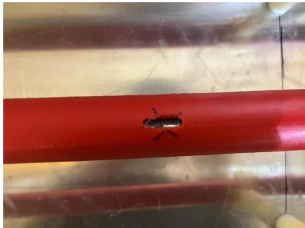
**Figure 22.** Demonstration of a hole on the dummy cable
