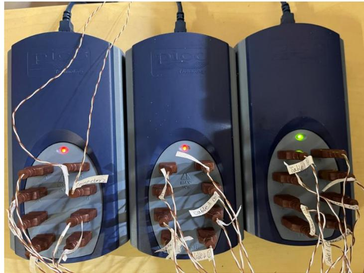
**Figure 20.** TC-08 thermocouple data logger
