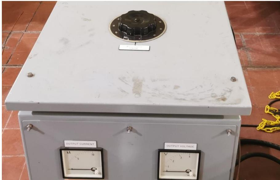
**Figure 15.** The current transformer as experiment power supply
