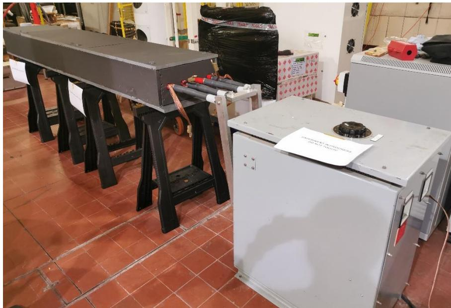
**Figure 14.** Practical cables accelerated thermal ageing experiment platform
