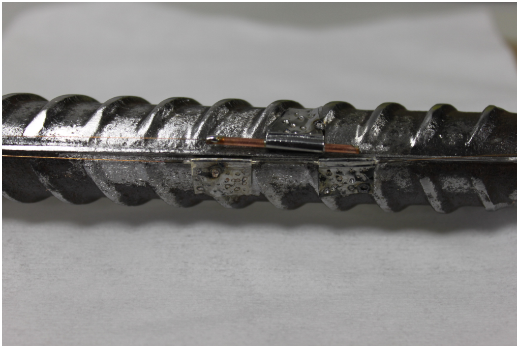
(b) Non Pre-Stressed Strain Sensor & Brazed Capillary with Soldered Copper Tube and Shim
