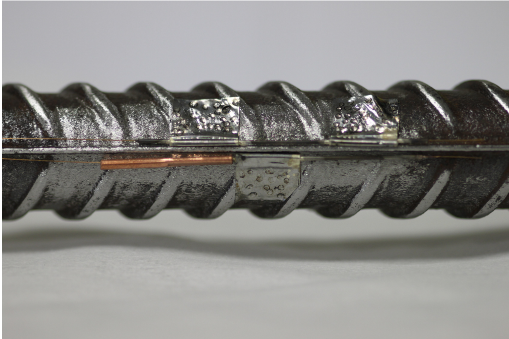
(a) Pre-Stressed Strain Sensor & Brazed Capillary and Shim
