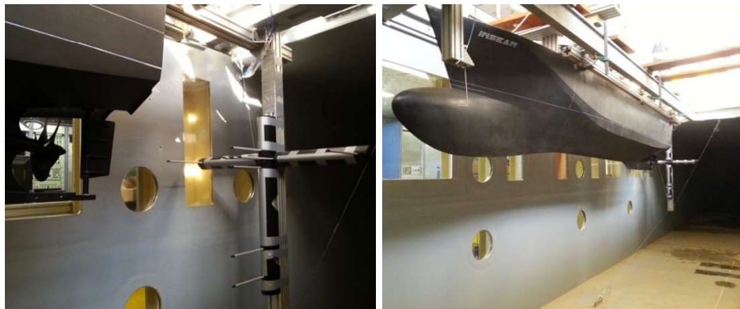
Figure 7-4 Cavitation observations: set up arrangement
