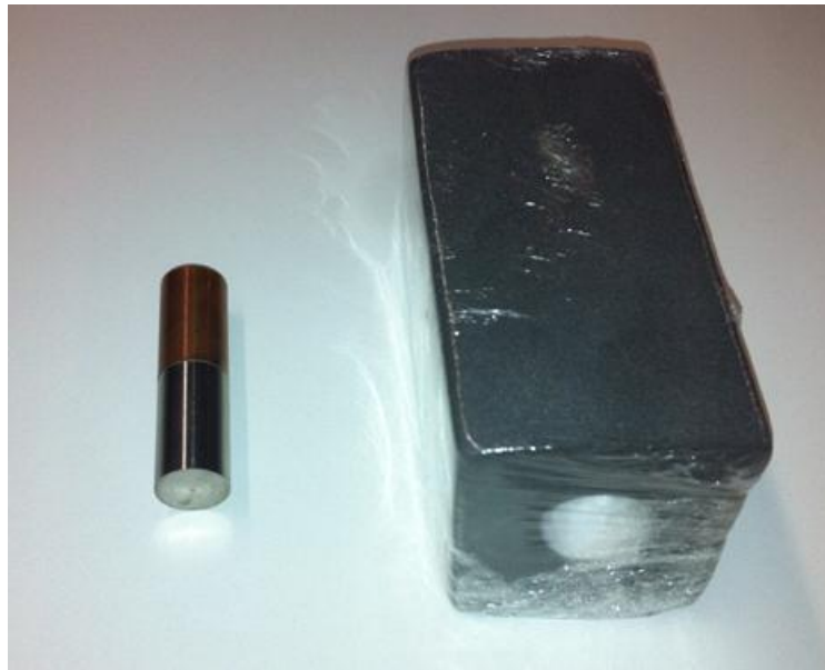
Figure 5-5 - Insulated sample for thermal autofrettage to -196^{\circ}\text{C} in liquid nitrogen
