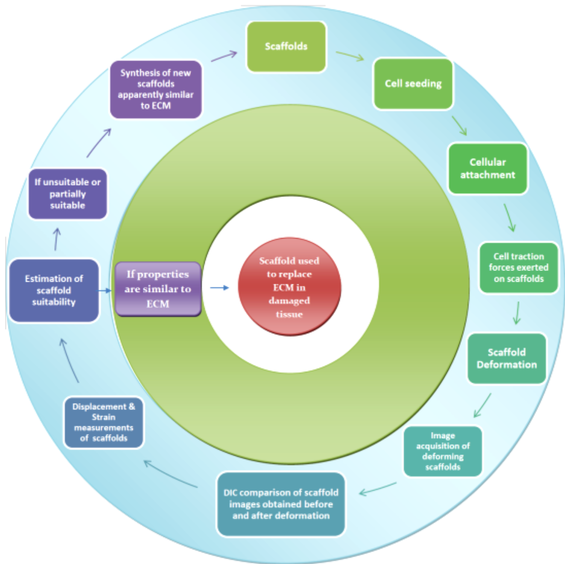
Figure 3-21 Process of scaffold evaluation using digital image correlation
