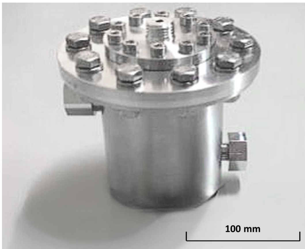
Figure 6.7 Assembly of the designed nozzle
