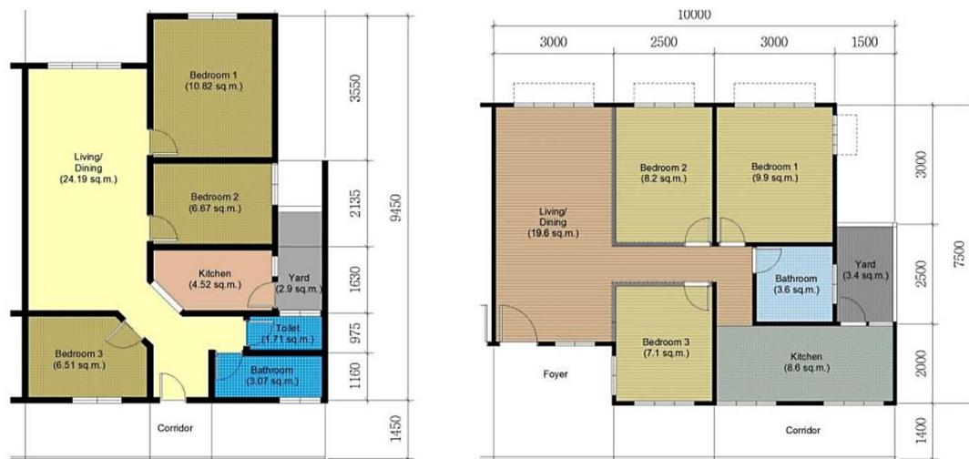
Figure 2.21: The unit plan layouts for the PPR first-generation (left) and the new proposal made in 2012 (right) (Mohd Sahabuddin, 2012)
