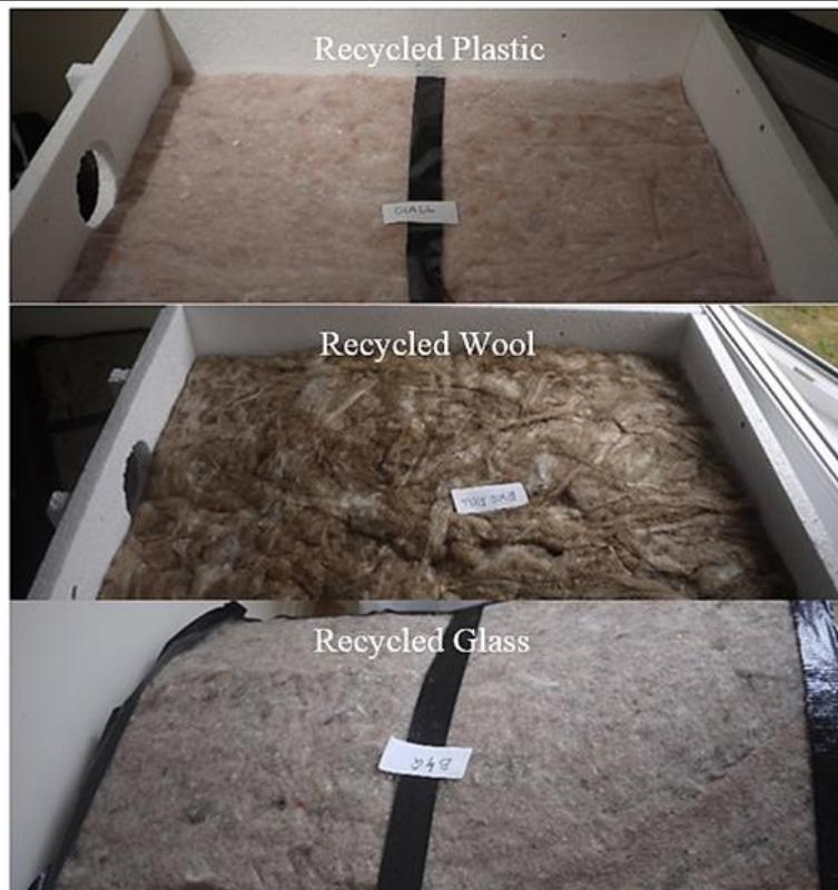
*Figure 4.7: The recycled insulations used in Test 2*
