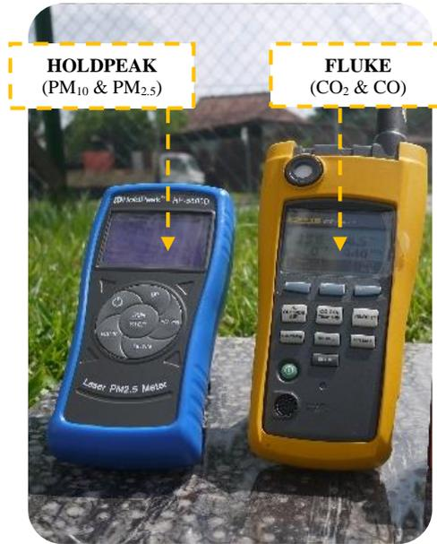
Figure 3.5: The air quality instrument
