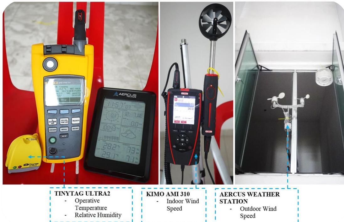
Figure 3.4: The thermal comfort instrument
