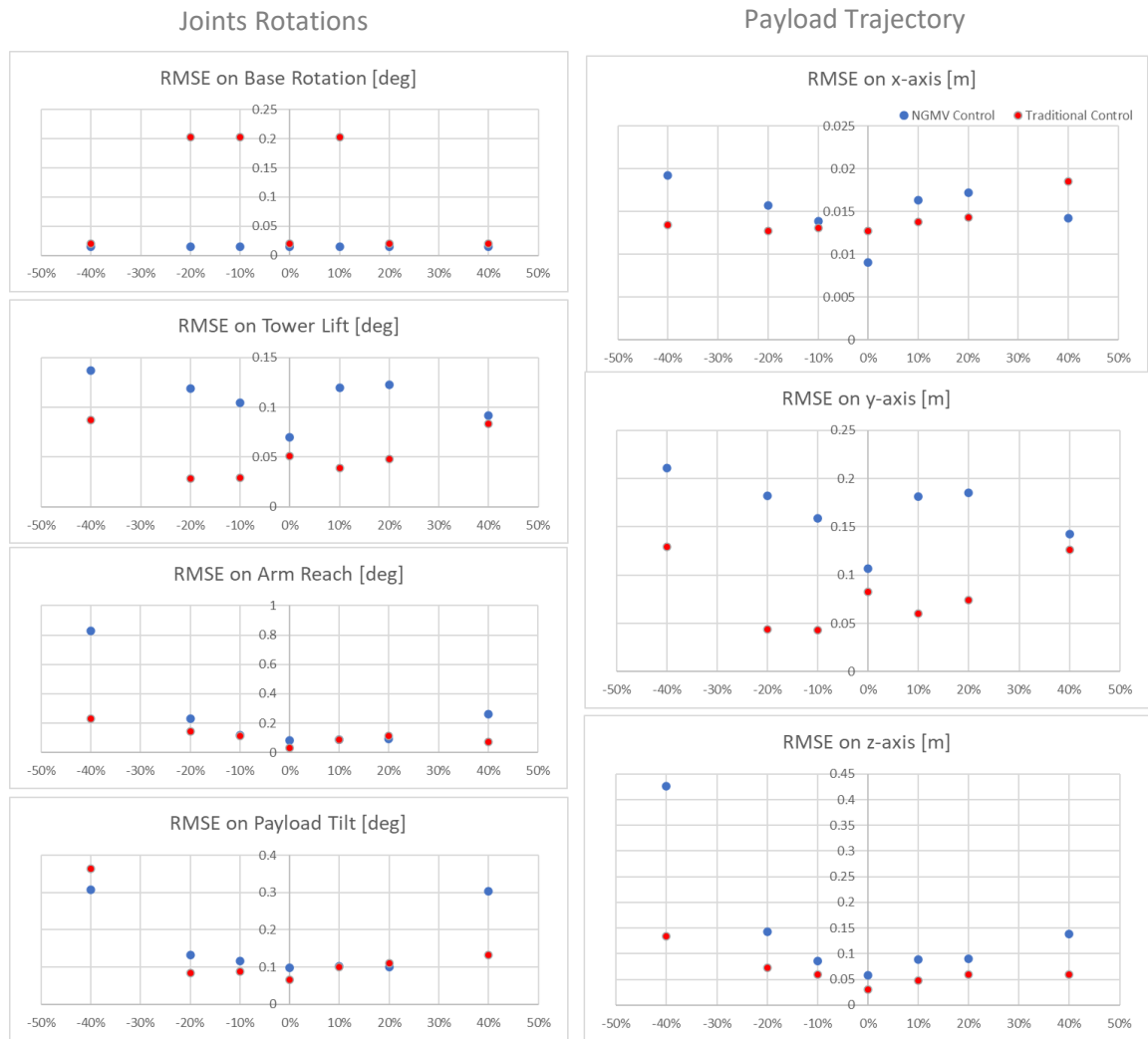
Figure 4.25: Plotted root mean square errors for joints rotations and resulting payload trajectory on x-y-z across 0%, 10%, 20% and 40% mismatch levels
