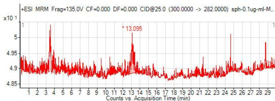
Figure 6.14 MRM trace obtained for sphingosine at 0.1 ng/ml monitoring the transition from m/z 300 to m/z 282 with 25 V collision energy using a silica gel column.
