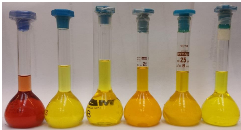
Figure 2.15 1mM solutions of mononuclear ruthenium picolinic acid complexes Left to right: trispicolinate, bispicolinate, (2,3) , (2,4) , (2,5) , (2,6).
