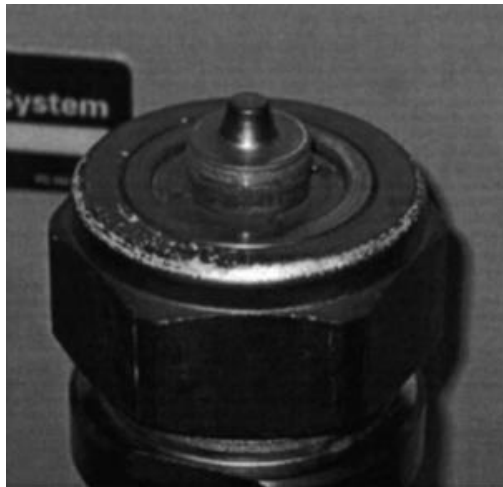
Figure 2.1: Tungsten alloy tool used by Reynolds et al. [2.14].
