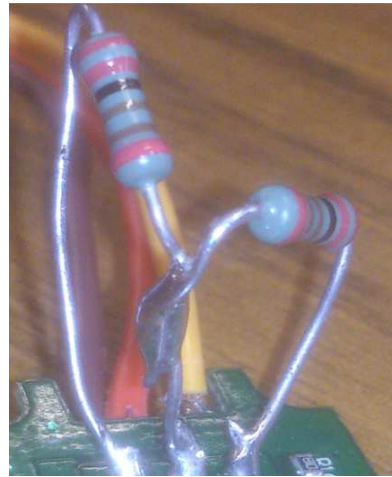
Figure 32 Replacing resistors structure
