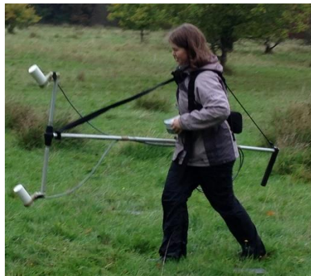
Figure 5.5: The G-858 MagMapper Magnetometer in use as a gradiometer.
