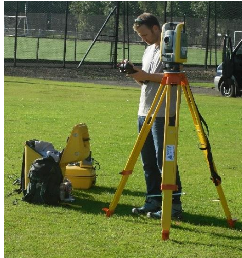
Figure 5.25: A photograph showing the Trimble S6 Total Station used in the field trial.
