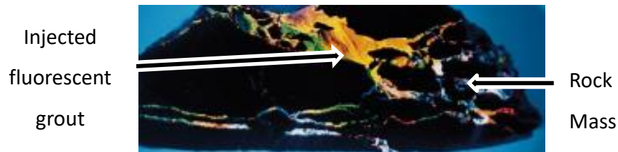
Figure 2.12: A cored sample showing injected grout containing a fluorescent substance (After Chen et al. , 2000).
