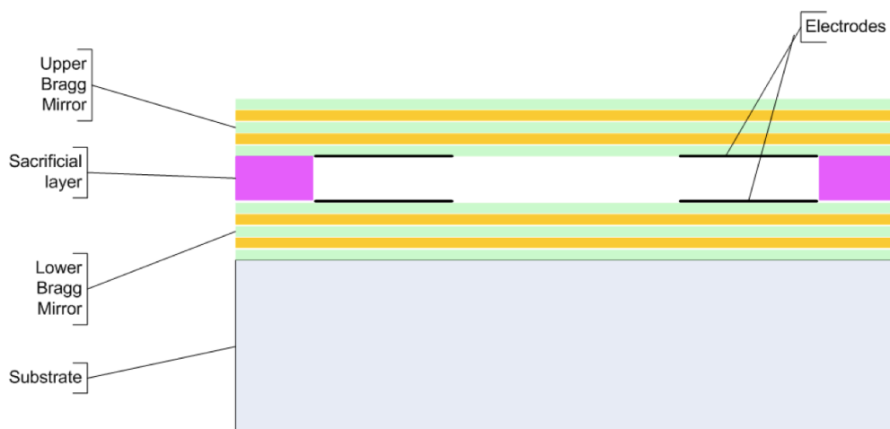
Figure 1.3 - MEMS Fabry-Pérot interferometer, taken from reference 109.
