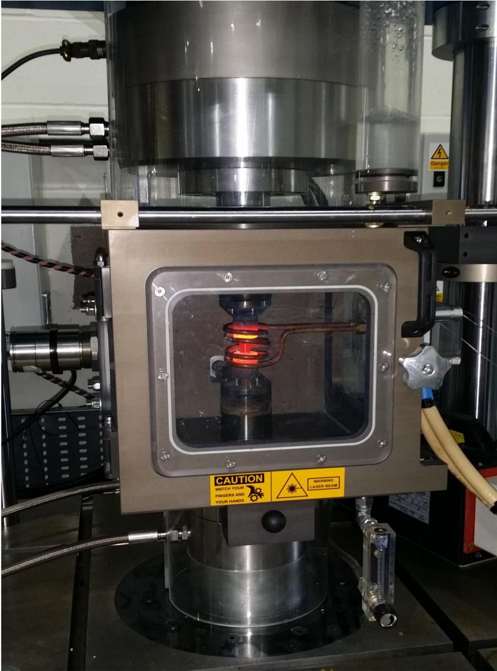
Figure B.3: Sample during heating inside Phoenix tester before compression
