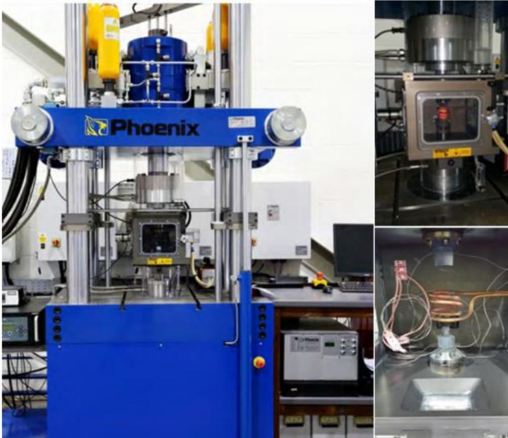
**Figure 3.1:** Servo-hydraulic forging simulation a) machine, b) chamber and c) interior
