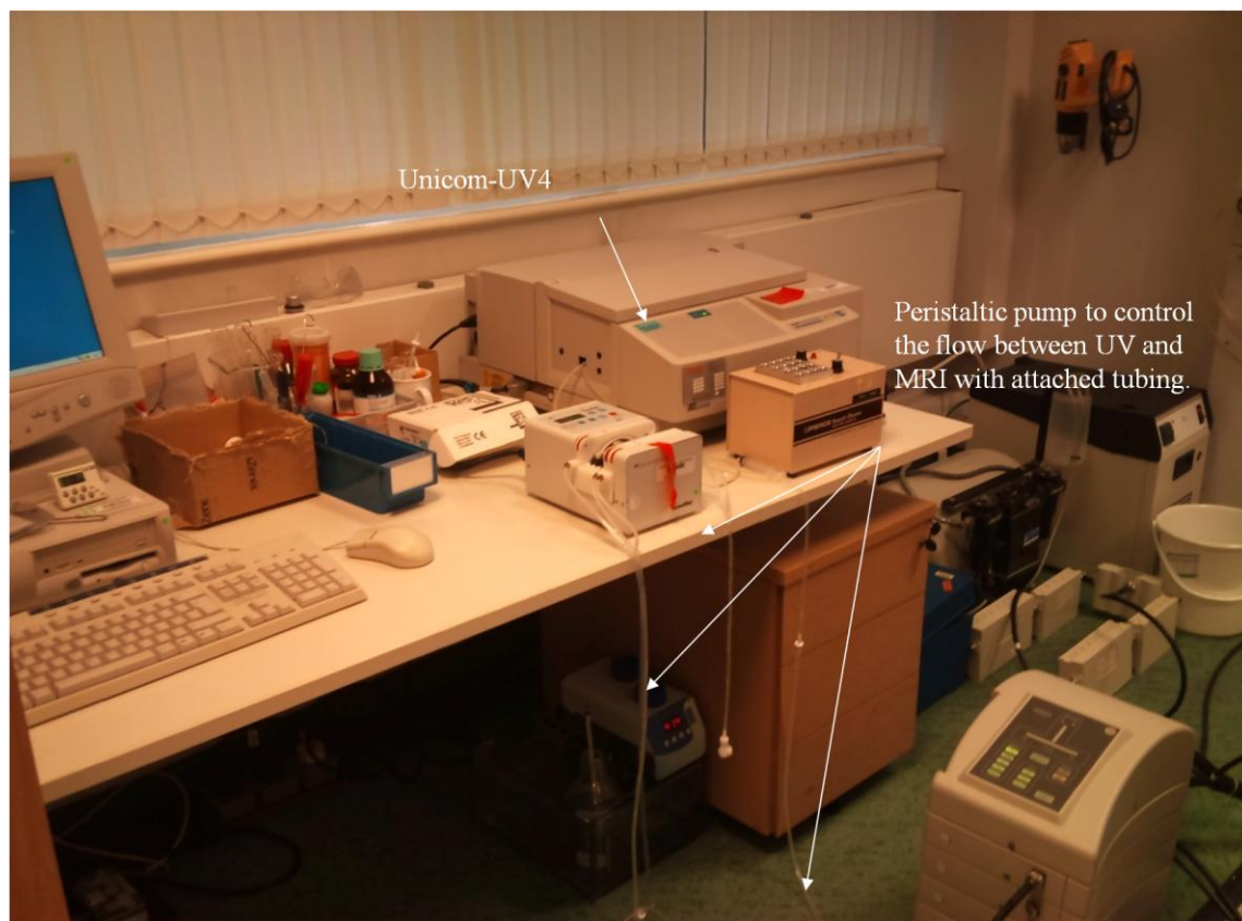
Figure 6.7 The Unicom-UV4 spectrometer attached to peristaltic pump and USP 4 type dissolution apparatus through connected plastic tubing for UV data acquisition.
