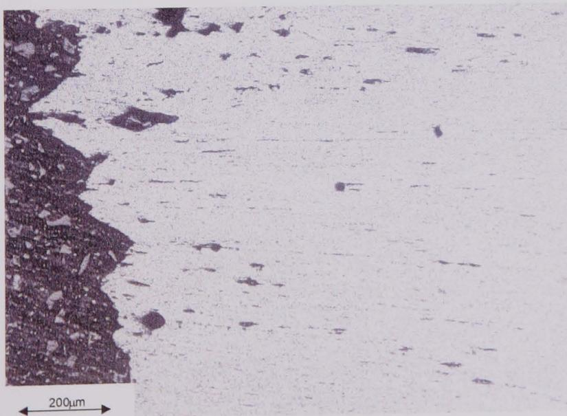
Figure 7.12 Cross section of Alloy C3(1) stress rupture failure
