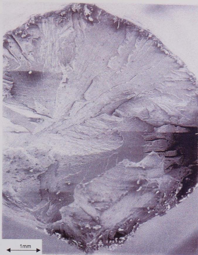
*Figure 9.6a Fracture surface of room temperature tensile test*
