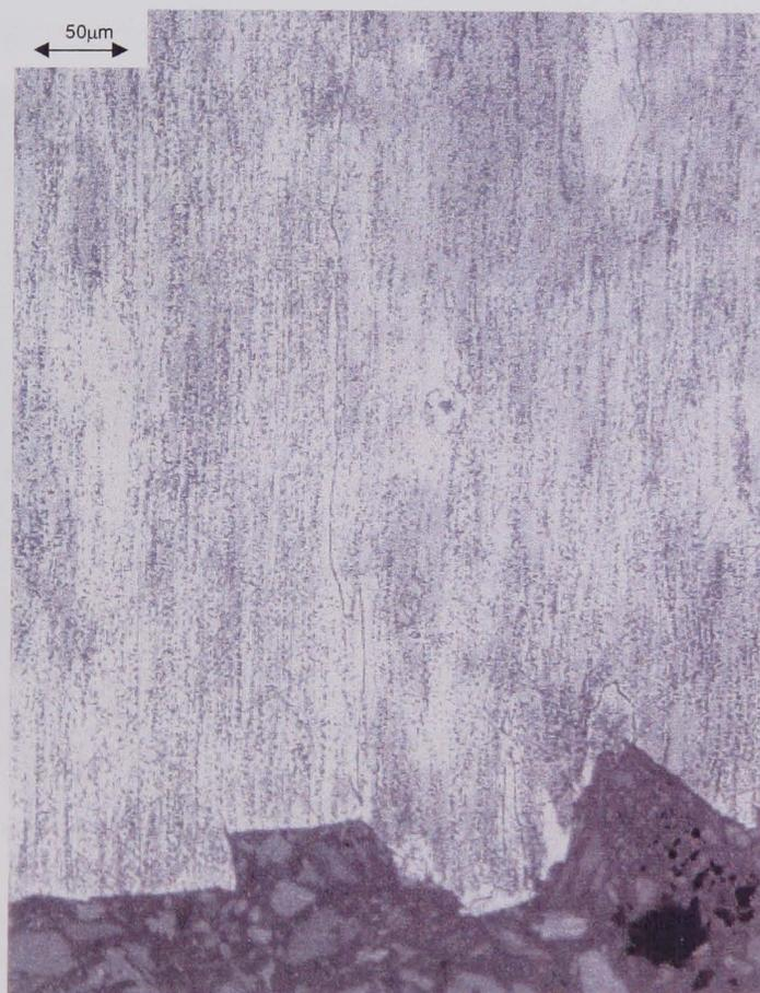
*Figure 9.6b Cross section of room temperature fracture surface*
