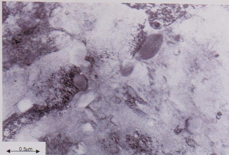
*Figure 7.4a Area of coarse particles in Alloy D*
