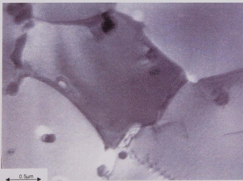
*Figure 7.5 Area of coarse particles in Alloy C3(1)*
