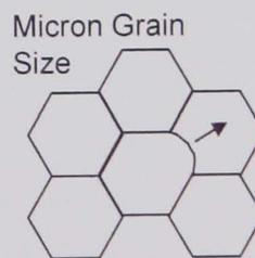
Grain boundary junctions provide pinning points for small grains.
