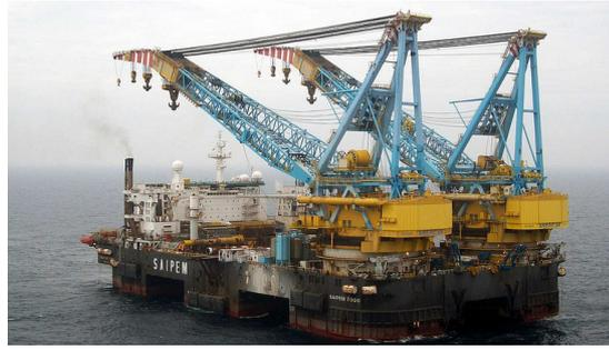
Figure 22: Semi-submersible crane vessel (Saipem S.p.A., 2012)
