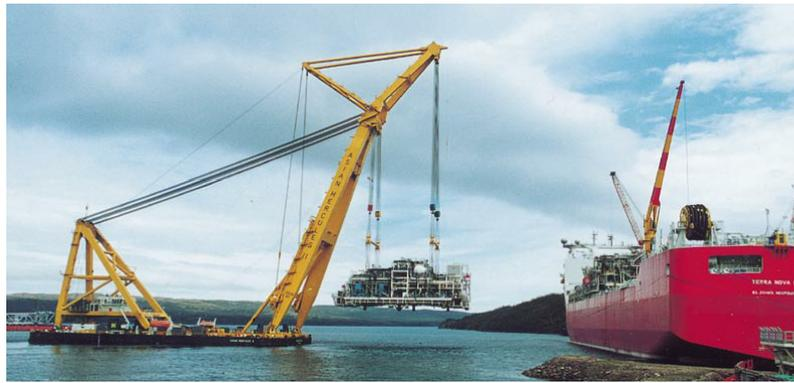
Figure 20: Sheer-leg heavy-lift crane barge (SMIT Heavy Lift Europe, 2012)
