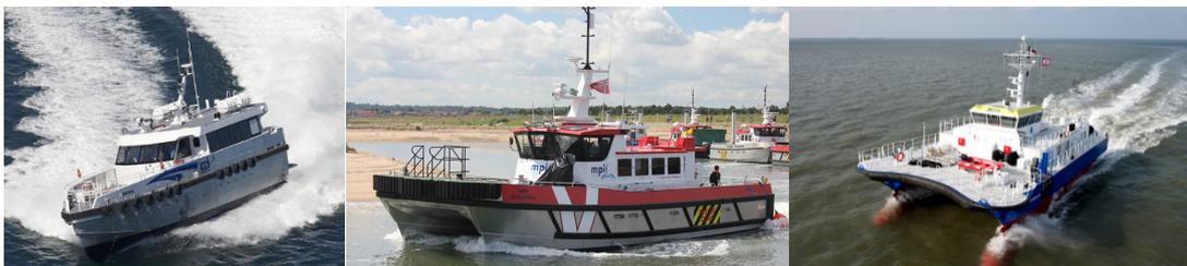
Figure 15: Vessel for minor maintenance operations (Monohull – Catamaran - SWATH) (MPI Offshore, 2012, BARD Group, 2013, Incat Crowther, 2013)
