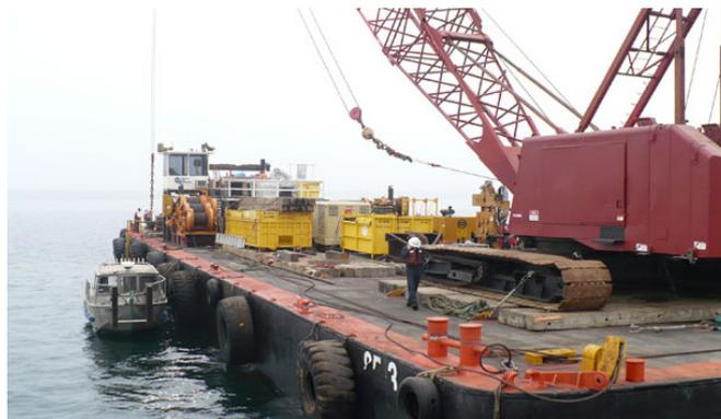
Figure 21: Heavy-lift crane barge with mobile crane (Turn Key Maritime Solutions, 2012)
