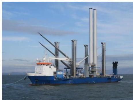
Figure 18: Leg-stabilised vessel (A2SEA, 2012a)
