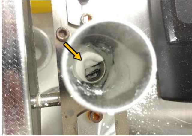
Figure 4.8 Material build-up at powder inlet due to screws becoming flooded in the nucleation setup.
