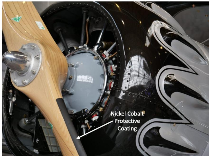
Figure 12.1: Nickel Cobalt coating on an aeroplane propeller to protect it against LEE. Source [224]
