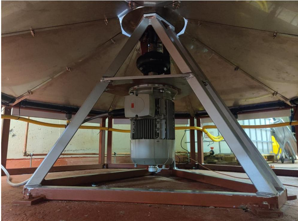
Figure 5.3: Motor stand frame under the main octagon of the WARER.
