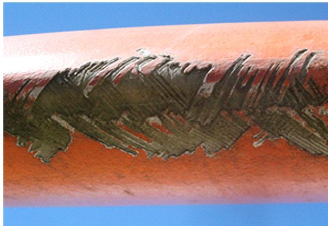
Figure 10.1: Severe leading edge erosion of a turbine blade. Source [52]
