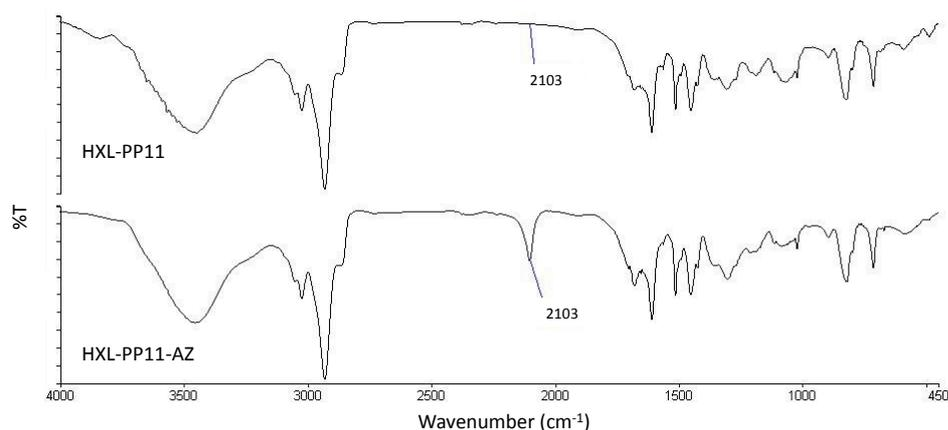
**Figure 4.3.9.2. – FT-IR spectra of the hypercrosslinked polymer HXL-PP11 and the corresponding azide-modified hypercrosslinked material HXL-PP11-Az.**
