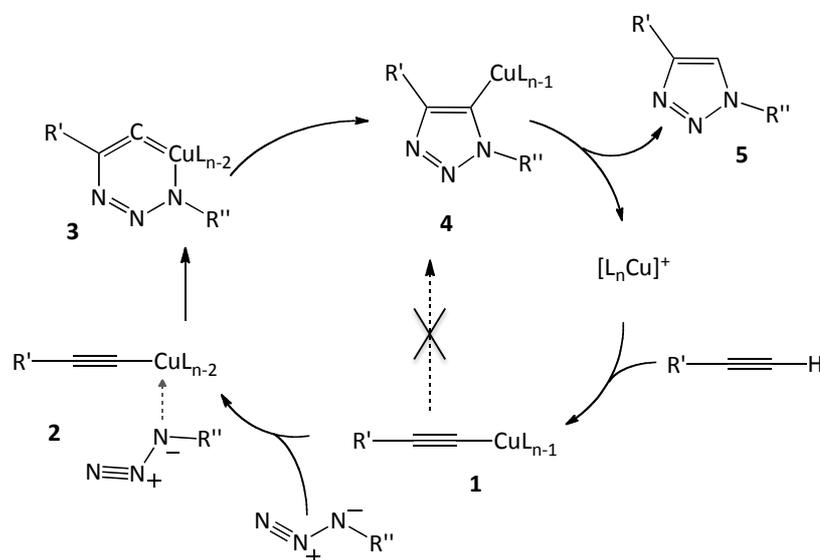
**Figure 4.1.3.1.1. – Mechanism proposed by Sharpless for copper(I) catalysed azide-alkyne cycloaddition.**<sup>13</sup>
