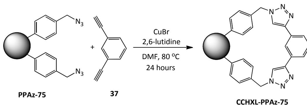
Figure 4.3.10.2.1. - Click-based hypercrosslinking reaction of PPAz-75.
