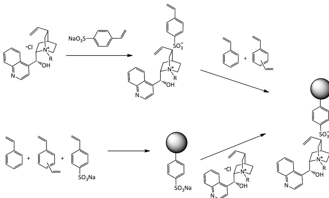
**Figure 2.1.2.1. – Synthesis of polymer-supported chiral catalyst (side chain).<sup>14</sup>**
