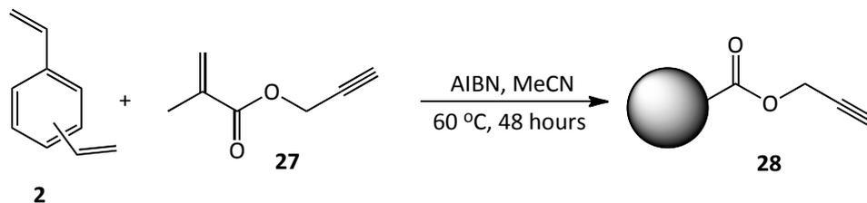
**Figure 4.1.6.2.3. - Preparation of alkyne-containing polymer microspheres by precipitation polymerisation.**
