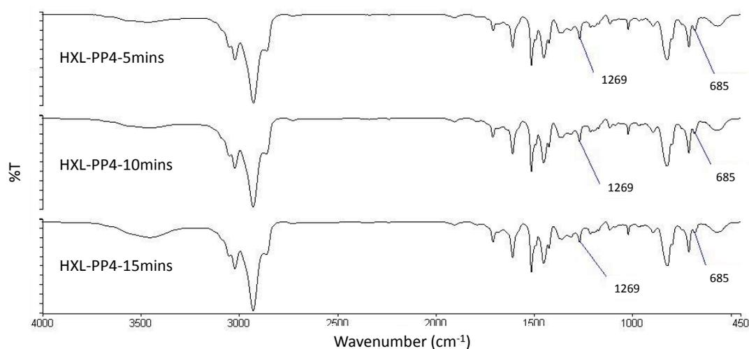
**Figure 3.3.3.3. – FT-IR spectra for the hypercrosslinked products formed after 5, 10 and 15 minutes of reaction.**
