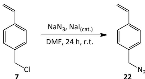
**Figure 4.3.1.1. – Conversion of VBC into VBAz.**
