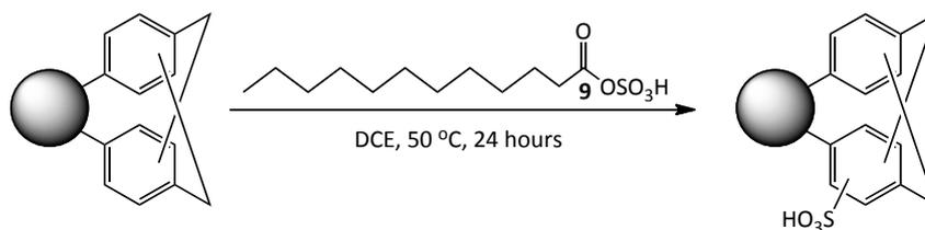
**Figure 2.3.3.1. – Sulfonation of hypercrosslinked particles using lauroyl sulfate.**
