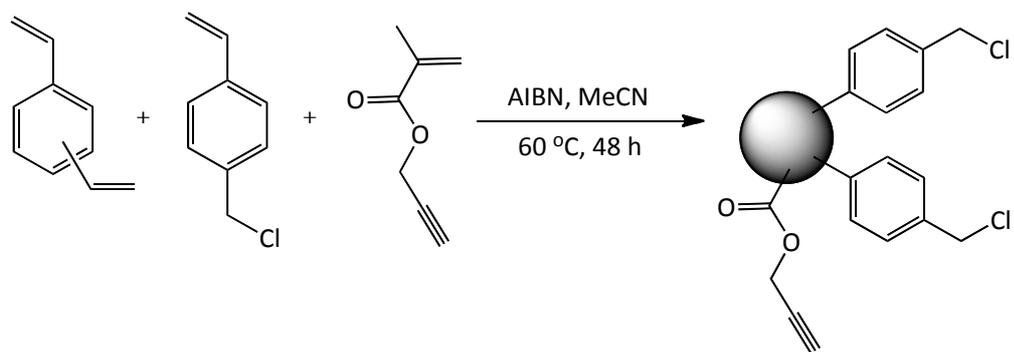
**Figure 4.3.5.2. – Synthesis of 25/70/5 (w/w/w) DVB/VBC/PMA polymer microspheres under precipitation polymerisation conditions.**
