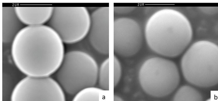
Figure 4.3.3.7. – SEM micrographs obtained for: (a) the azide-containing polymer PPAz-1, and (b) the product of its click reaction with propargyl alcohol, PPAz-CC7.
