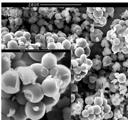
**Figure 4.3.5.4. – SEM images of poly(DVB-co-VBC-co-PMA) (PPAlk-1).**
