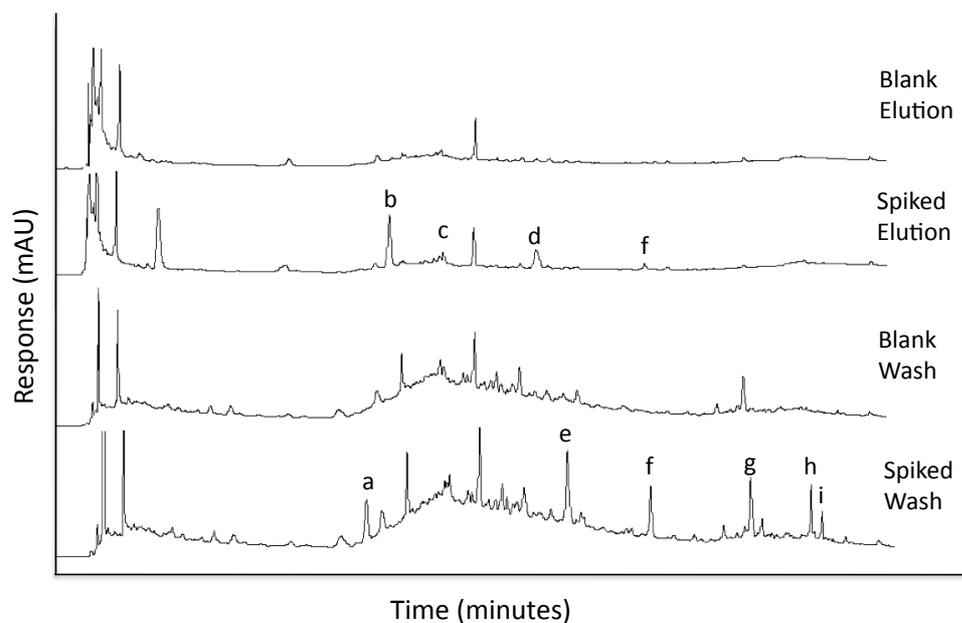
**Figure 2.3.7.3.2. - Chromatograms obtained for the washing and elution steps of 250 mL spiked (8 µg/L) and blank samples of WWTP effluent water percolated through the HXL-PP-SCXc sorbent: (a) caffeine, (b) trimethoprim, (c) antipyrine, (d) propranolol, (e) salicylic acid, (f) carbamazepine, (g) clofibric acid, (h) diclofenac and (i) ibuprofen.**
