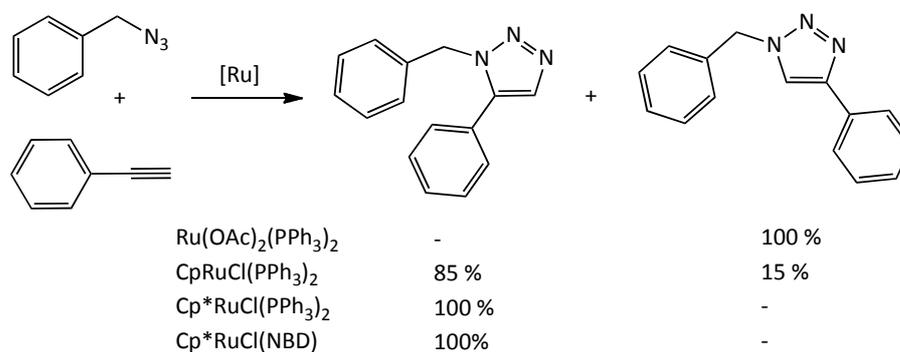
Figure 4.1.3.4.1. – Ru-catalysed cycloaddition of benzyl azide and phenylacetylene.<sup>22</sup>
