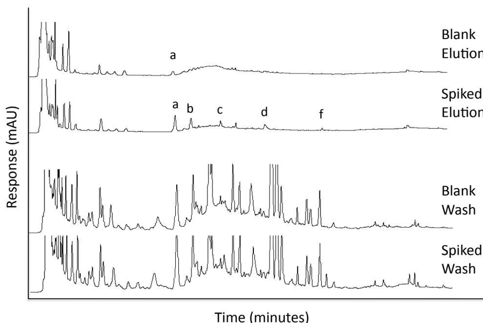
**Figure 2.3.7.3.3. - Chromatograms obtained for the washing and elution steps of 100 mL spiked (20 µg/L) and blank samples of WWTP influent water percolated through the HXL-PP-SCXc sorbent: (a) caffeine, (b) trimethoprim, (c) antipyrine, (d) propranolol and (f) carbamazepine.**
