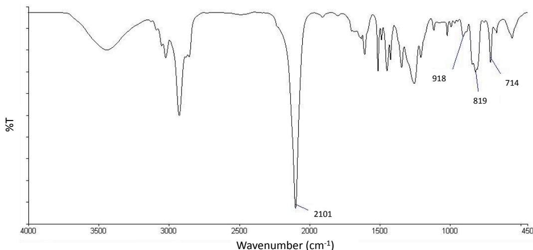
**Figure 4.3.10.1.2. - FT-IR spectrum for the copolymer prepared from a feed of 25/75 (w/w) DVB/VBAz (PPAz-75).**
