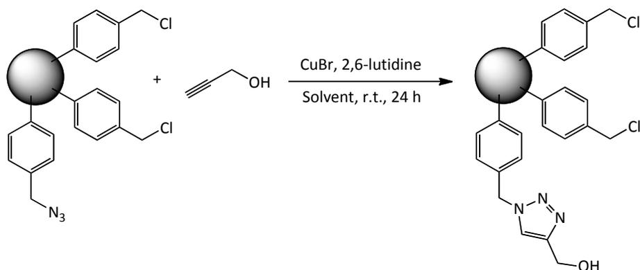
**Figure 4.3.3.1. – Click chemistry modification of the azide-containing polymers (PPAz-1, PPAz-2 and PPAz-3) with propargyl alcohol.**
