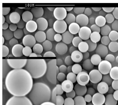
**Figure 4.3.1.4. – SEM micrographs for PPAz-1.**
