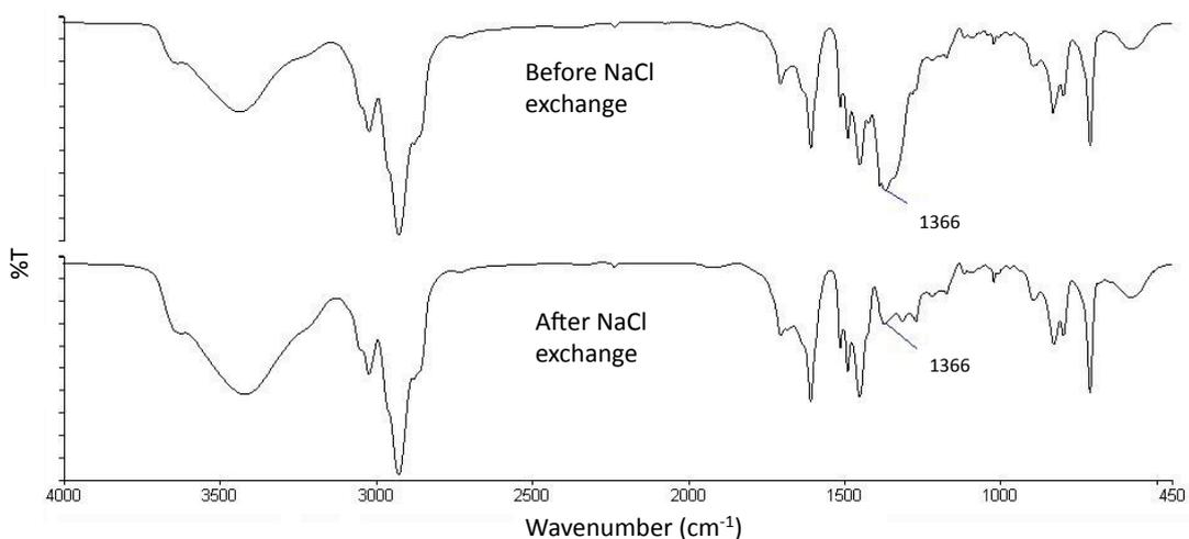
**Figure 3.3.5.2.3. – FT-IR spectra of HXL-PP8-AD\* before and after NaCl exchange.**
