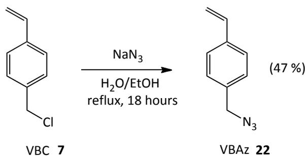
**Figure 4.1.6.1.1. – Reaction of VBC and sodium azide to yield VBAz.**
