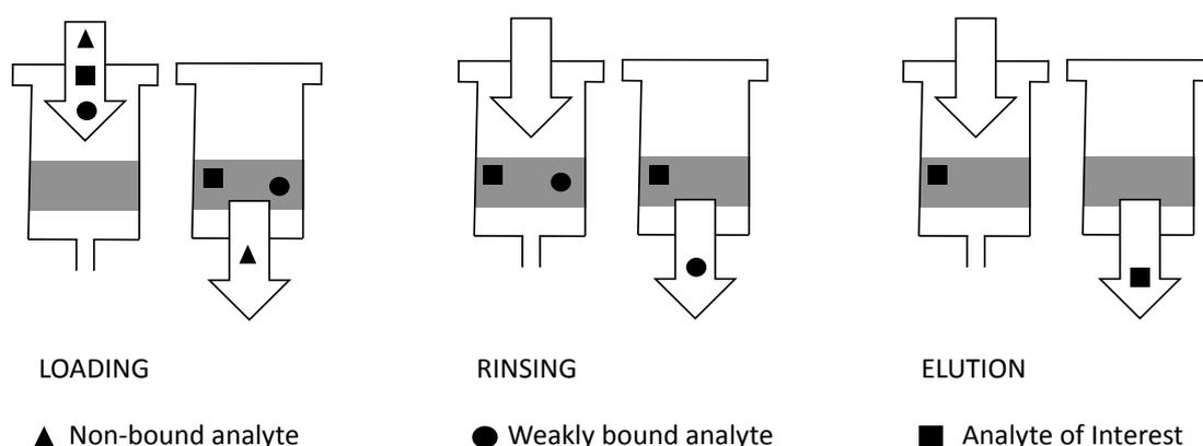
**Figure 2.1.4.3. - Loading, rinsing and elution steps of SPE.<sup>36</sup>**
