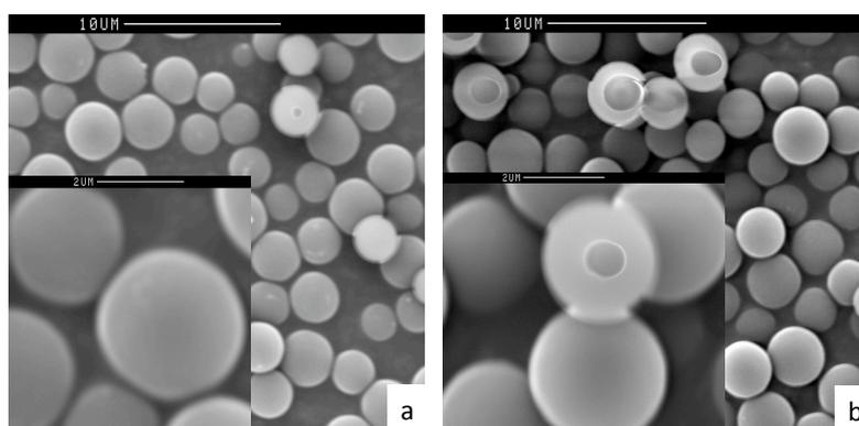
**Figure 4.3.4.2. – SEM micrographs obtained for hypercrosslinked functionalised polymers: (a) HXL-PPAz-CC4 (b) HXL-PPAz-CC7.**
