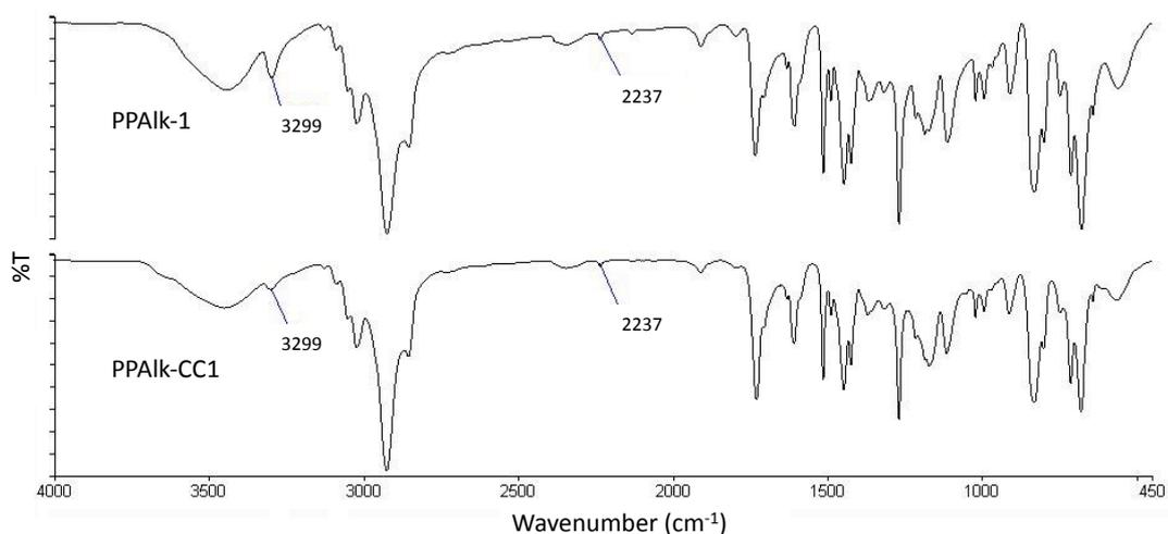
**Figure 4.3.7.2. – FT-IR spectra of the alkyne-containing precursor polymer PPAlk-1 and the product obtained from reaction of PPAlk-1 with VBAz in DMF at  $80\text{ }^{\circ}\text{C}$  for 24 hours, PPAlk-CC1.**
