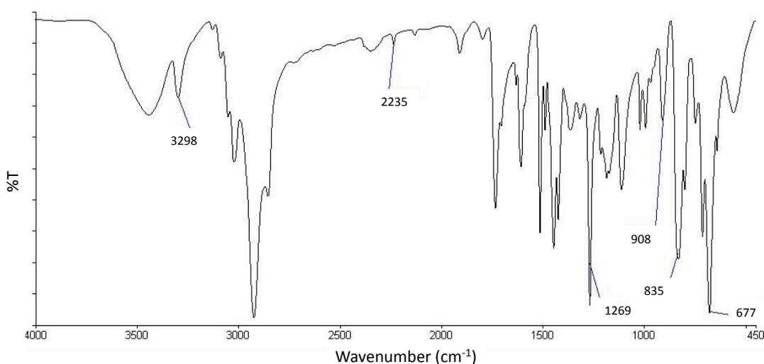
**Figure 4.3.5.3. – FT-IR spectrum for copolymer PPAlk-1 prepared using 25/70/5 (w/w/w) DVB/VBC/PMA in the feed.**
