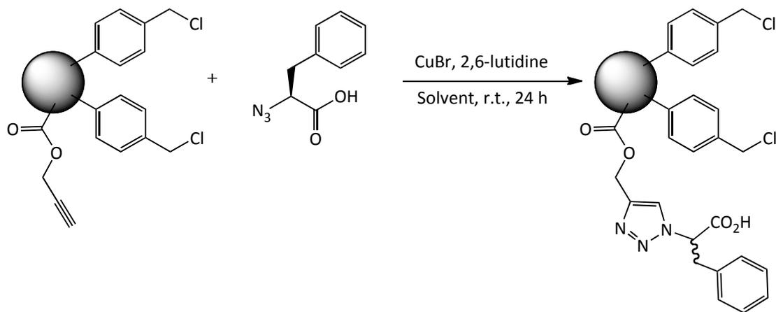
**Figure 4.3.7.5. – Reaction of  $\alpha$ -azido-*L*-phenylalanine with alkyne-containing polymer microspheres PPAlk-1 *via* click chemistry.**
