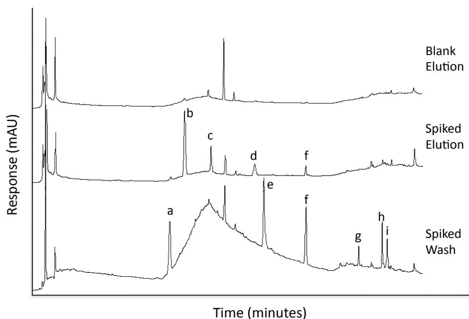
**Figure 2.3.7.3.1. – Chromatograms obtained from 1,000 mL spiked (2 µg/L) and blank samples of Ebro river water percolated through the HXL-PP-SCXc sorbent: (a) caffeine, (b) trimethoprim, (c) antipyrine, (d) propranolol, (e) salicylic acid, (f) carbamazepine, (g) clofibric acid, (h) diclofenac and (i) ibuprofen.**
