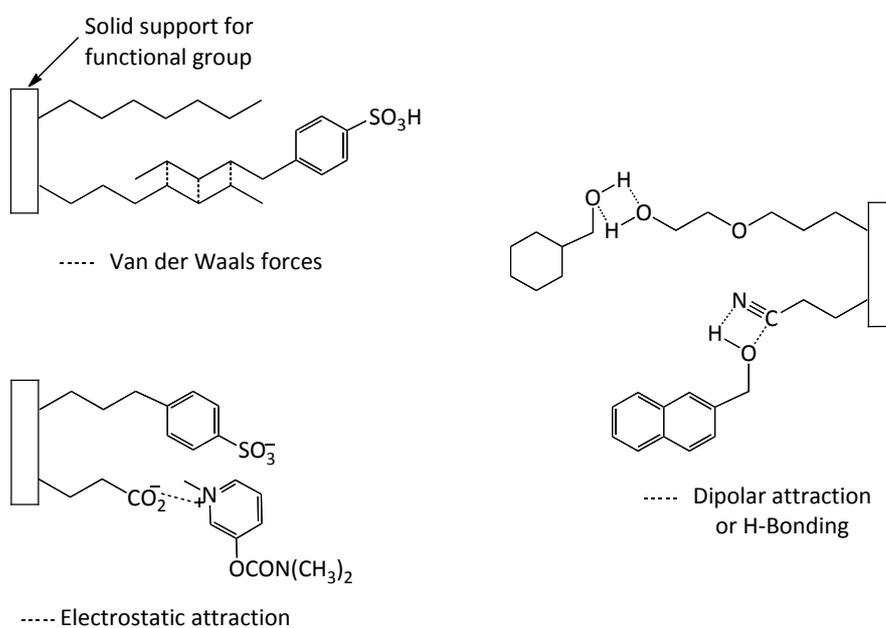
Figure 2.1.4.2. – Modes of bonding in SPE.<sup>36</sup>
