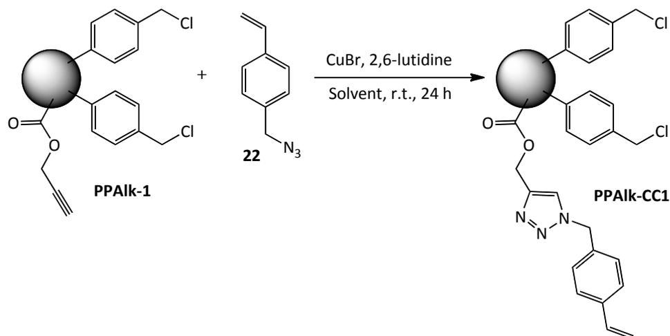
**Figure 4.3.7.1. - Click chemistry modification of alkyne-containing polymer microspheres PPAlk-1 with the azide VBAz.**
