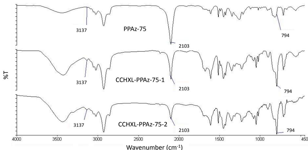
**Figure 4.3.10.2.2. – FT-IR spectra obtained for azide-containing precursor polymer (PPaz-75) and the corresponding hypercrosslinked click products CCHXL-PPaz-75-1 and CCHXL-PPaz-75-2.**
