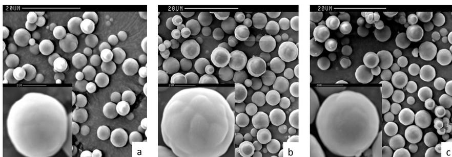
**Figure 4.3.9.3 – SEM images obtained for: (a) the precursor PP11, (b) the hypercrosslinked polymer HXL-PP11 and (c) the azide-modified hypercrosslinked polymer HXL-PP11-Az.**
