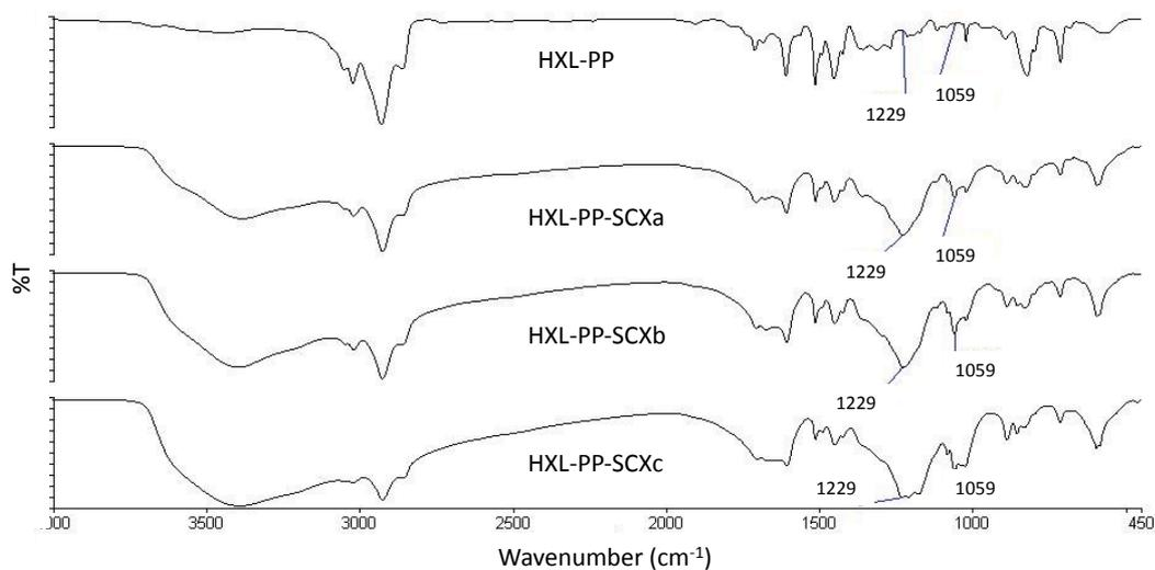
**Figure 2.3.6.2. – FT-IR spectra of a non-sulfonated hypercrosslinked polymer and three sulfonated derivatives.**
