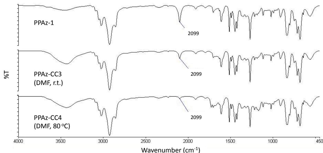
**Figure 4.3.3.3. – FT-IR spectra for an azide-containing polymer, PPAz-1, and the products of click reactions of PPAz-1 and propargyl alcohol carried out in DMF at different temperatures.**
