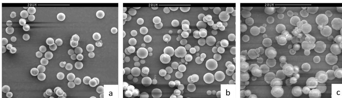
**Figure 2.3.6.1. – SEM micrographs obtained for the sulfonated hypercrosslinked polymers: (a) HXL-PP-SCXa, (b) HXL-PP-SCXb, (c) HXL-PP-SCXc.**
