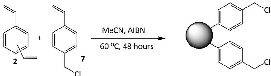
**Figure 2.3.1.1.1. – Synthesis of poly(DVB-co-VBC) microspheres.**
