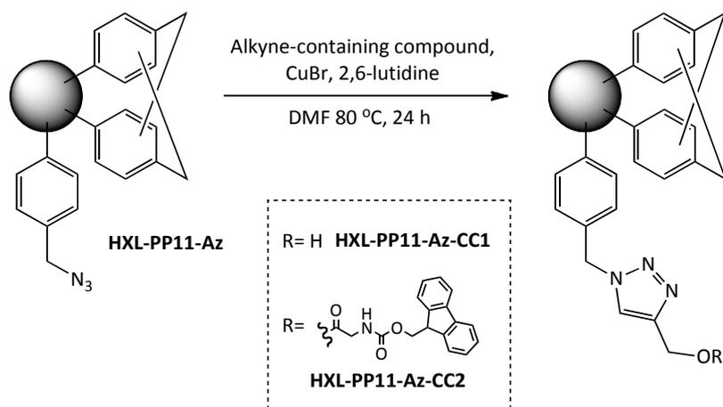
**Figure – 4.3.9.4. – Modification of the azide-containing hypercrosslinked polymer HXL-PP11-Az microspheres using propargyl alcohol and Fmoc-glycine propargyl ester to give the products HXL-PP11-Az-CC1 and HXL-PP11-Az-CC2, respectively.**
