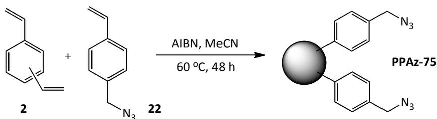
**Figure 4.3.10.1.1. – Synthesis by precipitation polymerisation of 25/75 (w/w) DVB/VBAz copolymer, PPAz-75.**
