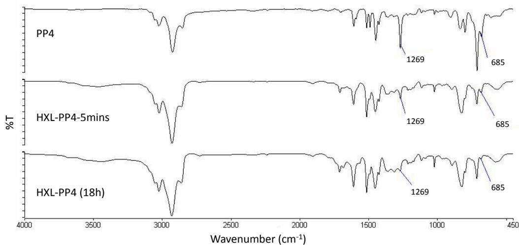
**Figure 3.3.3.2. – Comparison of FT-IR spectra for the hypercrosslinked polymers formed after 5 minutes and 18 hours of reaction with the non-hypercrosslinked precursor material.**
