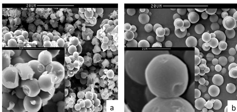
**Figure 4.3.7.3. – SEM micrographs obtained for (a) PPAlk-1 and (b) PPAlk-CC1.**
