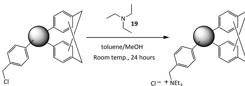
**Figure 3.3.1.1. – Amination of pendent chloromethyl groups on the hypercrosslinked polymer, using TEA as the amine.**
