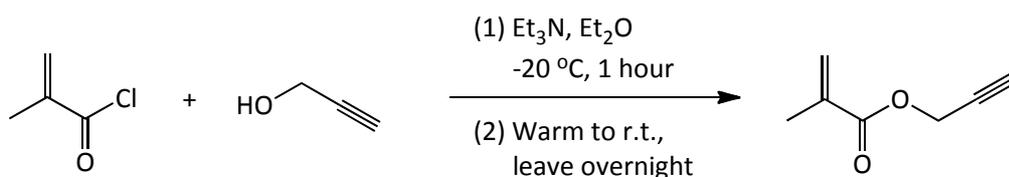
**Figure 4.3.5.1. - Reaction of methacryloyl chloride with propargyl alcohol to give the methacrylate ester propargyl methacrylate (PMA).**
