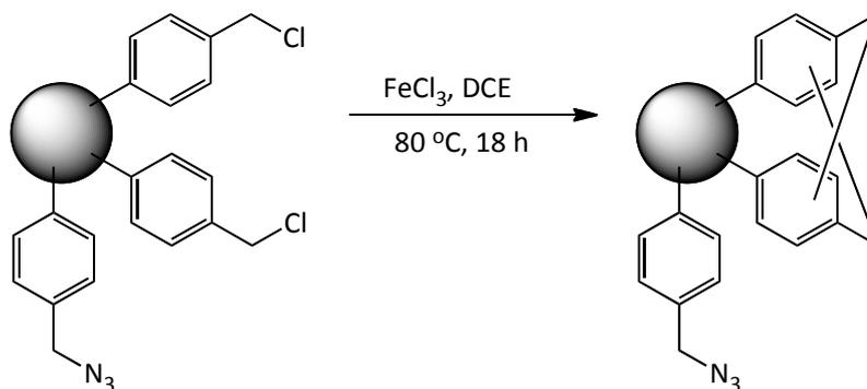
Figure 4.3.2.1. - Hypercrosslinking of the azide-containing polymer, PPAz-1.
