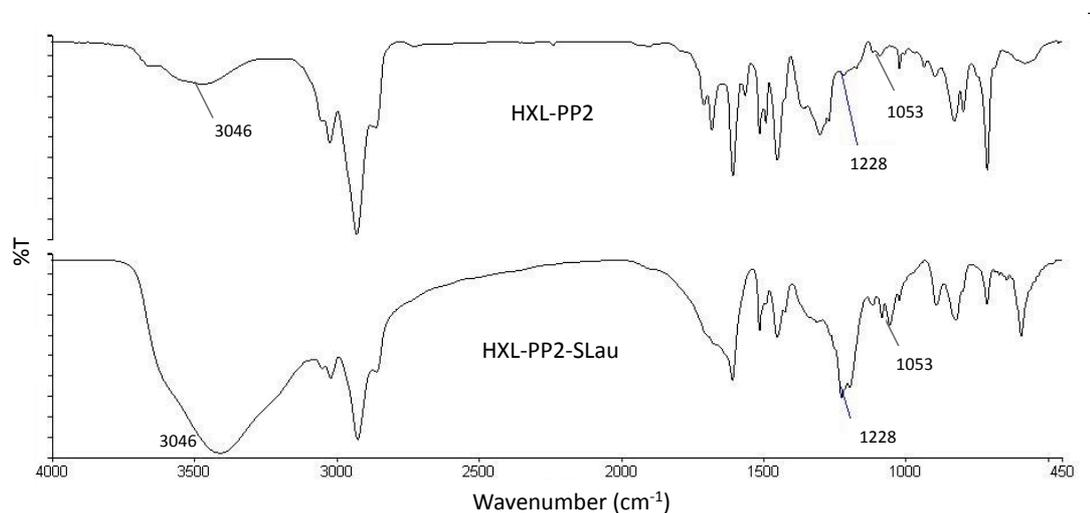
**Figure 2.3.3.2. – FT-IR spectra showing the hypercrosslinked polymer HXL-PP2 and the product of the reaction of the HXL-PP2 polymer with lauroyl sulfate, HXL-PP2-SLau.**
