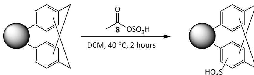
**Figure 2.3.2.1. – Sulfonation of hypercrosslinked particles using acetyl sulfate.**
