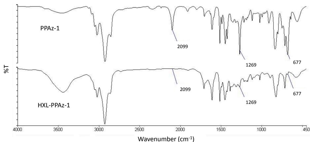
**Figure 4.3.2.2. - FT-IR spectra of the azide-containing polymer PPAz-1 and its hypercrosslinked derivative.**
