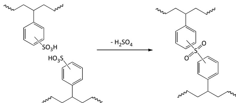
**Figure 2.1.3.1. - Formation of sulfone bridges.**
