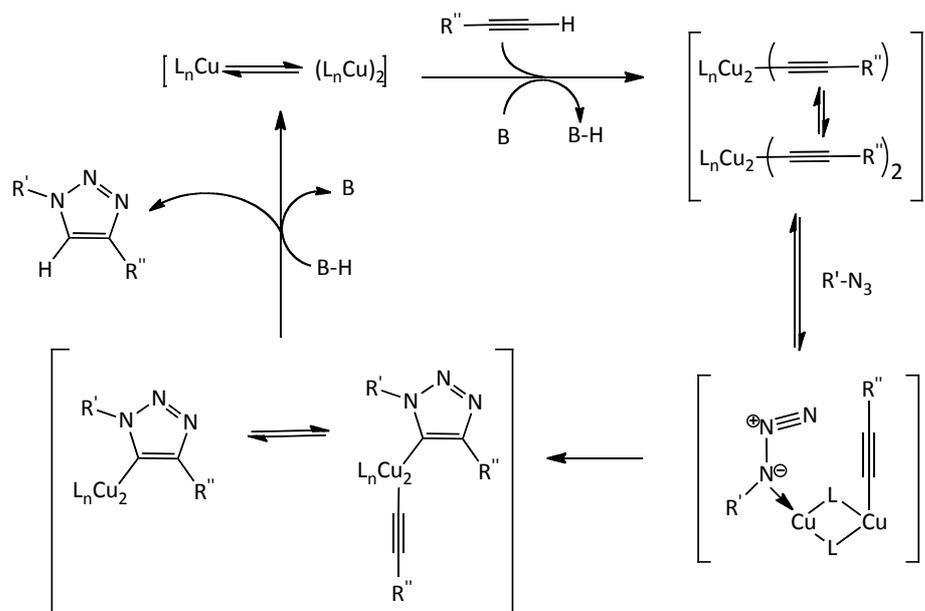
**Figure 4.1.3.1.2. – Mechanism proposed by Rodionov for copper(I) catalysed azide-alkyne cycloaddition.<sup>14</sup>**
