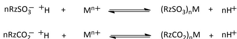
Figure 2.1.1.1. – Exchange of protons on cation-exchange resins (Rz = resin).
