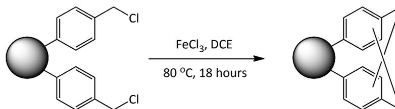
**Figure 2.3.1.2.1 – Hypercrosslinking reaction using FeCl<sub>3</sub> as the Friedel-Crafts catalyst.**
