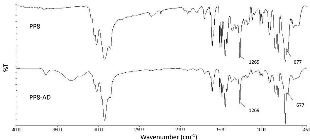
**Figure 3.3.5.1.2. – FT-IR spectra for the poly(DVB-co-VBC) precursor, PP8, and the corresponding aminated material, PP8-AD.**
