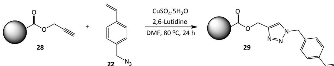
**Figure 4.1.6.2.4. - Click reaction of alkyne-containing polymer microspheres and VBAz (22).**
