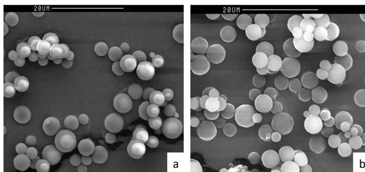
**Figure 3.3.6.2. – SEM micrographs for the HXL-PP-SAX materials; (a) HXL-PP-SAXa, (b) HXL-PP-SAXb.**
