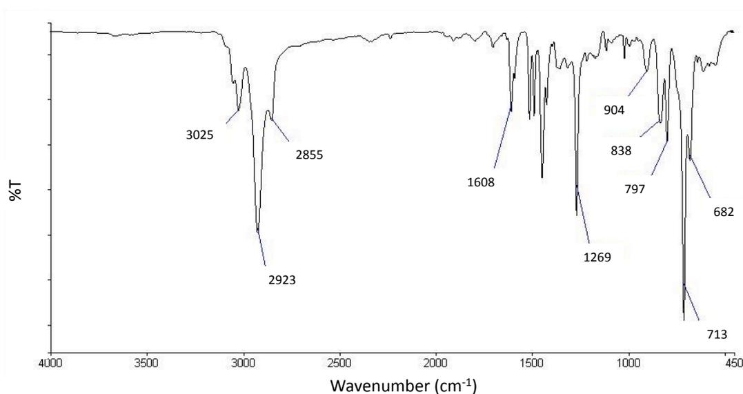
**Figure 2.3.1.1.2 – FT-IR spectrum for DVB/VBC copolymer PP1.**
