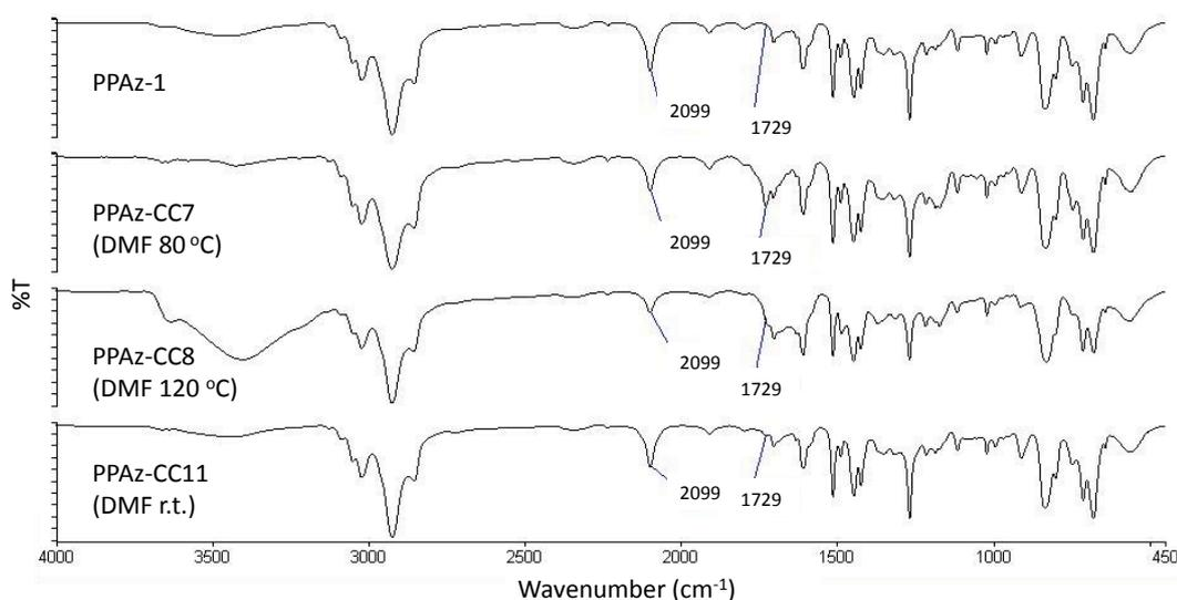
**Figure 4.3.3.6. – FT-IR spectra obtained for the products collected after reaction of PPAz-1 with Fmoc-glycine propargyl ester in DMF for 24 hours at different temperatures.**
