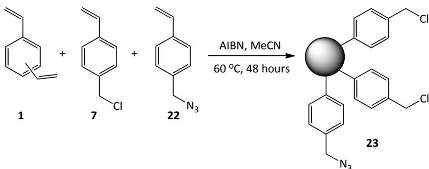
**Figure 4.1.6.1.2. – Precipitation polymerisation incorporating ‘clickable’ monomer VBAz.**
