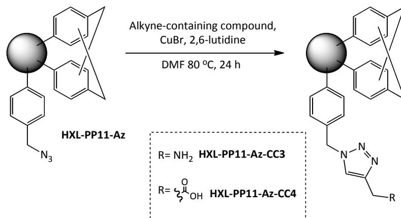
**Figure 4.3.9.7. - Modification of the azide-containing hypercrosslinked polymer HXL-PP11-Az microspheres using propargyl amine and 4-pentynoic acid to give the products HXL-PP11-Az-CC3 and HXL-PP11-Az-CC4, respectively.**
