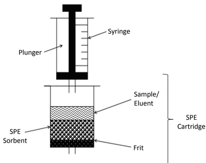
Figure 2.1.4.1. – SPE process using positive pressure.<sup>36</sup>
