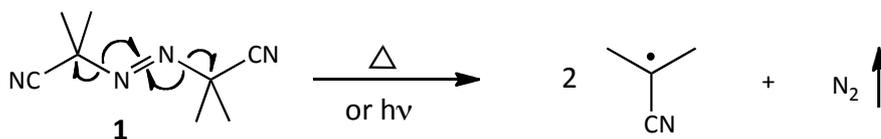
**Figure 1.1.1. - Thermal and photochemical breakdown of AIBN.**
