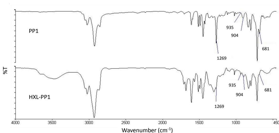
**Figure 2.3.1.2.2. – FT-IR spectra of precursor, PP1, and its hypercrosslinked derivative HXL-PP1.**
