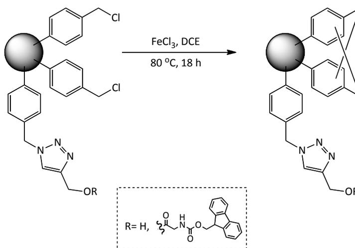
Figure 4.3.4.1. – Hypercrosslinking of the polymer microspheres modified using click chemistry.
