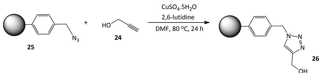
**Figure 4.1.6.2.2. - Click reaction of propargyl alcohol and azide-containing polymer microspheres.**
