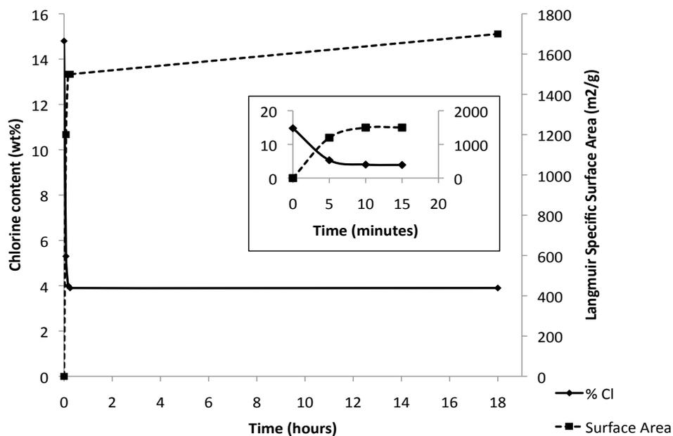
**Figure 3.3.3.1. - Time study graph showing a decrease in chlorine content and simultaneous increase in Langmuir specific surface area with respect to time.**
