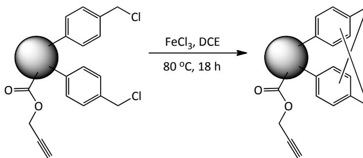
**Figure 4.3.6.1. - Hypercrosslinking of the alkyne-containing polymer microspheres PPAlk-2 prior to functionalisation.**
