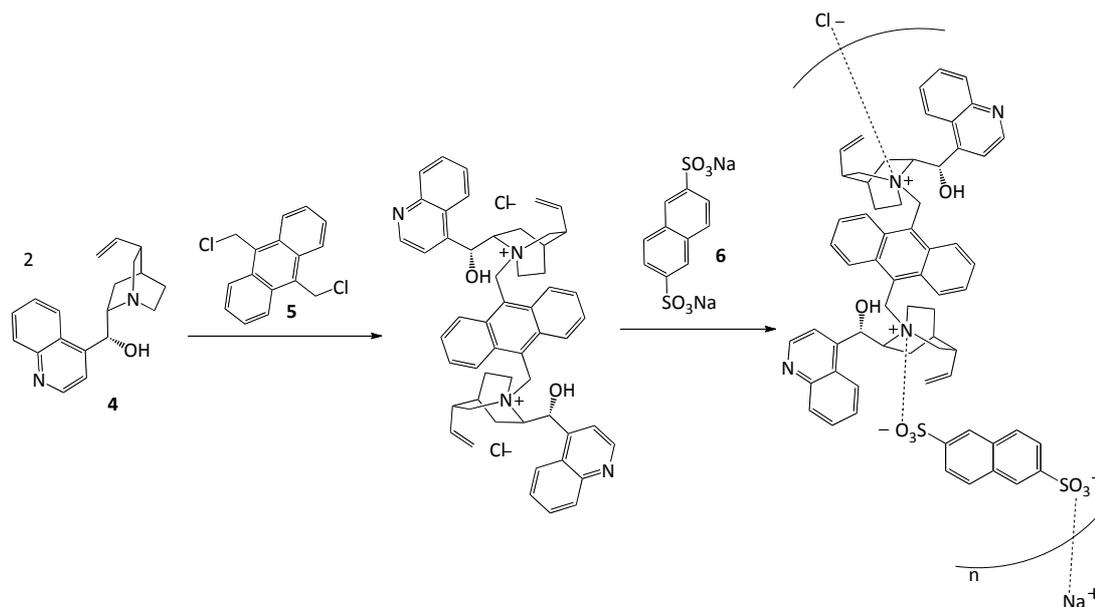
Figure 2.1.2.2. – Synthesis of main-chain polymer chiral catalyst.<sup>17</sup>
