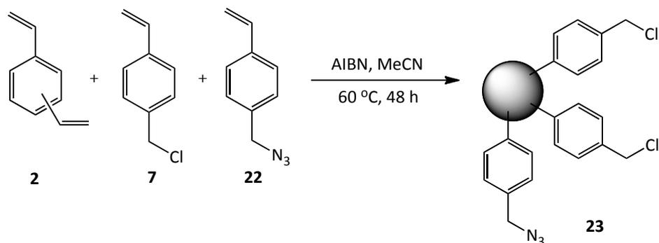
**Figure 4.3.1.2. – Synthesis of poly(DVB-co-VBC-co-VBAz) microspheres using precipitation polymerisation conditions.**
