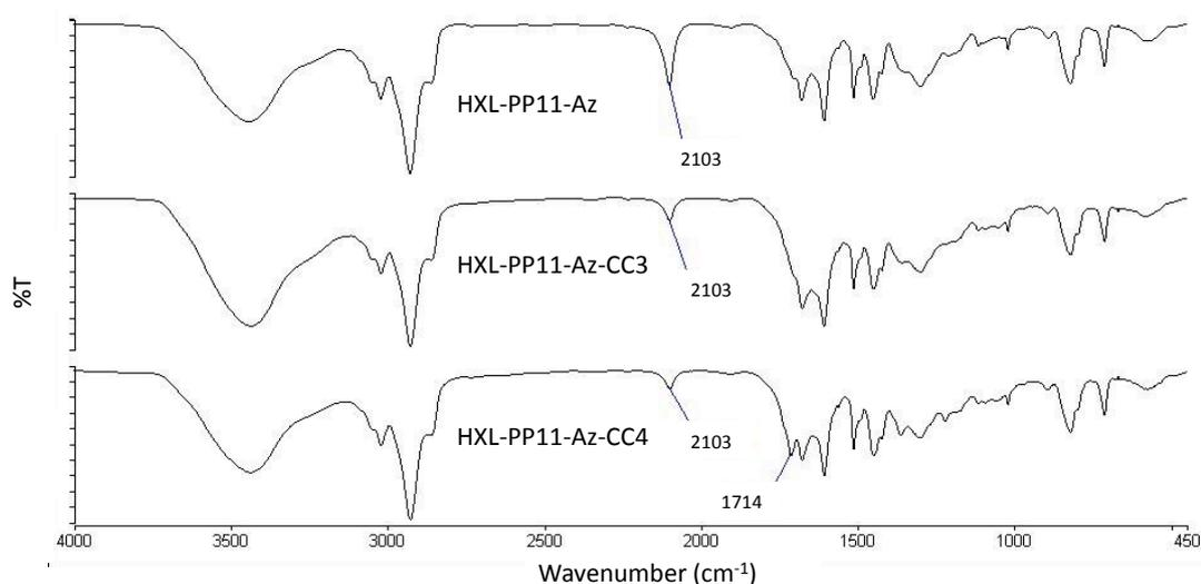
**Figure 4.3.9.8. – FT-IR spectra obtained for the azide modified hypercrosslinked polymer HXL-PP11-Az and the subsequent products derived from its click reactions with propargyl amine and 4-pentynoic acid (HXL-PP11-Az-CC3 and HXL-PP11-Az-CC4, respectively).**
