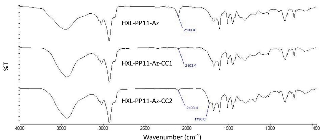
**Figure 4.3.9.5. – FT-IR spectra for the azide-modified hypercrosslinked polymer HXL-PP11-Az and the subsequent products derived from its click reactions with propargyl alcohol and Fmoc-glycine propargyl ester (HXL-PP11-Az-CC1 and HXL-PP11-Az-CC2, respectively).**
