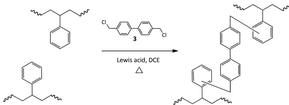
**Figure 1.4.1.** – Use of external crosslinking agent 1,4-*bis*-chloromethyldiphenyl (3).
