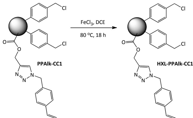
Figure 4.3.8.1. - Hypercrosslinking reaction of the click chemistry modified polymer PPAlk-CC1.
