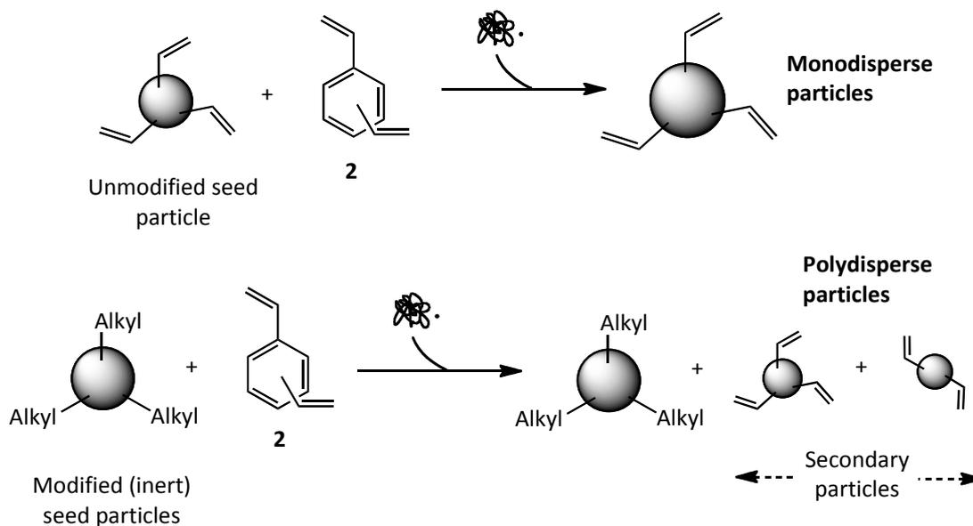
**Figure 1.3.3. - Particle growth mechanisms.<sup>8</sup>**
