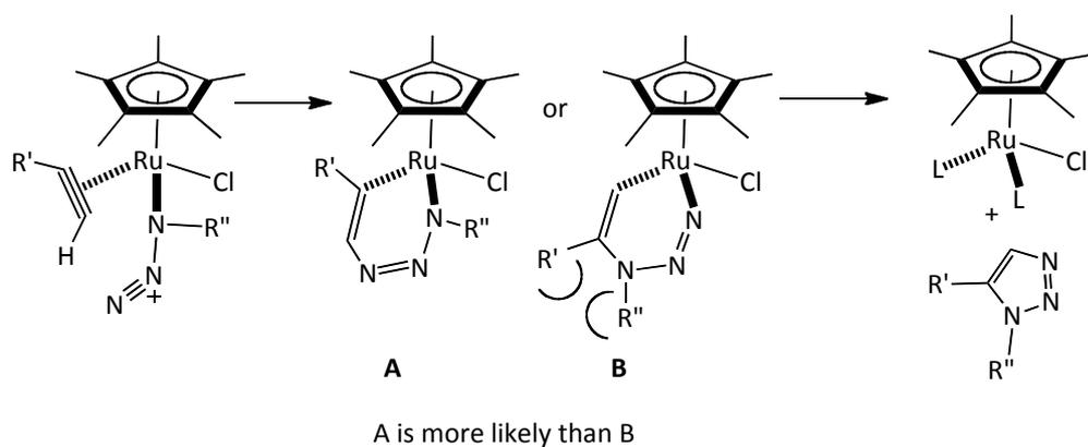
**Figure 4.1.3.4.2. – Proposed reaction intermediates for the ruthenium-catalysed reaction of an azide and a terminal alkyne.<sup>22</sup>**
