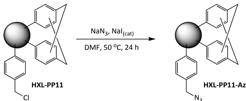
**Figure 4.3.9.1. – Synthesis of clickable polymer microspheres with high specific surface area via the post-polymerisation modification of a hypercrosslinked polymer (PP11).**
