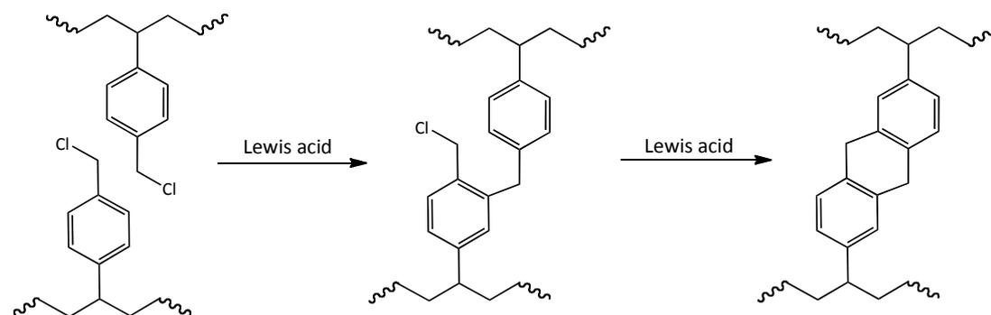
**Figure 1.4.2.** – Hypercrosslinking reaction of poly(DVB-*co*-VBC) via an internal electrophile.<sup>32</sup>
