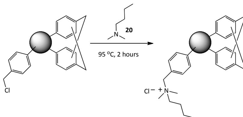
**Figure 3.3.2.1. - Amination of pendent chloromethyl groups on the hypercrosslinked polymer using DMBA.**
