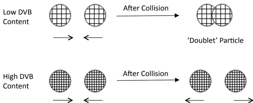
Figure 1.3.4. - Collision induced formation of multiplet particles.<sup>7</sup>
