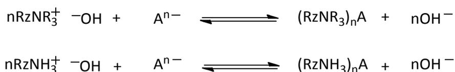
**Figure 3.1.1.1. - Exchange of hydroxyl anion on anion-exchange resin (Rz=Resin).**
