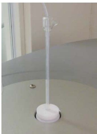
Figure 3.2 – Top of spectrometer showing glass Dewar and capillary
