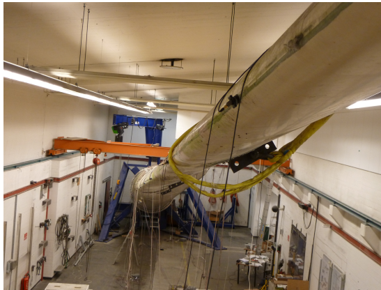
Figure 4.7: Experiment set up of the SSP34 wind turbine blade. a) Experiment scheme. b) Experiment set up. c) Electromechanical actuator.
