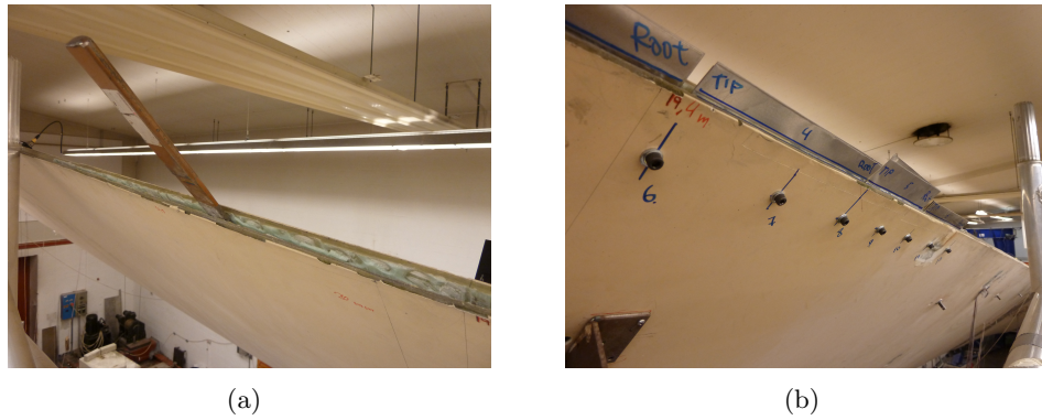
Figure 4.8: Damage introduced in SSP34 wind turbine blade. a) Damage introduced by chisel in the trailing edge. b) Damage bolted to control the damage size and any additional anomalies introduced by the impact to generate the damage
