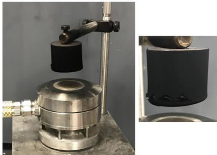
Figure 3.6: 33 mm diameter porous-plug burner with a 38 mm diameter cylindrical stabilisation plate.
