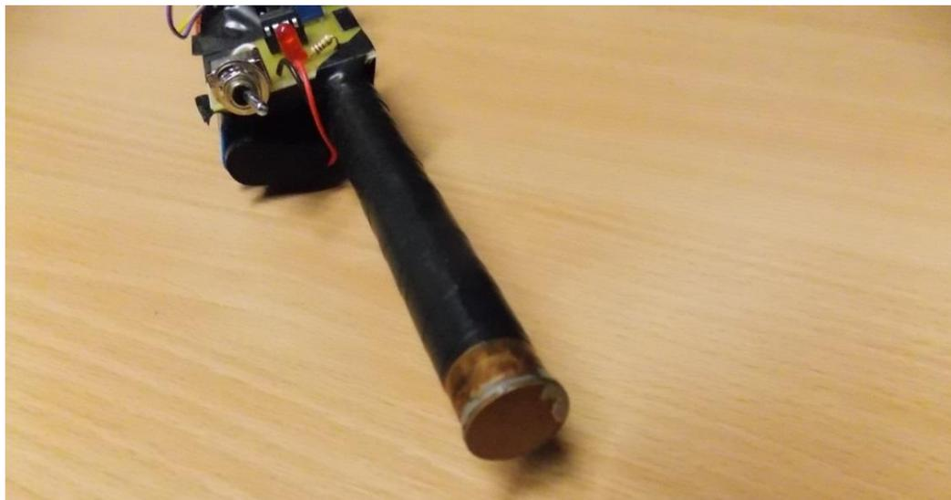
**Figure 7.16. Sealed end of pipe to allow samples to be held while IR sensor transmits voltage signal.**
