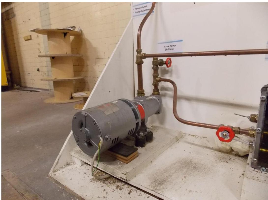
**Figure 6.4. Mono CMM263 Progressive Cavity Pump [104].**
