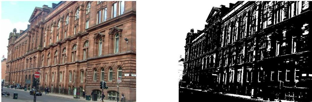
**Figure 6.21. Example of image processing where an image of the University of Strathclyde is converted to a binary image.**
