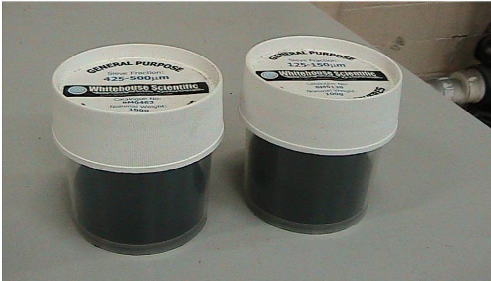
**Figure 6.44. Basalt spherical particles used for size testing and other experiments.**
