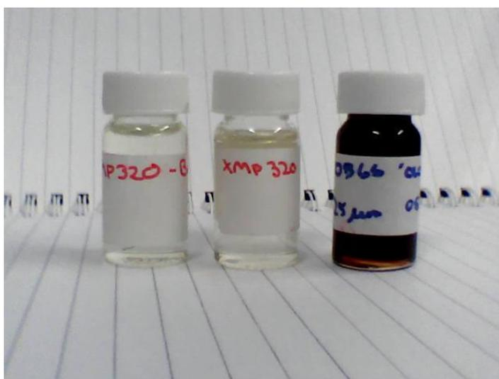
**Figure 7.1:** *Left* - New sample, *Middle* - Used test rig sample, *Right* - Used gearbox sample.
