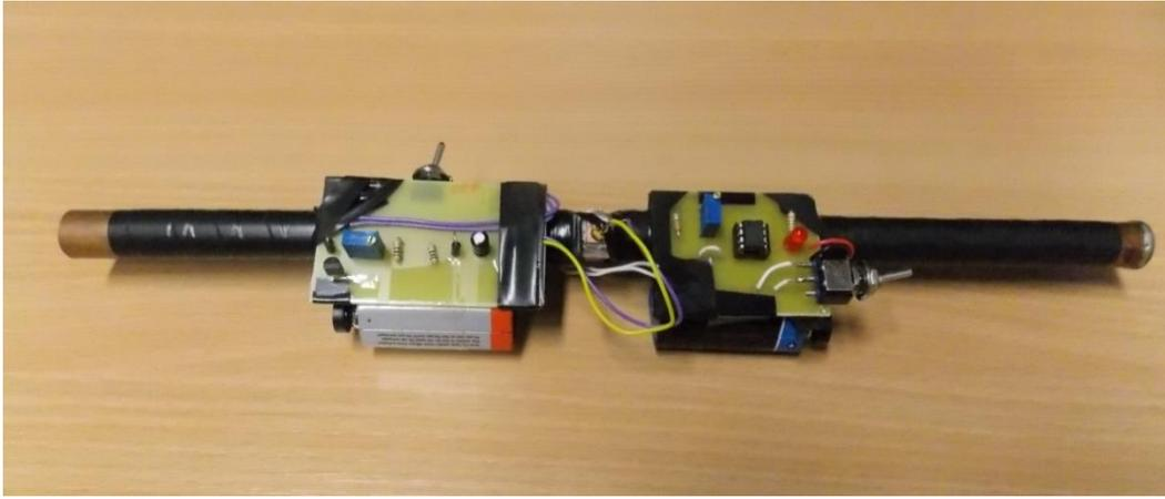
**Figure 7.15. Circuit mounted on copper pipe.**
