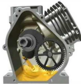
**Figure 4.12. Meshing gears with splash lubrication provided by reservoir at base.**
