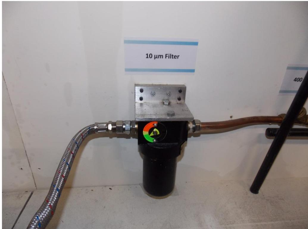
**Figure 6.8. 10 mm filter is last component before lubricant re-enters reservoir.**
