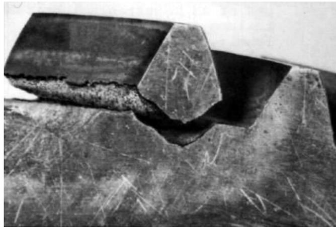
**Figure 3.1. Cracked tooth completely detached from gear [38].**
