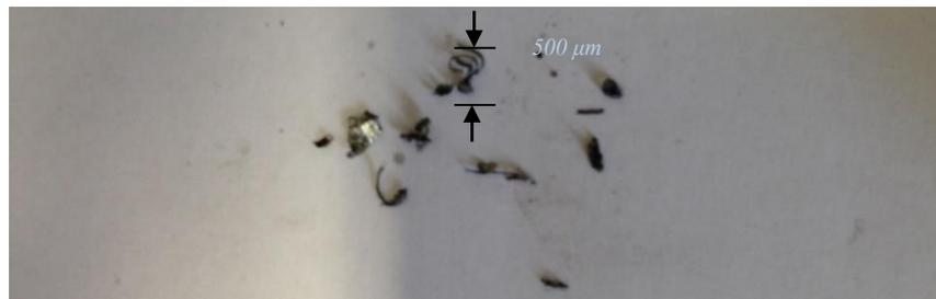
**Figure 6.46. Sample of wear particles used for testing morphology.**
