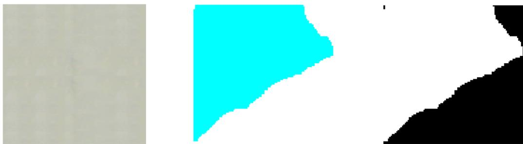
**Figure 8.12. Image with no particles present with application of Otsu's finding difference in greyscale and applies boundary conditions.**
