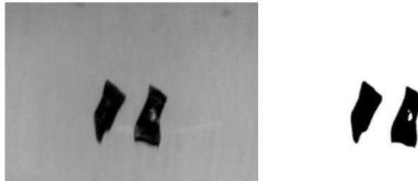
**Figure 6.37. 2x 750  $\mu\text{m}$  particles. *Left* – Image from APS, *Right* – Conversion of image using Otsu's method into bi-modal.**
