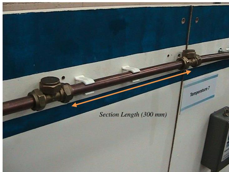
**Figure 6.16. Rig with 300 mm copper pipe sections visible.**
