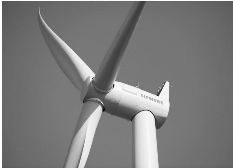
**Figure 2.3. Siemens 3MW 3 bladed HAWT wind turbine [19].**
