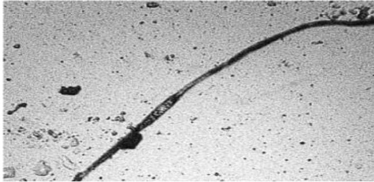
**Figure 3.10. Cutting wear particle 500  $\mu\text{m}$  in length [51].**
