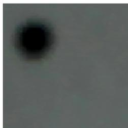
*Upper histogram represents image to the left - a particle in lubricant. Darker lubricant is an effect of having large particles skewing average greyscale value.*
