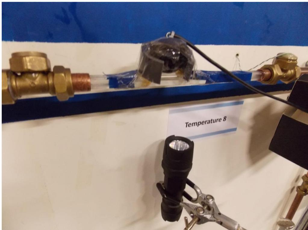
**Figure 6.20. Light source position below APS sensor (N.B. box shield is placed over assembly to reduce incident of ambient light).**
